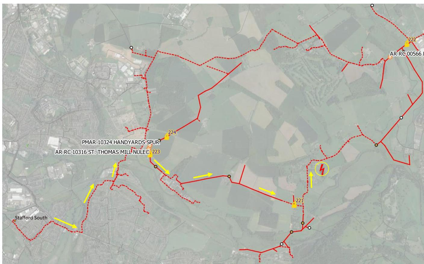
**Figure 5-3: Geographical view of part of the Tilcon Industrial Estate feeder from Stafford South**
