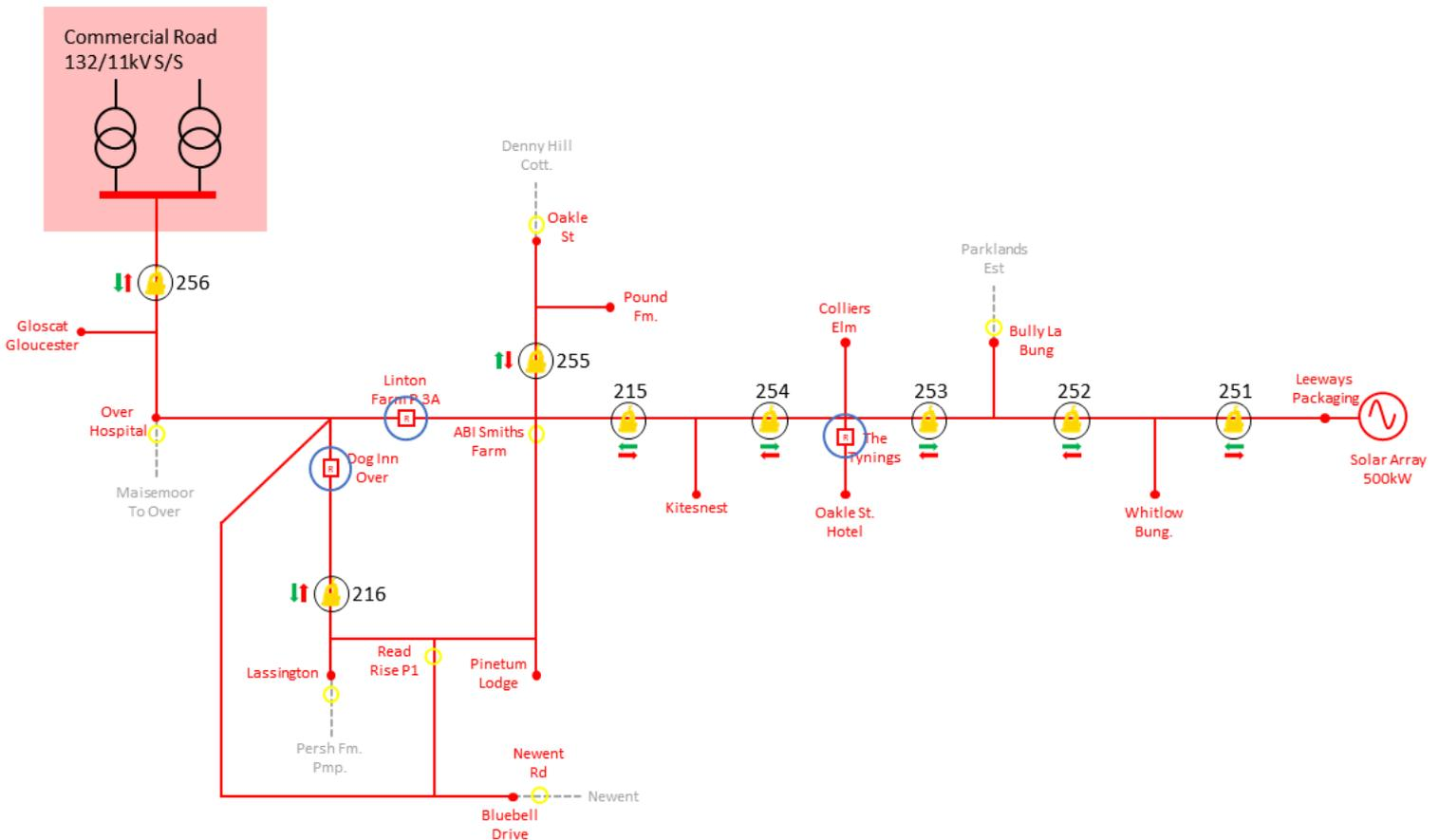
**Figure 5-1: The 11kV Distribution Network**
