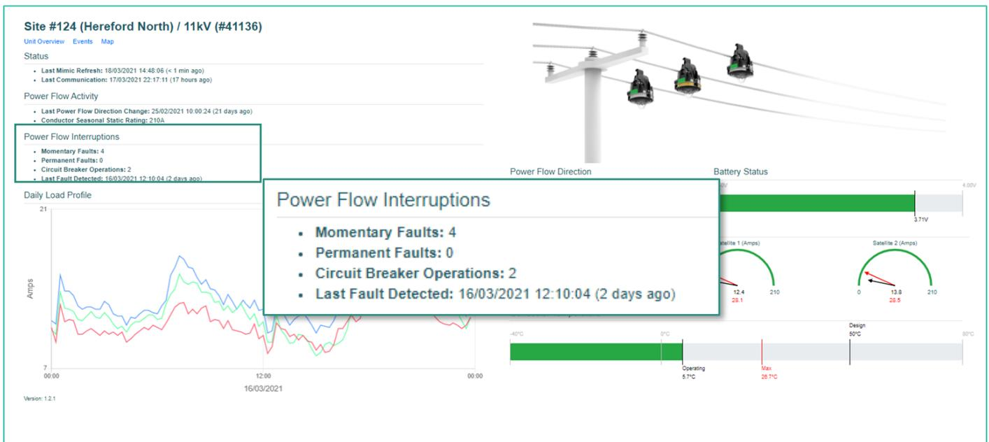
Figure 5-2: Smart Navigator 2.0 Dashboard – Power Flow Interruptions
