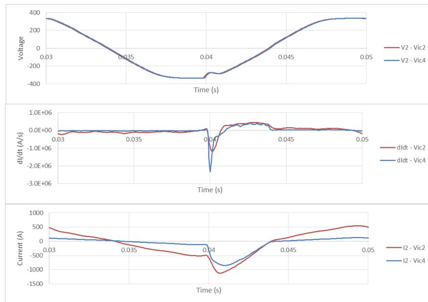
While the voltage waveforms look similar, the difference in the  $dl/dt$  waveforms is striking, with a significantly sharper and deeper dip recorded by Vic4 at the onset of the pecking fault. The portions of the current waveforms during the faults show a different shape reflecting the difference in the  $dl/dt$  signals. The larger background current in the waveform from Vic2 (bottom panel) is to be expected due to the fact that this trace represents the sum of the currents on all the feeders.
