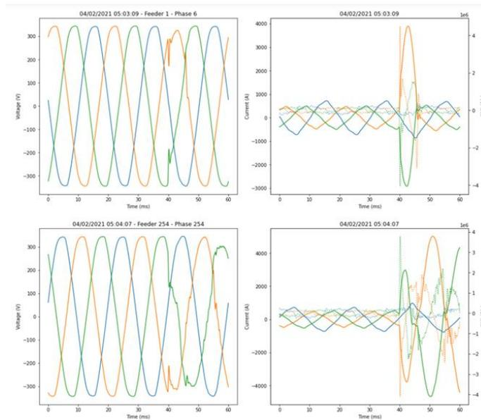
Only 4 pecking events were detected for this site, with an estimated distance of 120m +/- 14m. There is no feedback from the local team regarding whether this has been addressed and, if so, the distance of the fault.
