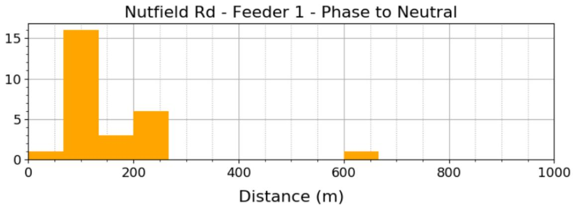
Further investigations are needed to determine if the peak at 100 m is originating from a different fault located around the indicated distance, or is caused by events originating actually at the location of the fault (40 m) that the analysis algorithm failed to characterise properly.
