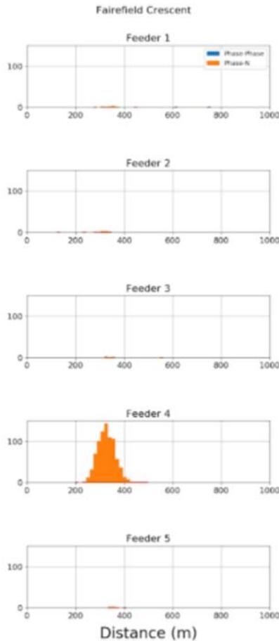
The histogram shows the likely distance to be 325m within +/-5m, with the uncertainty calculated as the error on the mean for a normal distribution.
