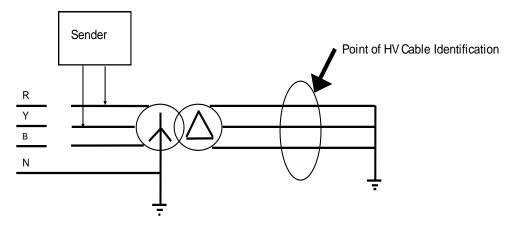
If it is not possible to make direct connection to the cable a signal may be injected through a distribution transformer.
