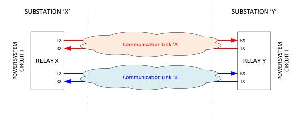
Notes: No single failure (e.g. D.C. power supply fuse, motherboard, multiplexer card, radio antenna, optical fibre, **Communication Bearer** etc.) should result in the concurrent failure of both **Communication Links**.
