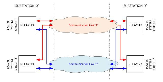
Notes: No single failure (e.g. D.C. power supply fuse, motherboard, multiplexer card, radio antenna, optical fibre, **Communication Bearer** etc.) should result in the concurrent failure of both **Communication Links**.
