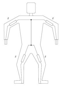
If Z is the internal impedance of an arm or a leg, then the hand to hand internal impedance is 2Z, as is the one hand to one foot internal impedance.
