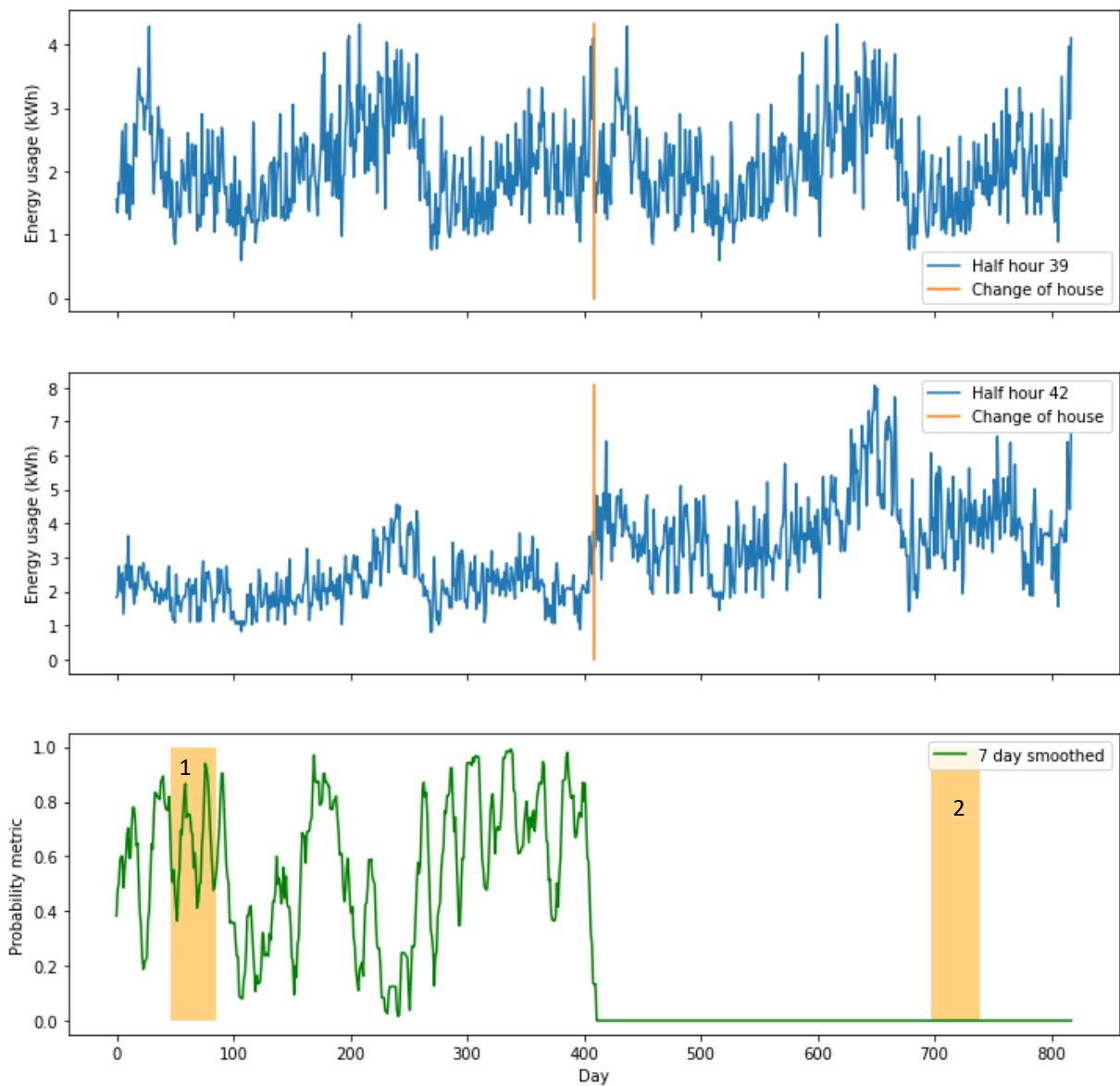
Figure 56: Change detection for increased night time usage (poor mental health).
