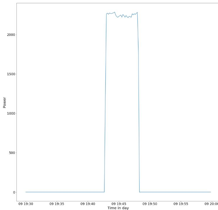
Figure 3: A randomly selected usage from the power drawn by the kettle from the UKEDC House 1 dataset.
