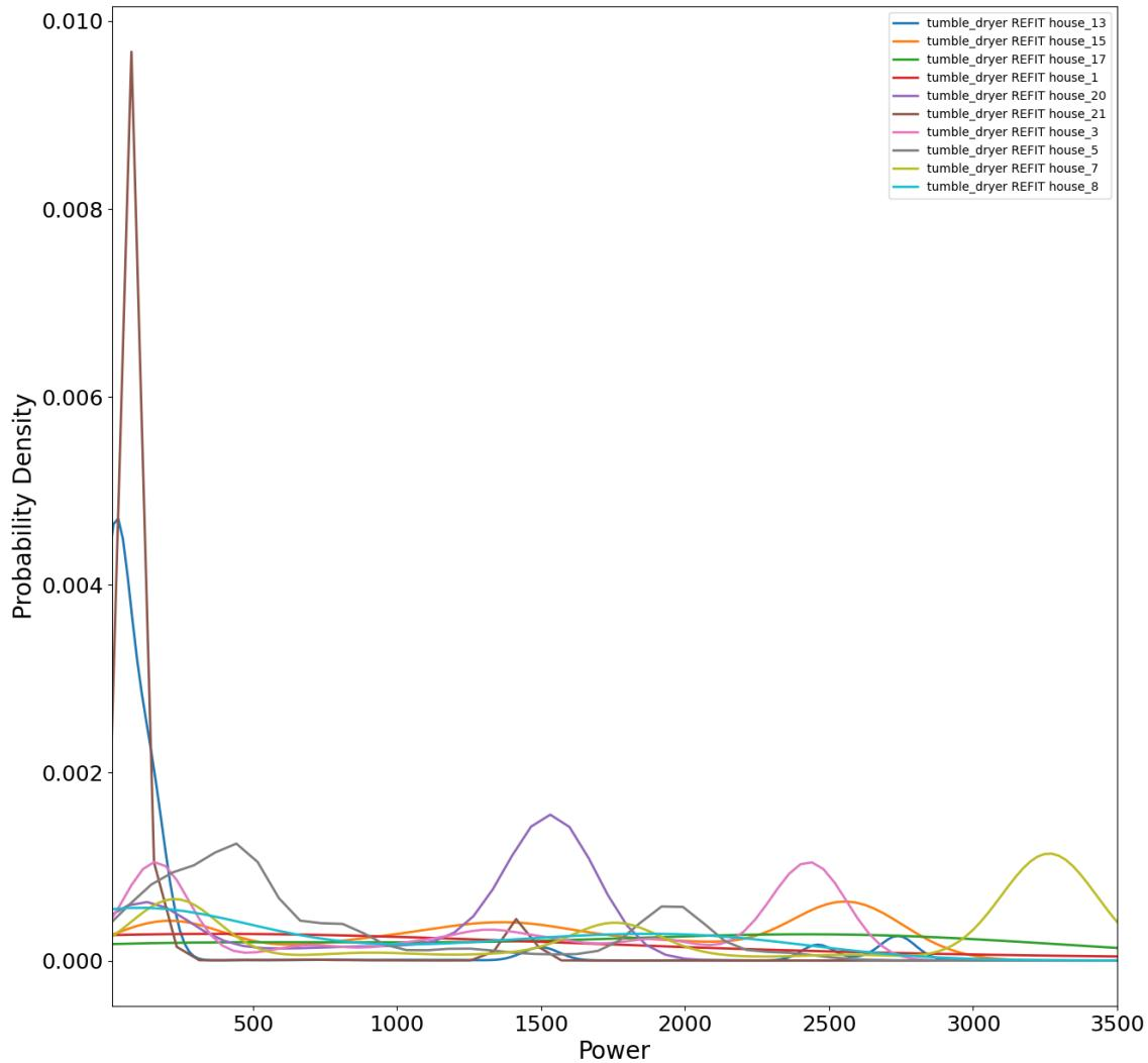
Figure 68: Gaussian kernel-density estimates of the power drawn by each appliance within the tumble dryer category.
