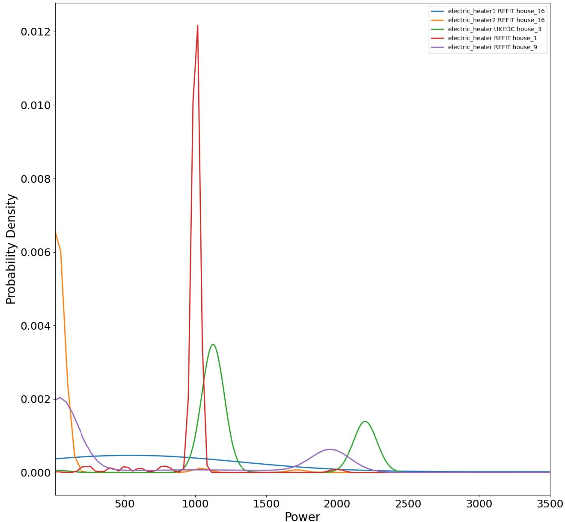
Figure 70: Gaussian kernel-density estimates of the power drawn by each appliance within the electric heater category.
