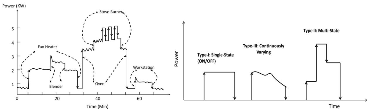
Figure 1: Plots showing the different types of power draw an appliance might have during a usage (David Murray et al., 2015).
