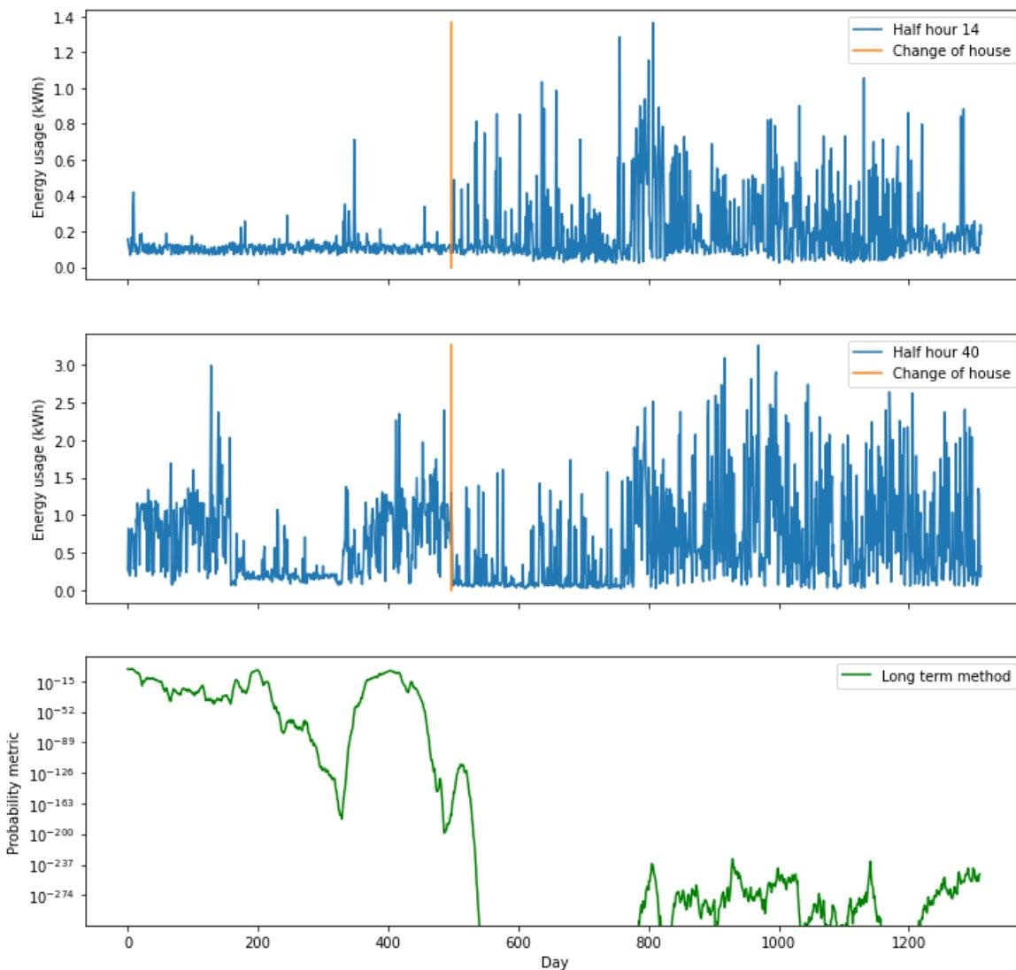
Figure 52: Example long term method output for two houses, with two half hours of underlying data also plotted.
