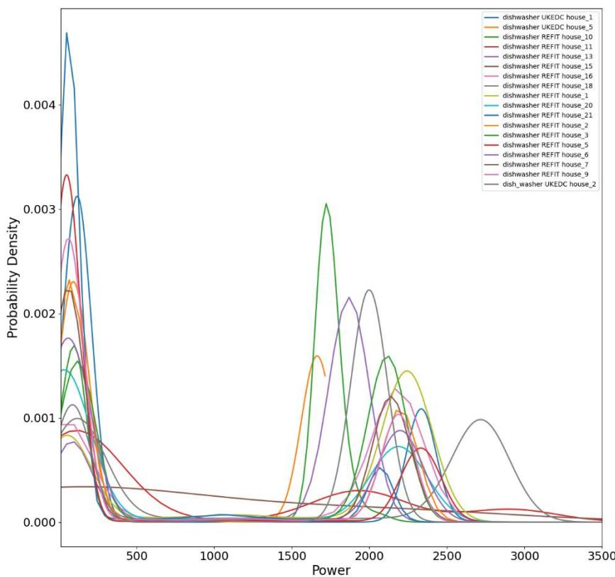
Figure 4: Gaussian kernel-density estimates of the power drawn by each appliance within the dishwasher category.
