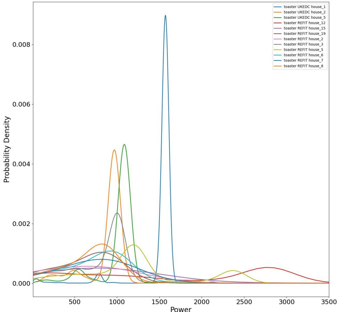
Figure 65: Gaussian kernel-density estimates of the power drawn by each appliance within the toaster category.
