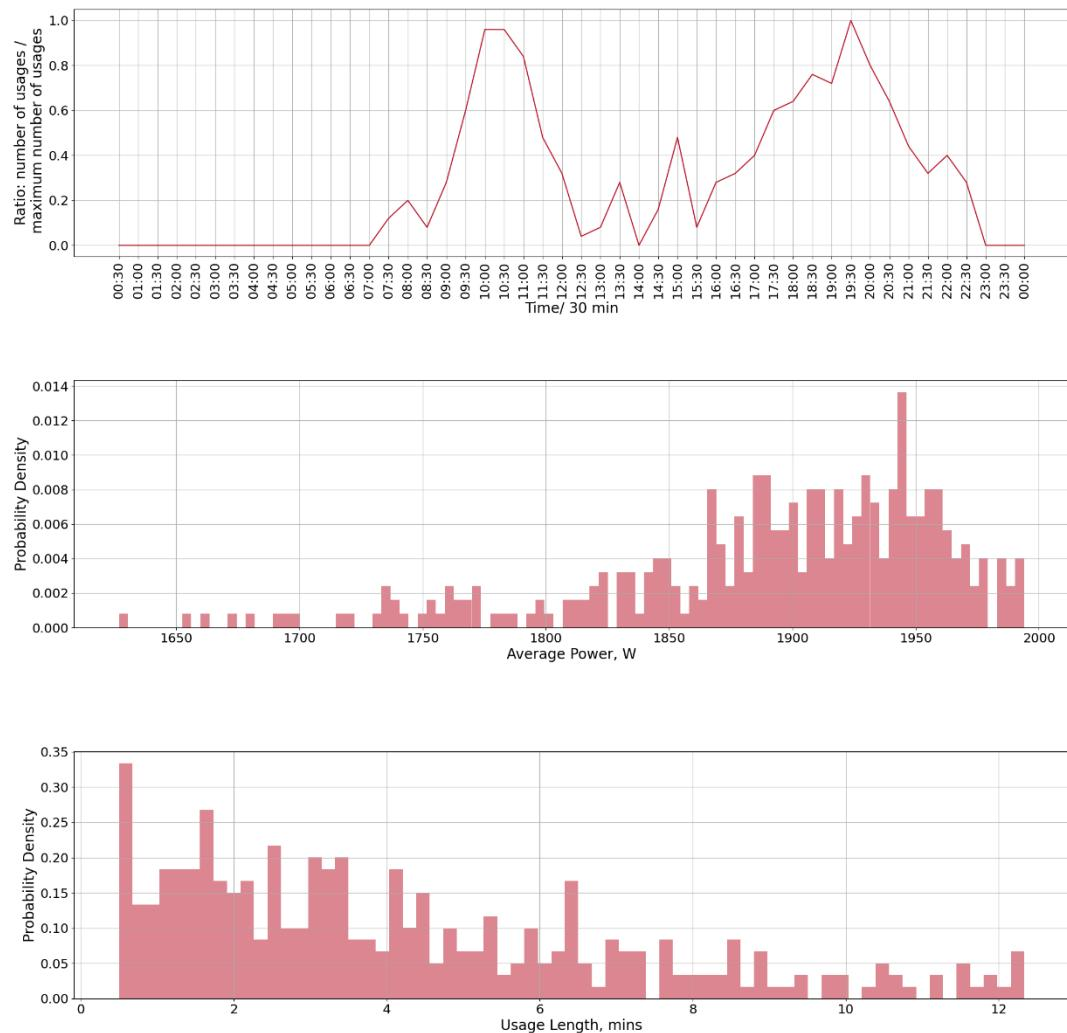
Figure 75: Usage statistics extracted for the vacuum across all datasets.
