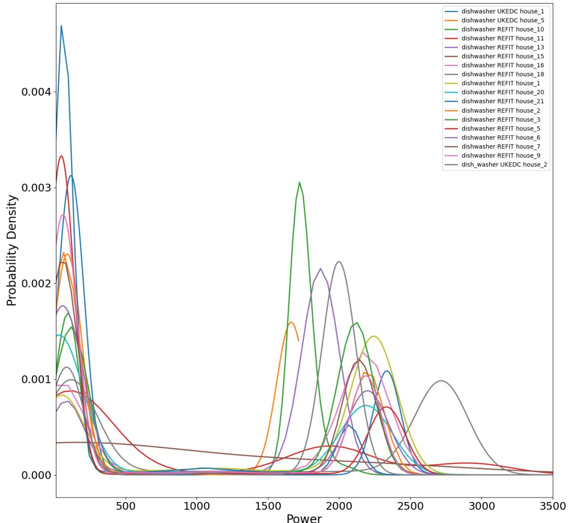
Figure 66: Gaussian kernel-density estimates of the power drawn by each appliance within the dishwasher category.
