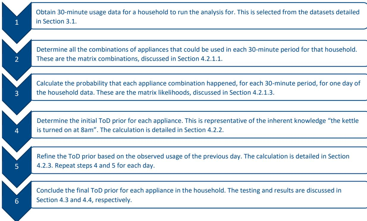
Figure 7: Overview of the appliance disaggregation and prediction method used.
