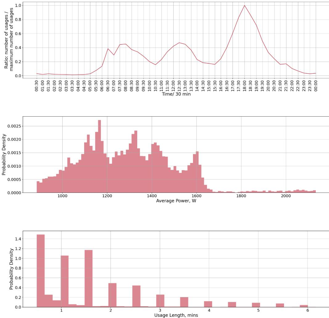
Figure 73: Usage statistics extracted for the microwave across all datasets.
