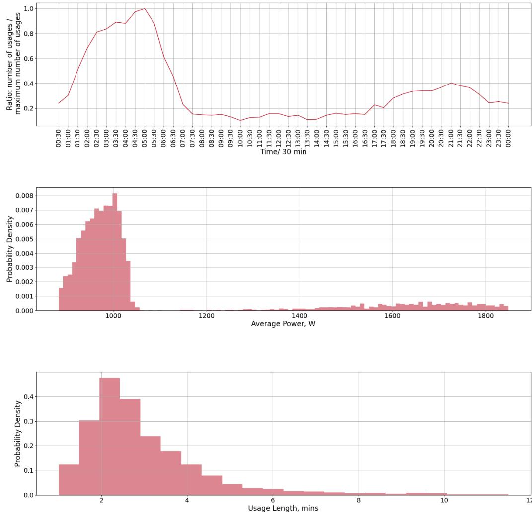
Figure 76: Usage statistics extracted for the electric heater across all datasets.
