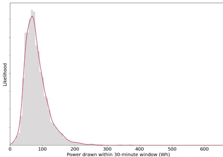
Figure 10: Distribution of power drawn by the kettle in a 30-minute window.
