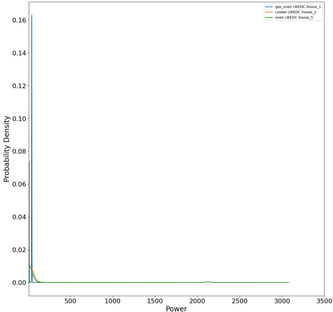
Figure 69: Gaussian kernel-density estimates of the power drawn by each appliance within the oven category.
