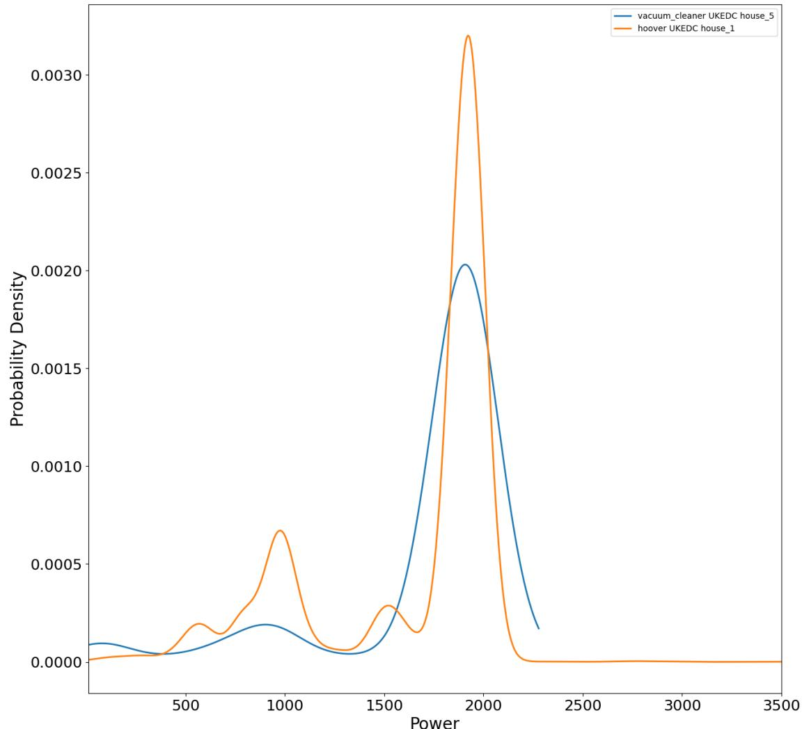
Figure 67: Gaussian kernel-density estimates of the power drawn by each appliance within the vacuum category.
