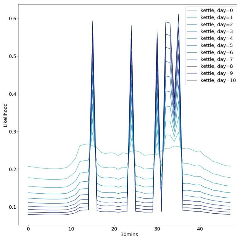
Figure 19: Change in the ToD prior for the kettle when the same day is run through the analysis ten times (day zero is the initial ToD prior and day ten is the ToD prior learnt after ten days of household usage). The kettle was turned on in 30-minute windows 15, 24, 30, 32 and 33.
