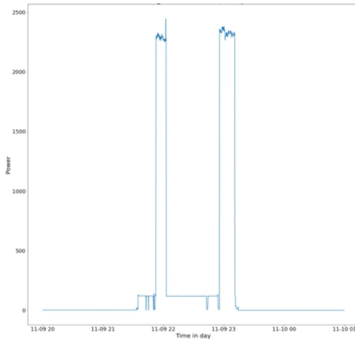
Figure 5: A randomly selected usage from the power drawn by the dishwasher from the UKEDC House 1 dataset. The time axis is displayed as the date and then the hour, for example, 11:09 20 represents 11<sup>th</sup> September at 8pm.
