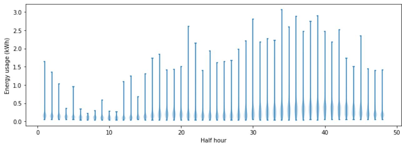
Figure 45: Violin plot showing distributions of half hourly usage for a specific house.
