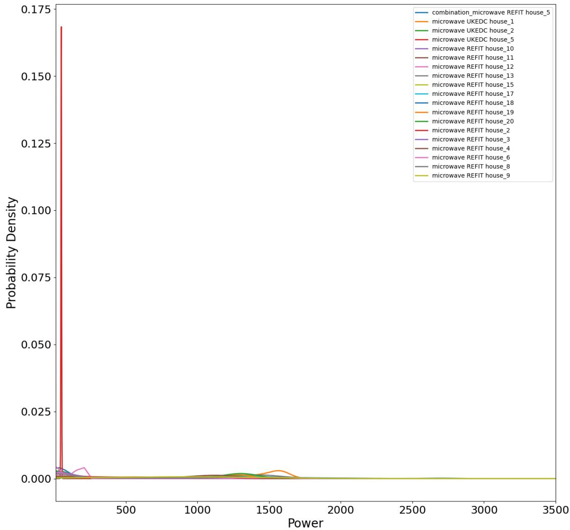
Figure 64: Gaussian kernel-density estimates of the power drawn by each appliance within the microwave category.
