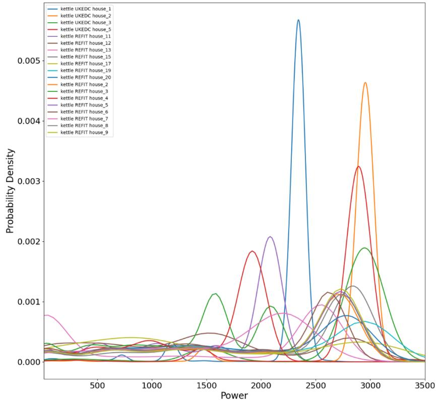
Figure 2: Gaussian kernel-density estimates of the power drawn by each appliance within the kettle category.
