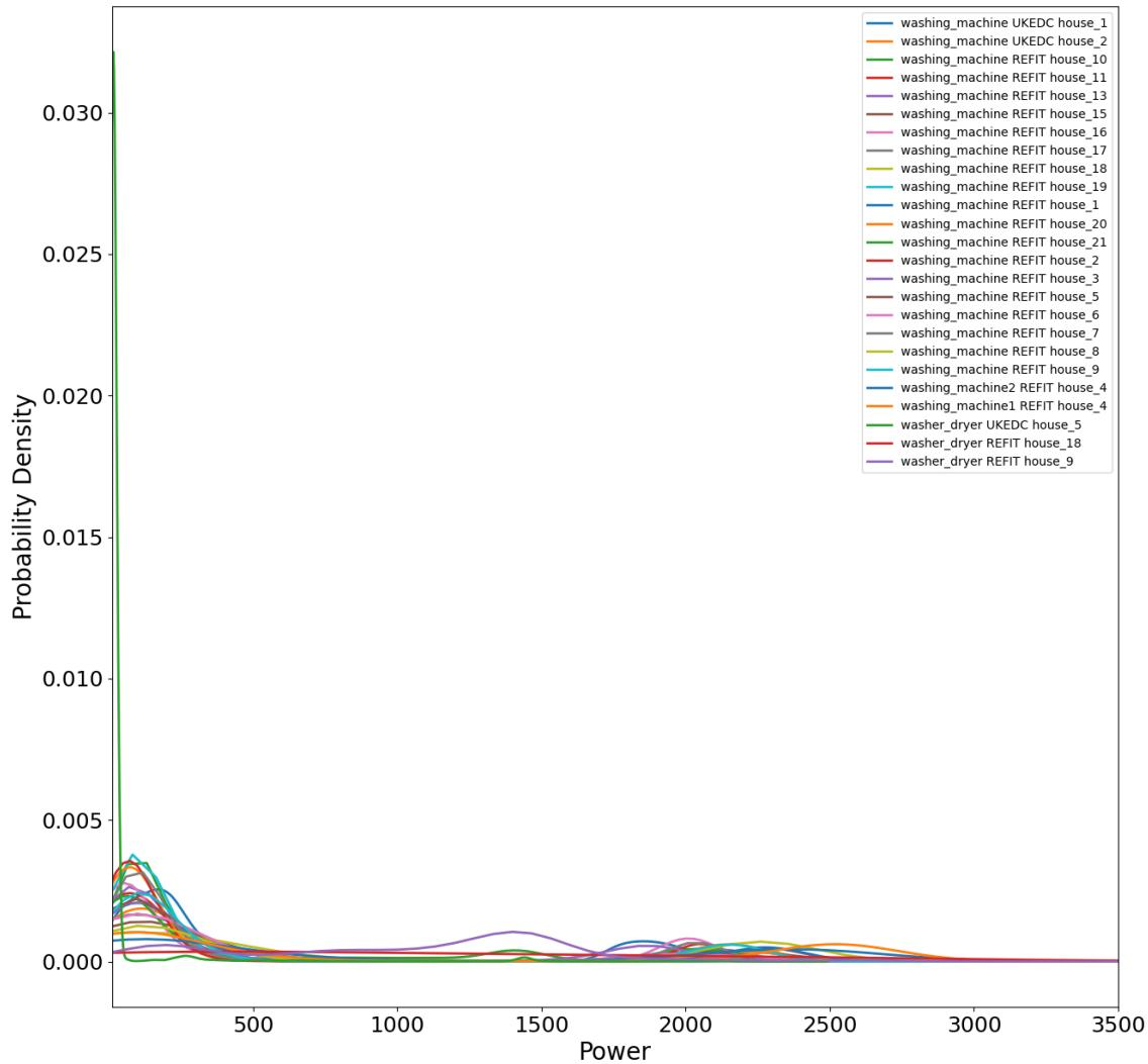
Figure 71: Gaussian kernel-density estimates of the power drawn by each appliance within the washing machine category.
