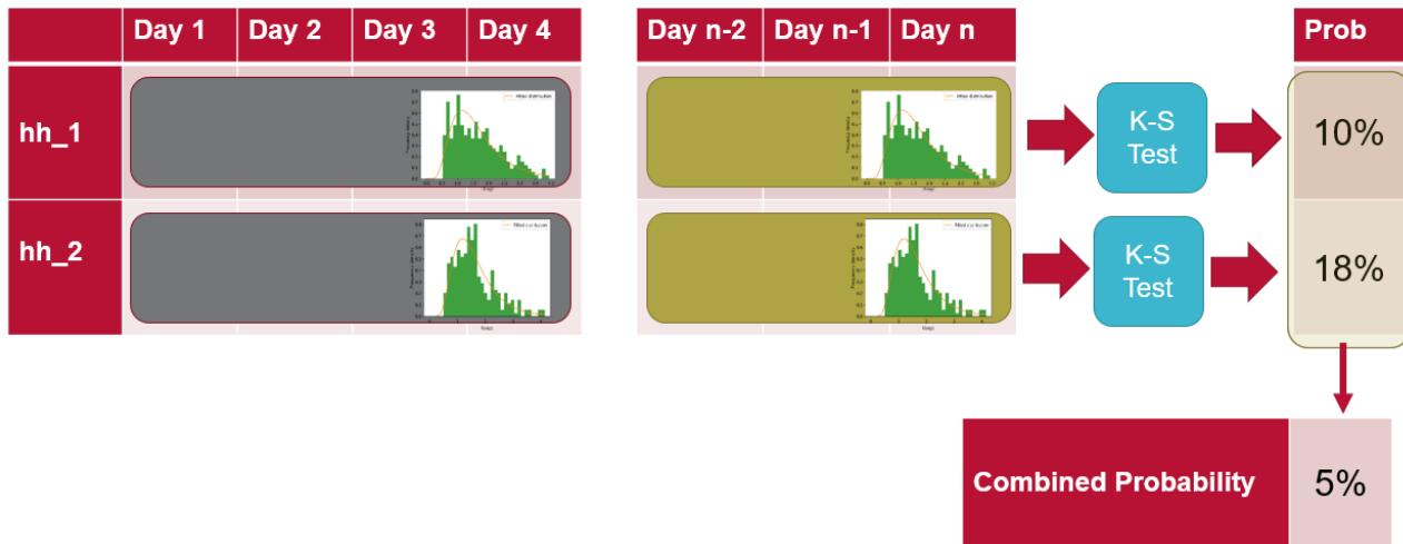
Figure 51: Long term method illustrated for reduced number of days and half hour (hh\_n) periods.
