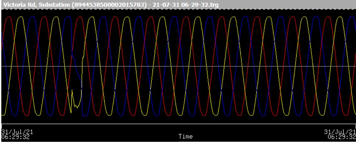
Diagram 10-11 Transitory HV system fault on Y phase
