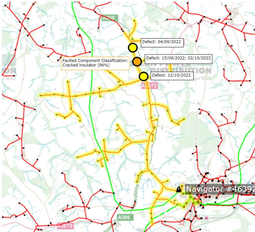
**Figure 4: Example of fault and pre-fault plotting on the SLD annotator.**
