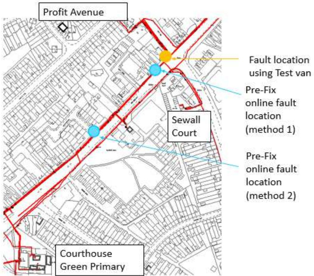
**Figure 10: Recommended fault location vs actual location**
