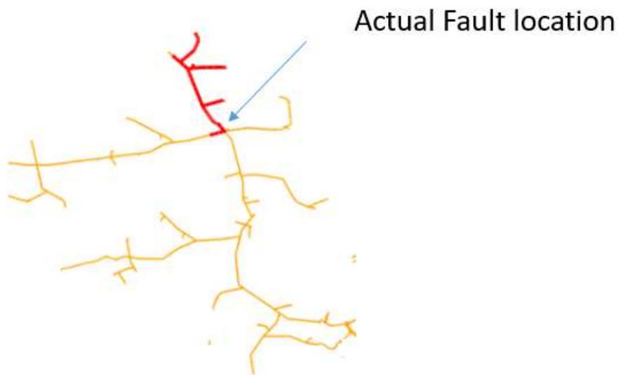
Figure 9: Recommended fault location vs actual location (using prototype system)
