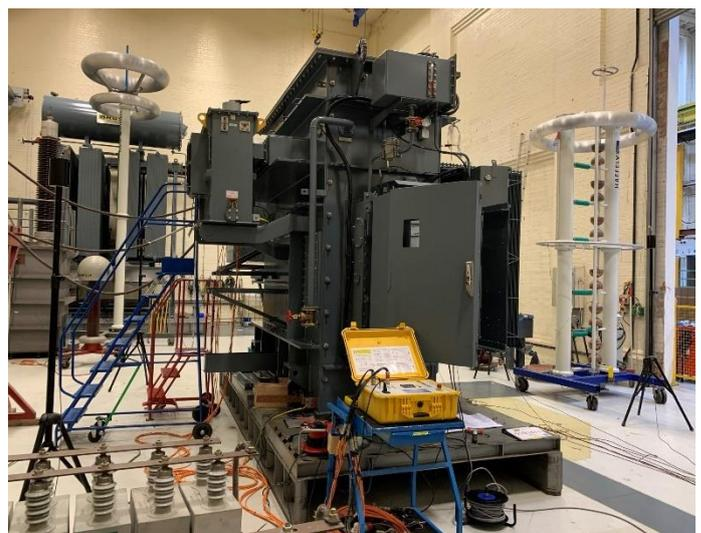
Figure 2 33/11 kV transformer undergoing tests
