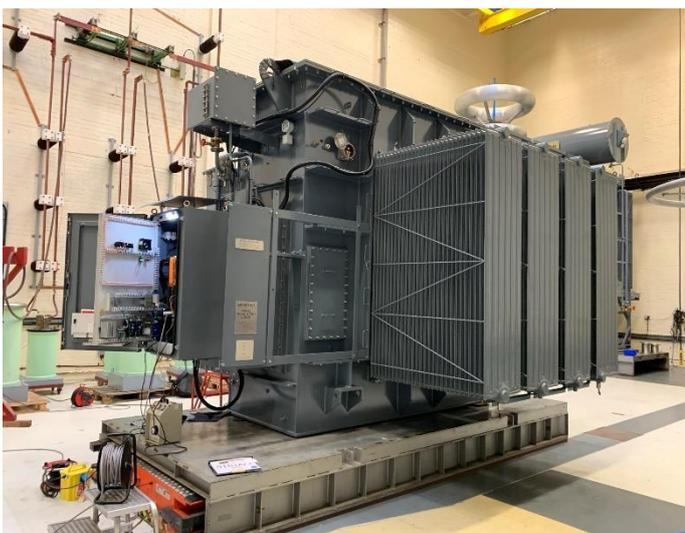
Figure 1 33/11 kV transformer in test laboratory
