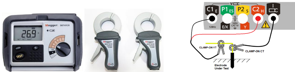
Figure 14: Example of a four-terminal earth tester and clamp-on CT & VT
