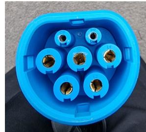
**Type 2 vehicle charging input port**    **Type 2 or Mennekes plug**
