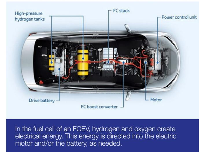
In the fuel cell of an FCEV, hydrogen and oxygen create electrical energy. This energy is directed into the electric motor and/or the battery, as needed.
