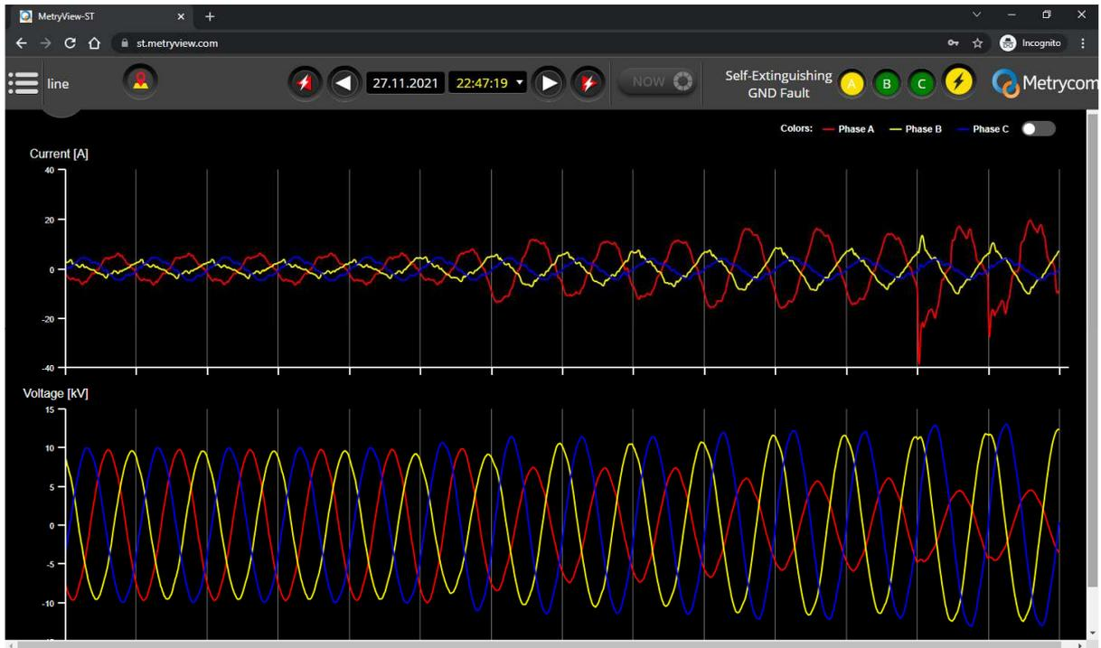
**Figure 6-18: MetryView screenshot showing persistent earth fault current and voltage waveforms for sensor set 43K83**
