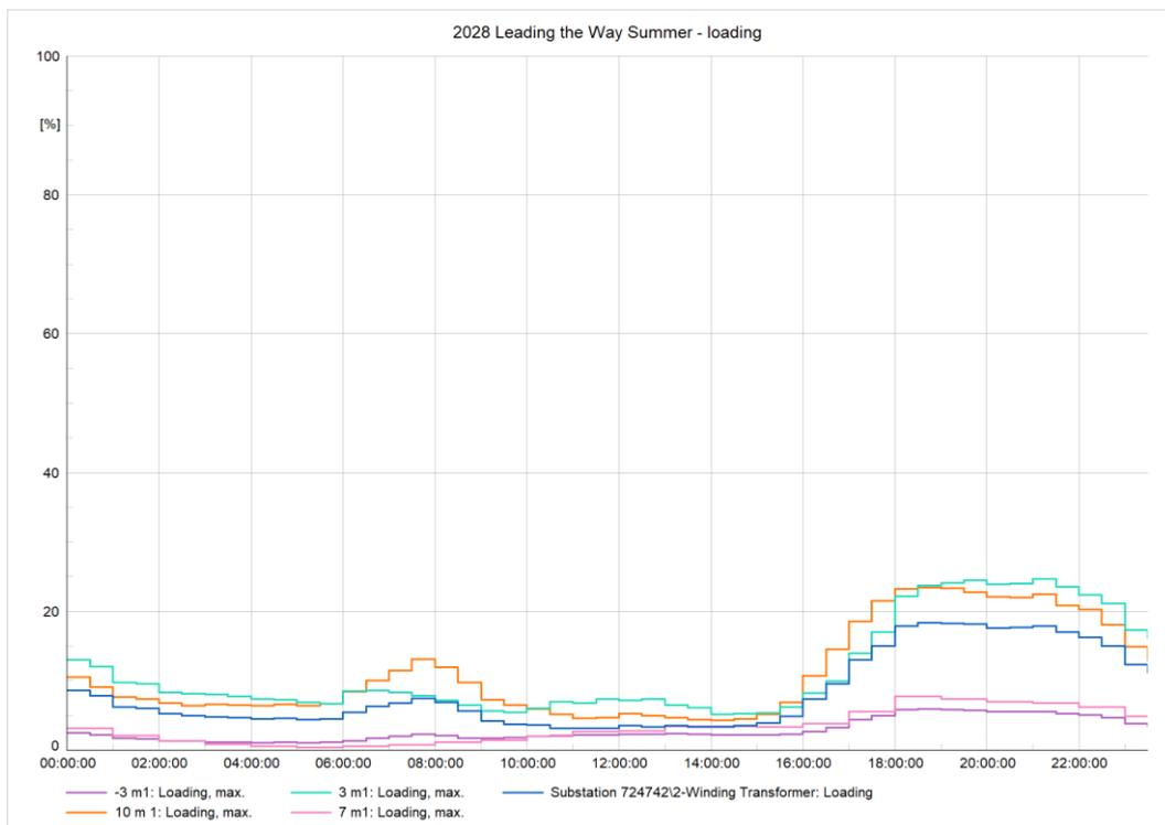
Figure 18 2028 Dense Urban Network Leading the Way summer loading profiles
