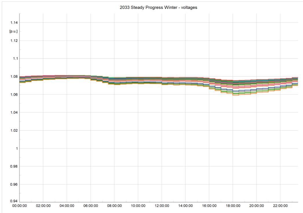
Figure 23 2033 Dense Urban Network Steady Progression winter voltage profiles
