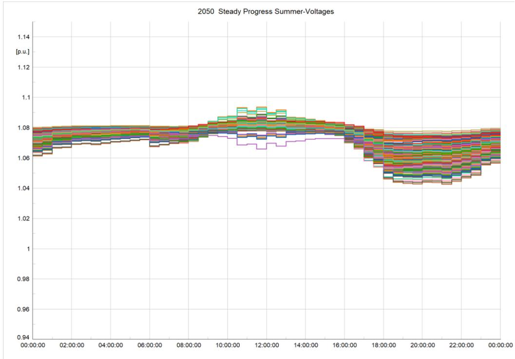
Figure 65 2050 Urban Network Steady Progress summer voltage profiles
