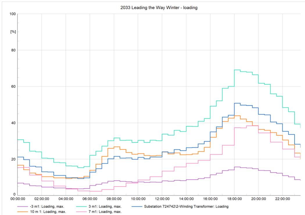
Figure 28 2033 Dense Urban Network Leading the Way Winter load profiles
