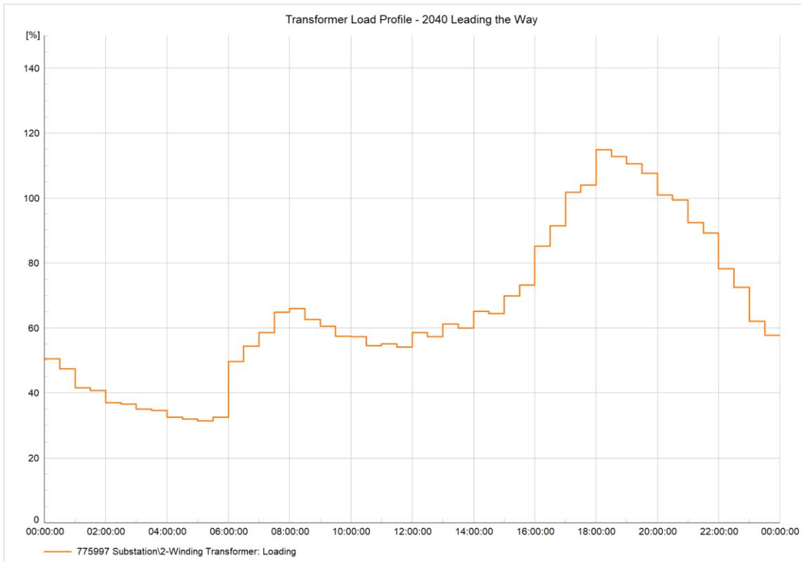
Figure 60 2040 Urban Network Leading the Way transformer loading profiles
