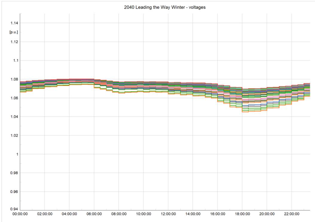
Figure 33 2040 Dense Urban Network Leading the Way winter voltage profiles
