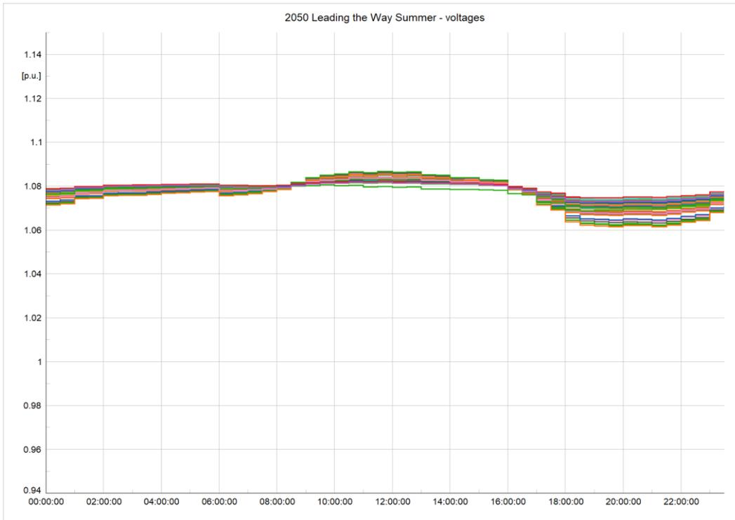
Figure 37 2050 Dense Urban Network Leading the Way summer voltage profiles
