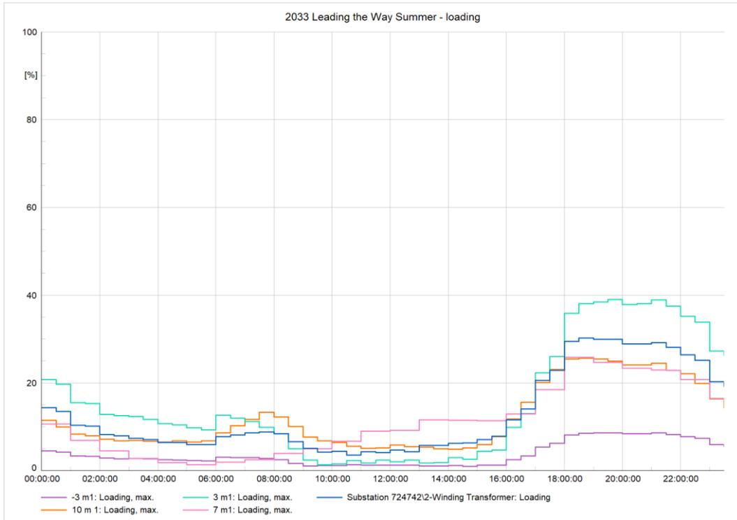
Figure 26 2033 Dense Urban Network Leading the Way Summer load profiles
