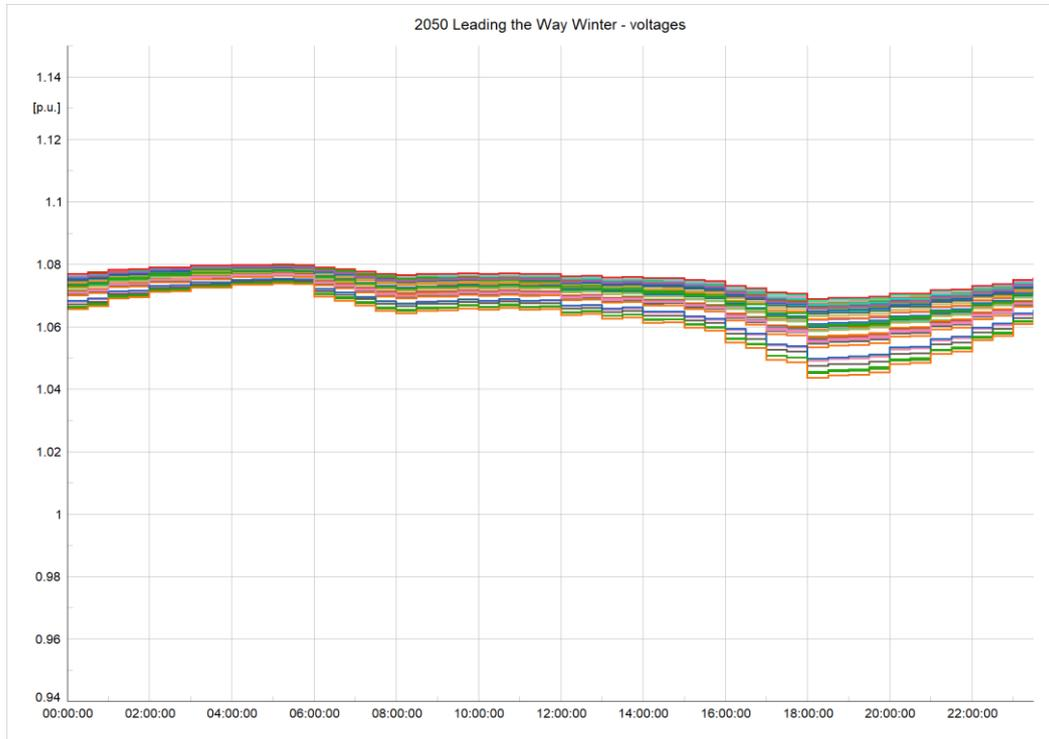
Figure 39 2050 Dense Urban Network Leading the Way winter voltage profiles
