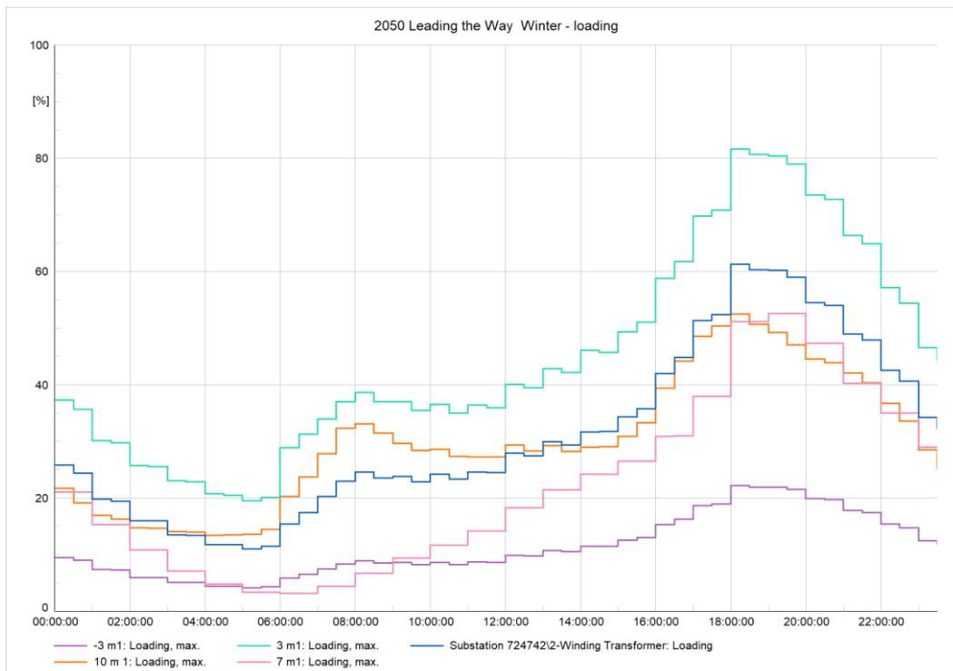
Figure 40 2050 Dense Urban Network Leading the Way winter loading profiles
