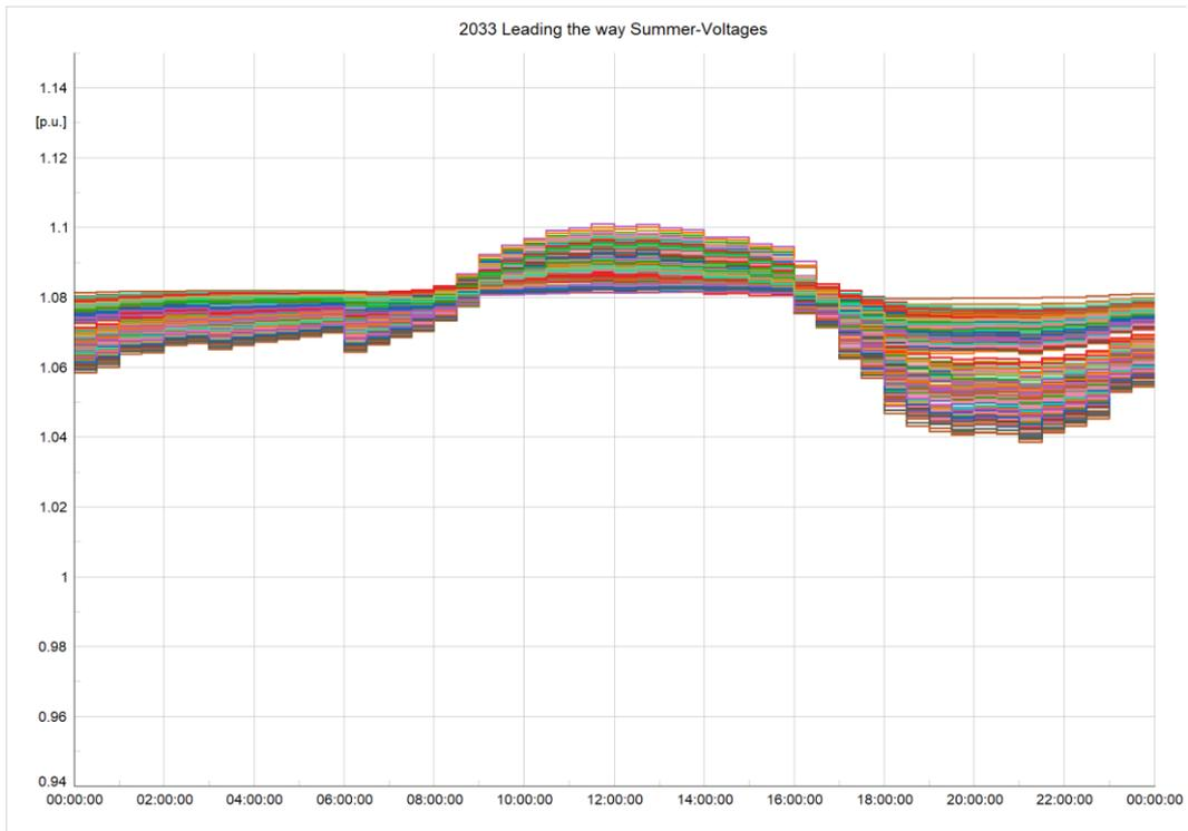
Figure 51 2033 Urban Network Leading the Way summer voltage profiles
