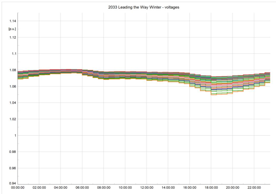
Figure 27 2033 Dense Urban Network Leading the Way Winter voltage profiles
