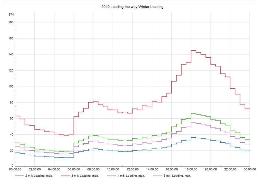
Figure 59 2040 Urban Network Leading the Way Winter loading profiles
