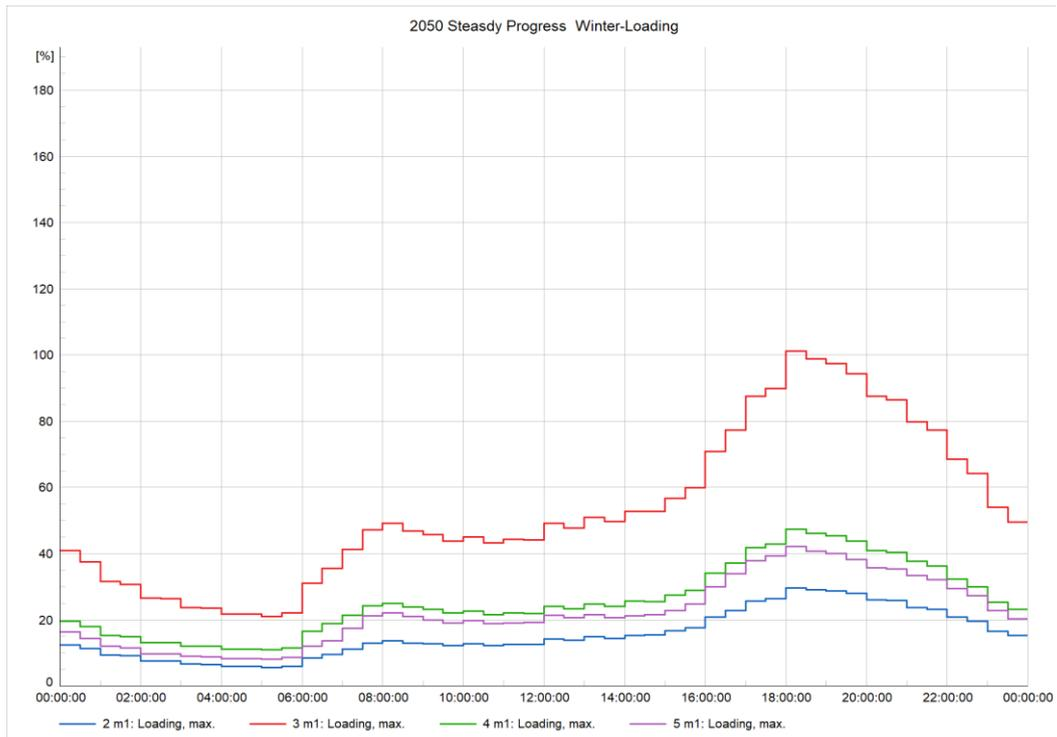
Figure 66 2050 Urban Network Steady Progress winter loading profiles
