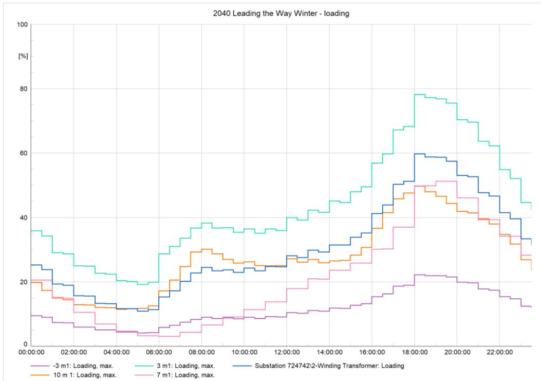
Figure 34 2040 Dense Urban Network Leading the Way winter loading profiles
