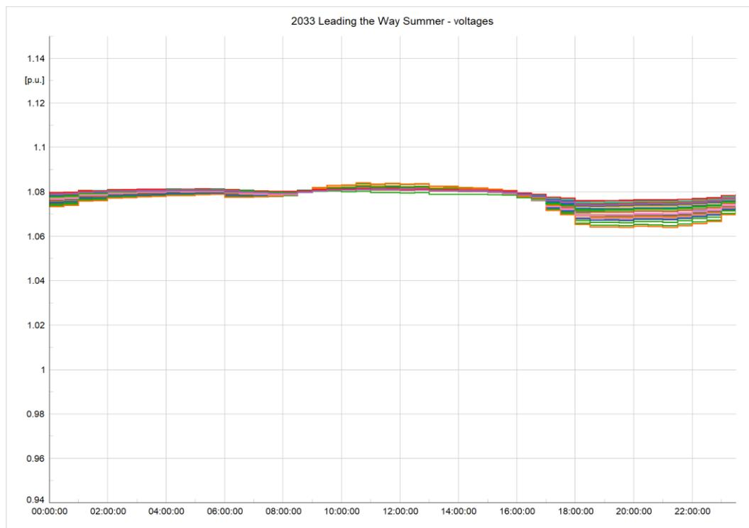
Figure 25 2033 Dense Urban Network Leading the Way Summer voltage profiles
