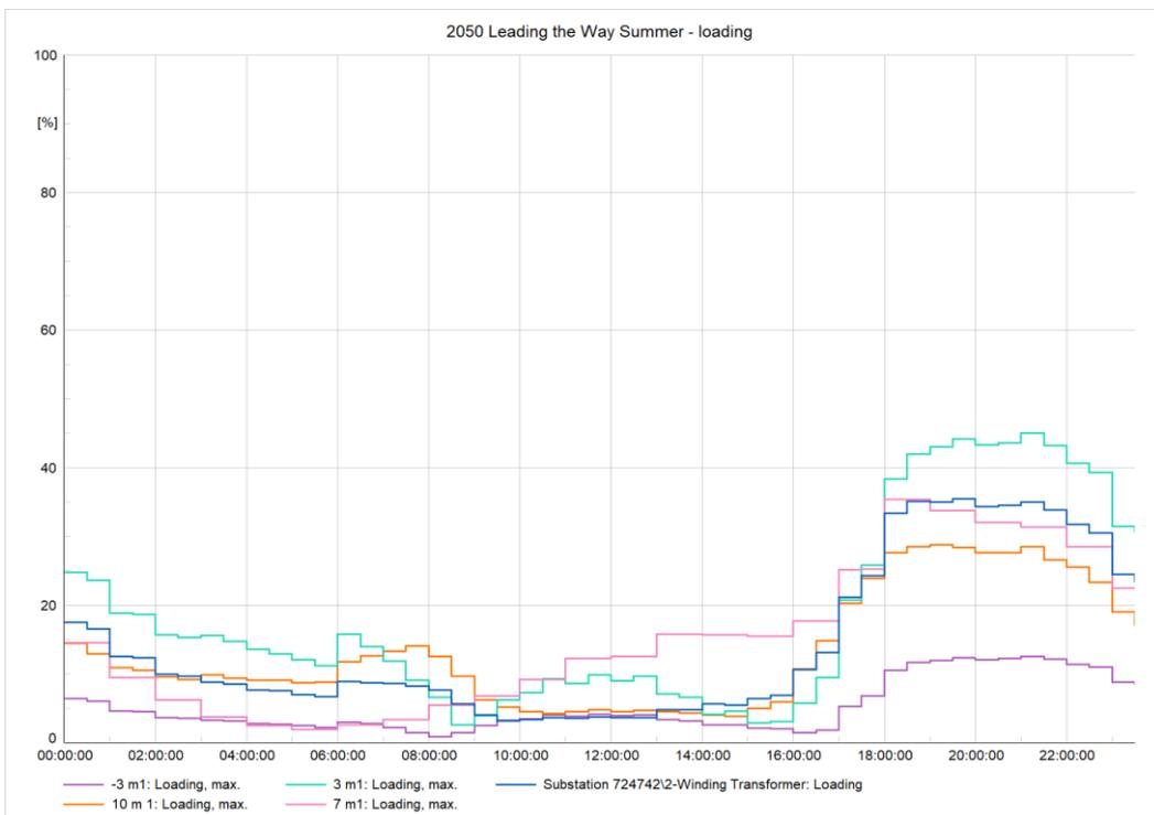
Figure 38 2050 Dense Urban Network Leading the Way summer loading profiles
