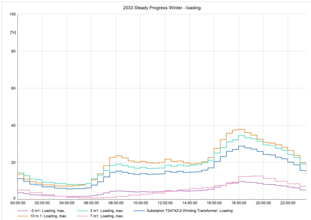
Figure 24 2033 Dense Urban Network Steady Progression winter loading profiles
