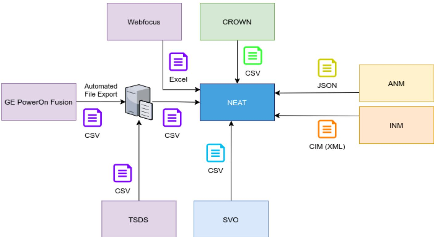
Figure 1 How data from WPD systems is imported into NEAT.
