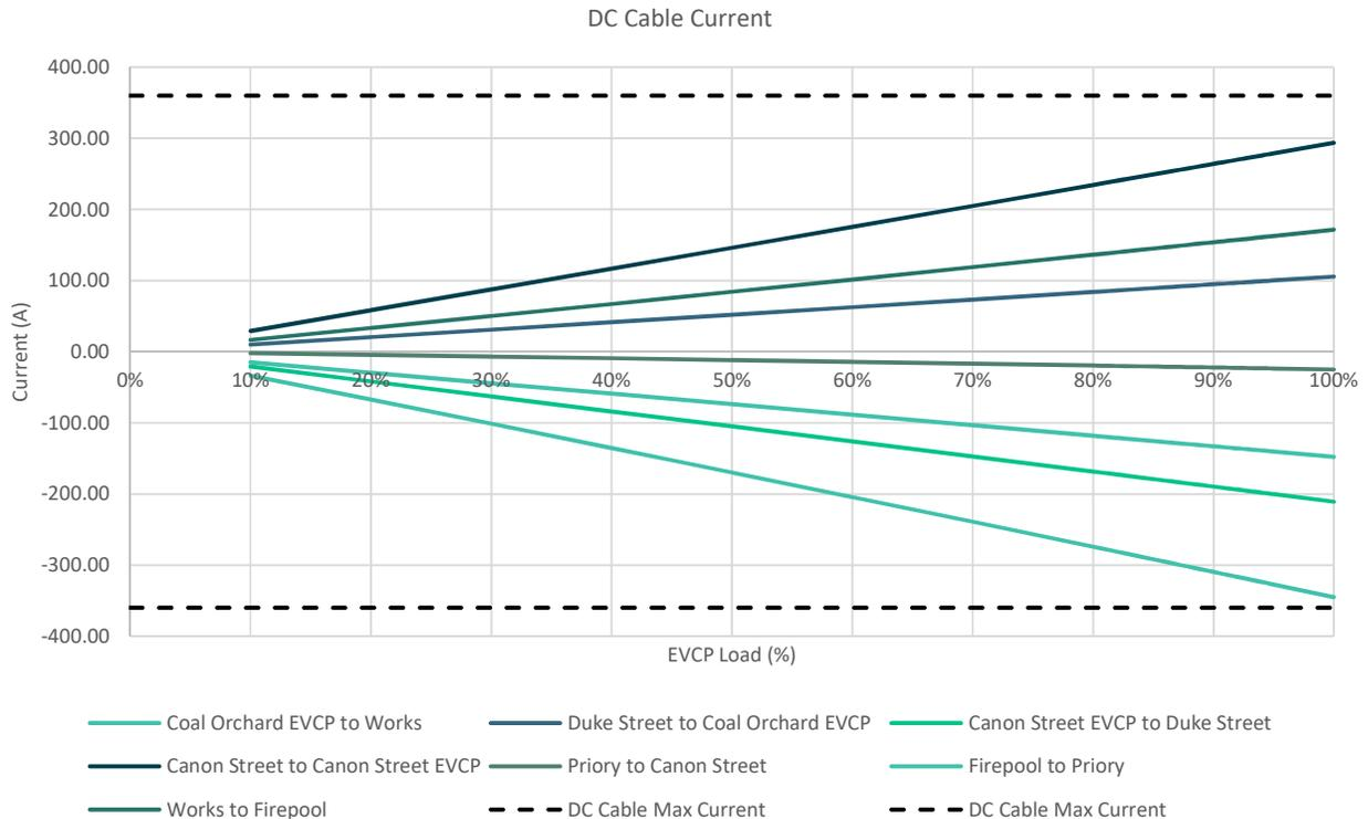
Figure 13: Current flow in the DC cable network
