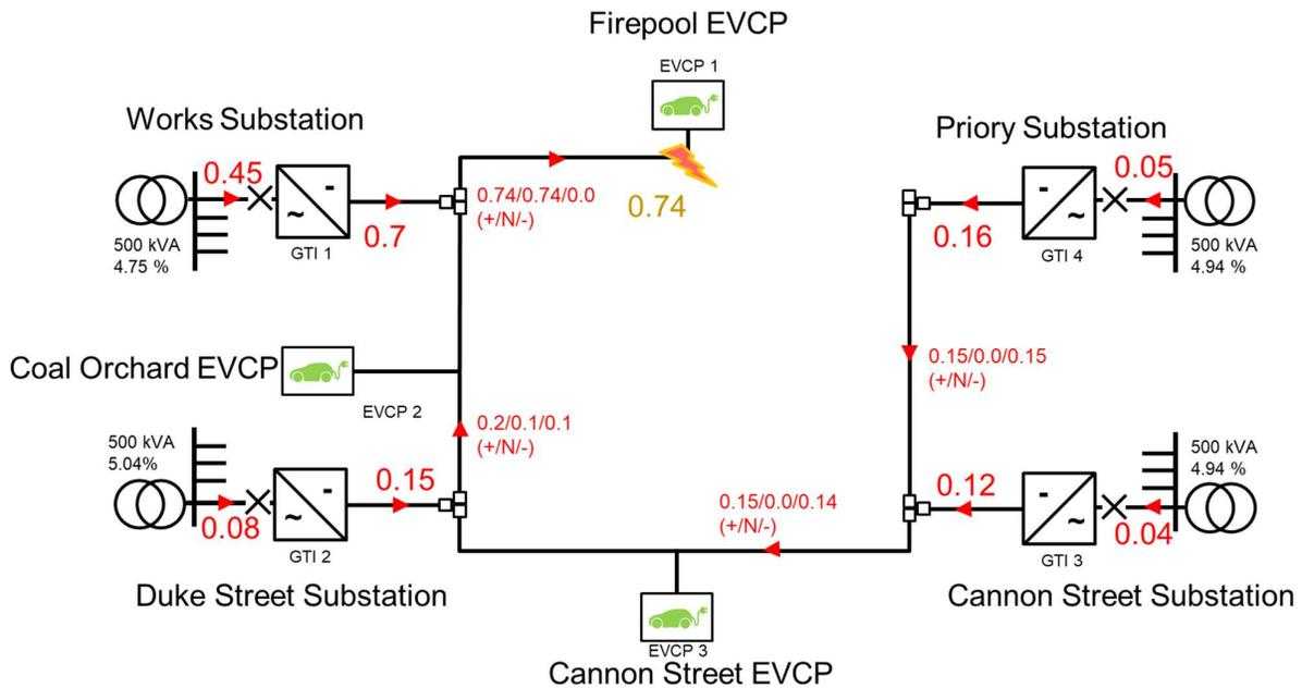
Figure 17. N-1 Scenario minimum Fault Level Summary in A
