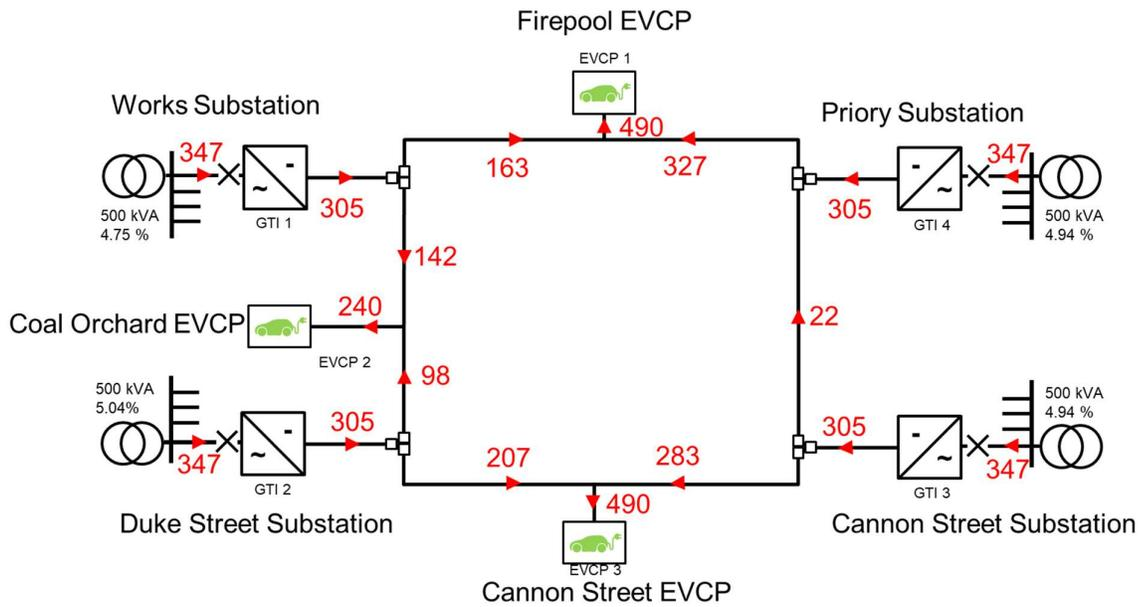
Figure 18. Maximum loading (Intact System) in A
