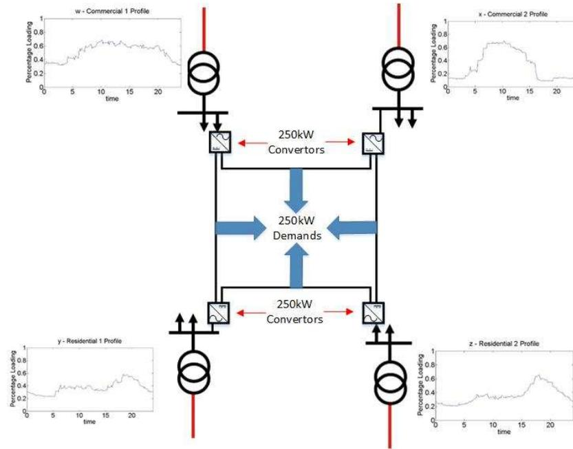
Figure 1: Example of capacity creation through dissimilar load profiles (before equalisation)
