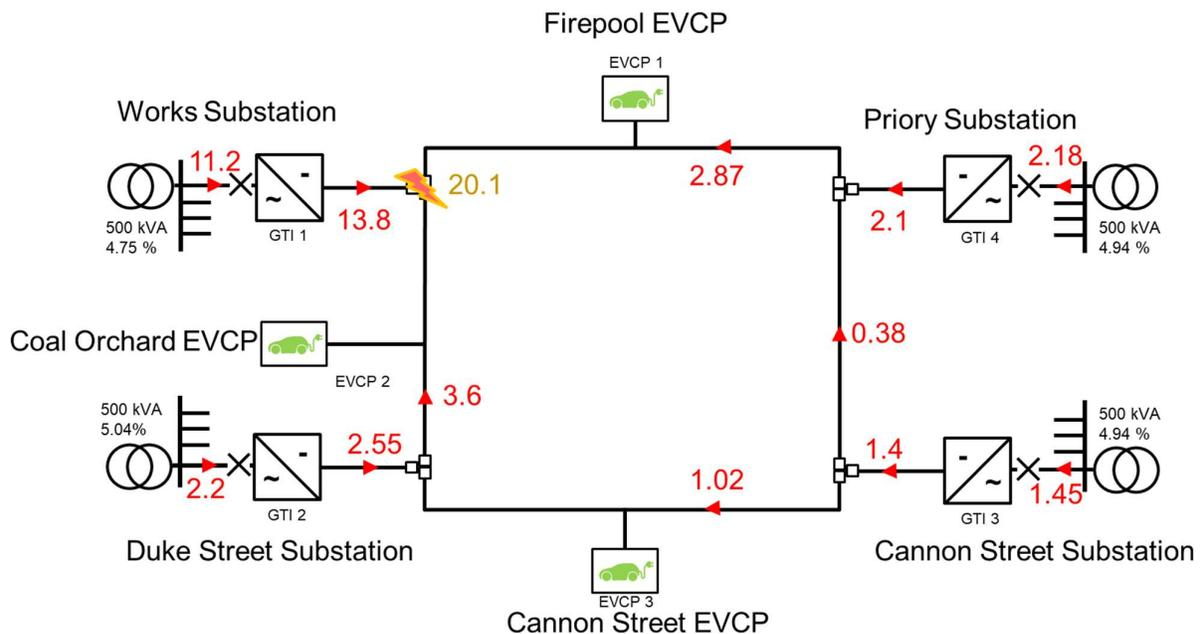
Figure 15. System intact maximum Fault Level Summary in kA
