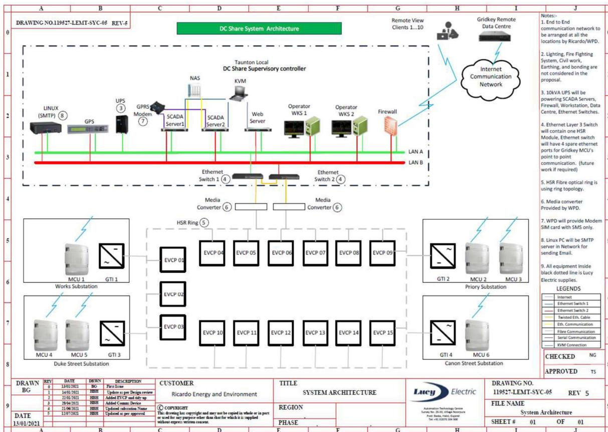
Figure 31. Supervisory Controller system Architecture
