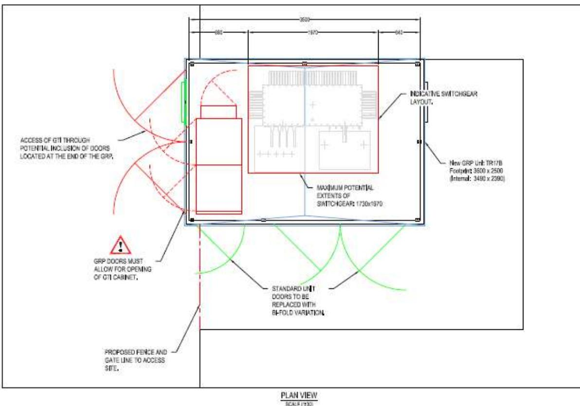
Figure 26: GTI installation in a GRP substation.
