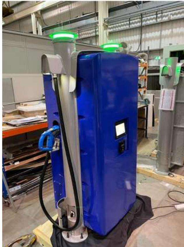
*Figure 27: EVCP in construction in the TPS works*
