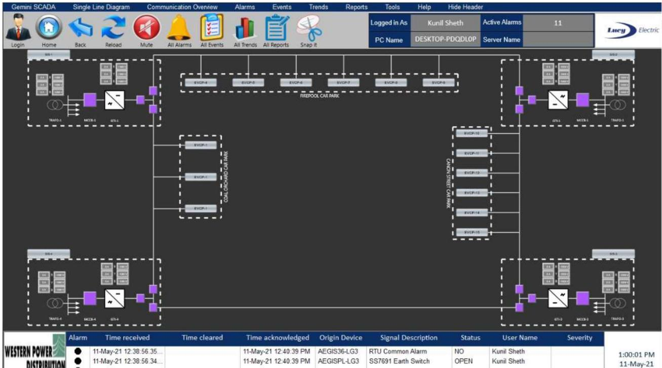
Figure 33. Network Overview Control scheme (Typical)
