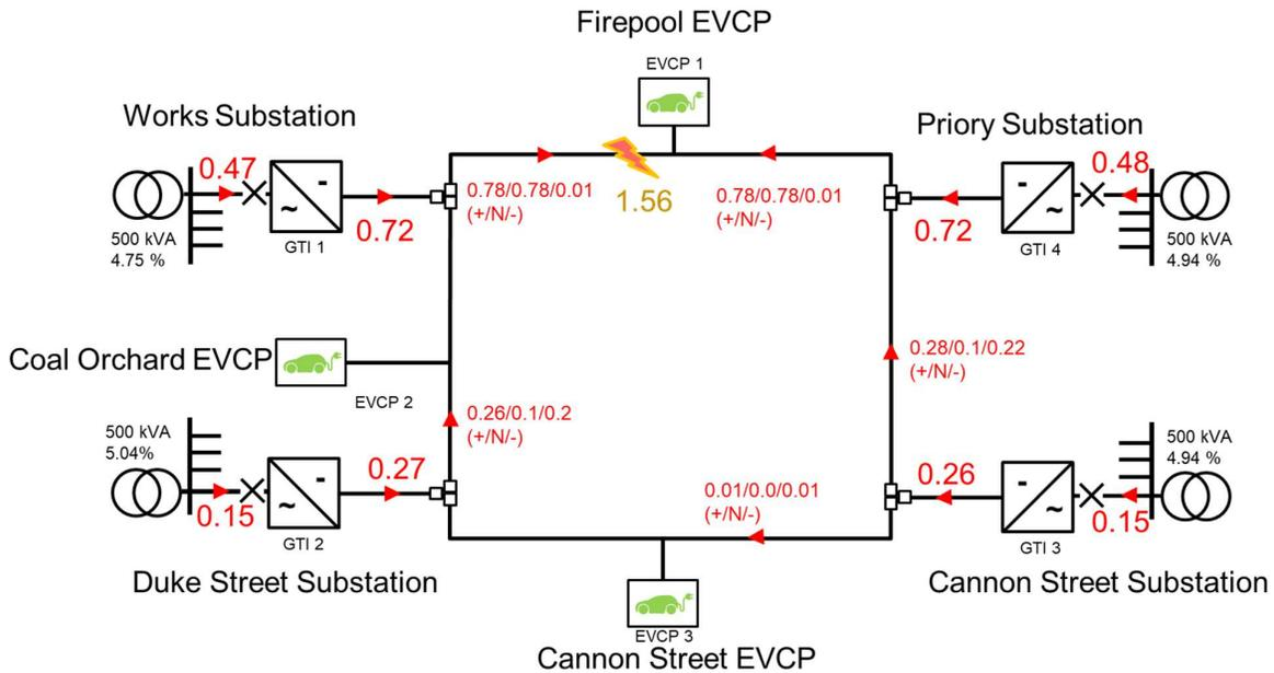
Figure 16. System intact minimum Fault Level Summary in kA
