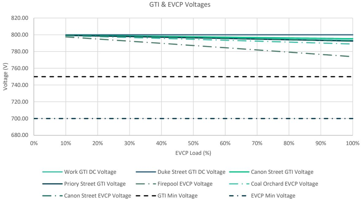
Figure 12: DC voltages required on the DC side of the GTI to share the load equally between the four GTIs and the EVCP voltages
