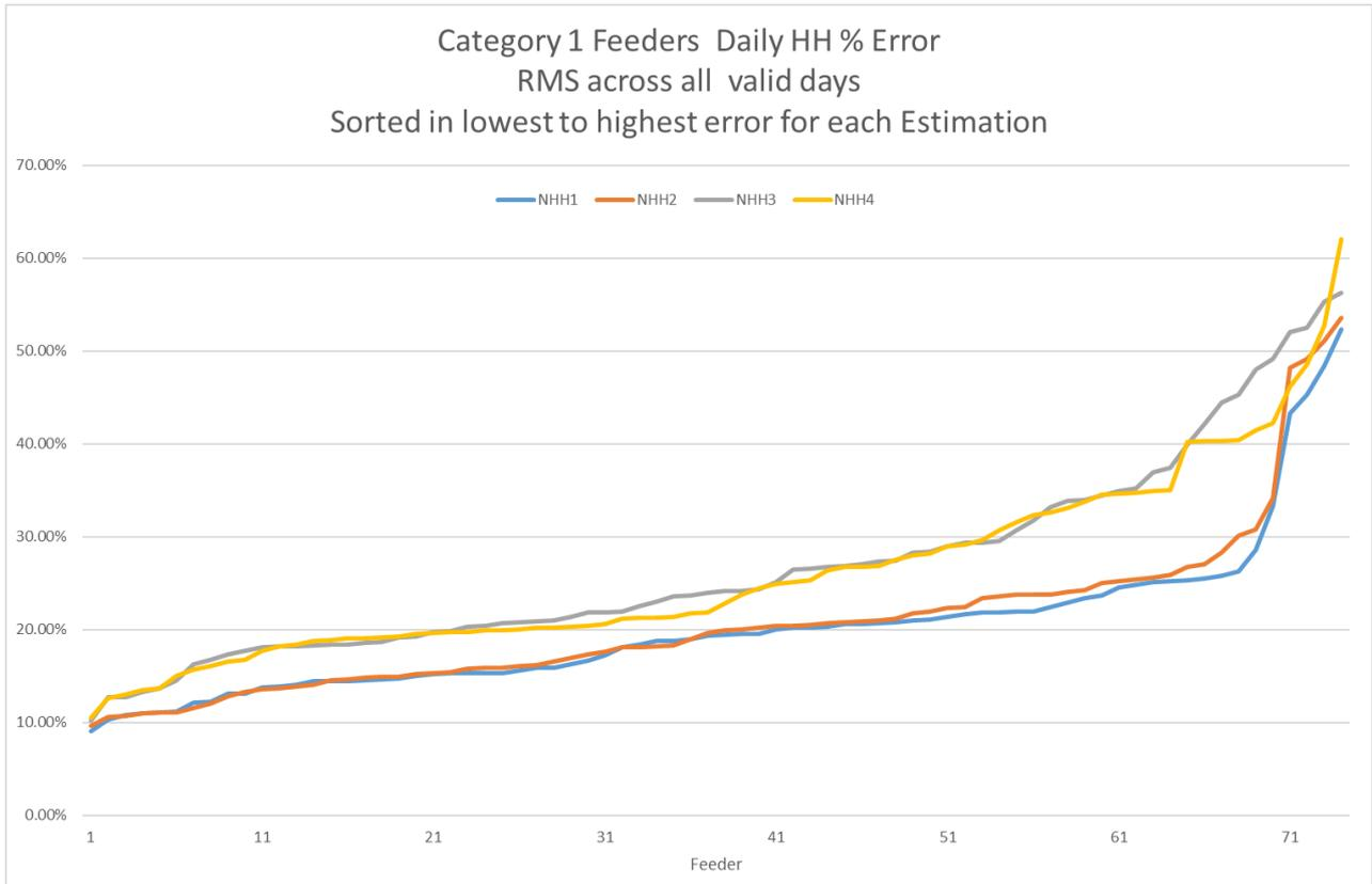
**Figure 18 - Feeder Category 1 RMS HH Profile Error**
