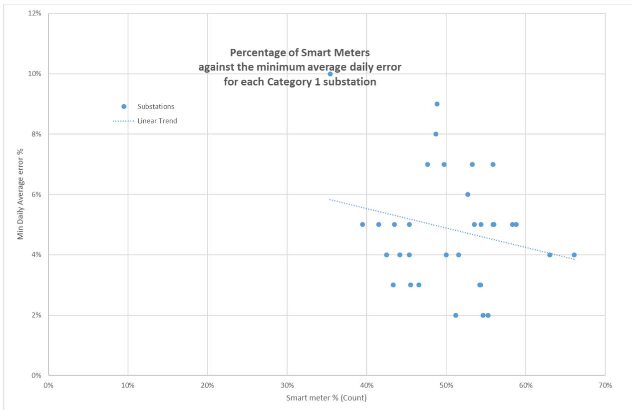
**Figure 57 - Smart Meter Population against estimation error**
