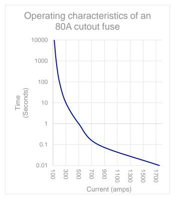
The characteristics of an 80A fuse can be seen above.
