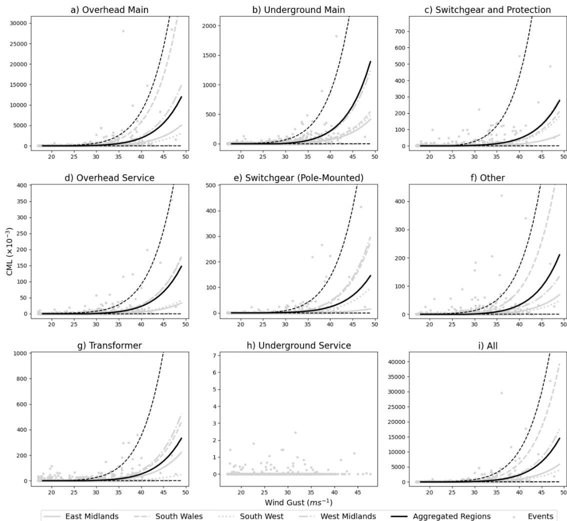
Figure 2 Example fragility curves showing the relationships between wind gust intensity and CML in a windstorm for each asset type.
