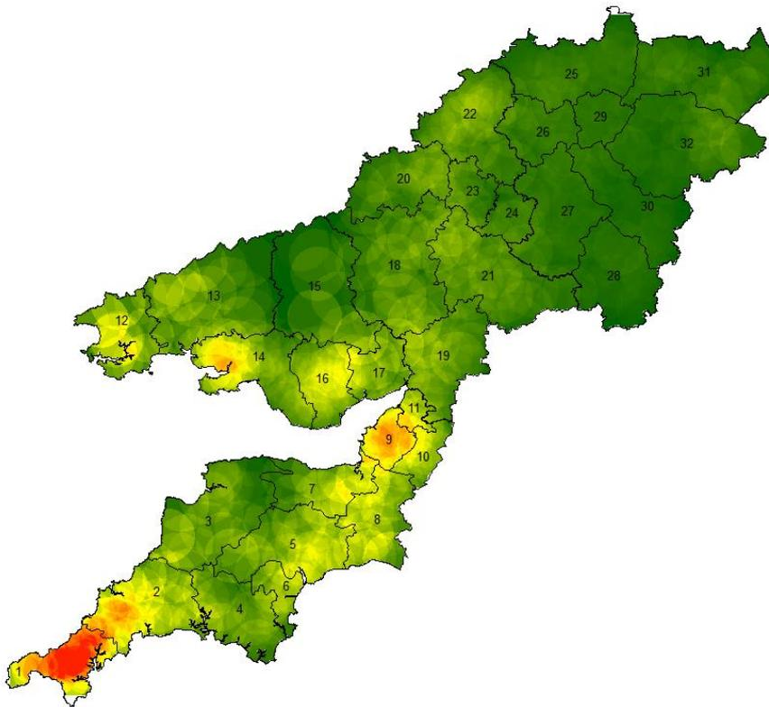
Figure 1 Example heatmap showing number of wind-related faults per primary substation shown on a red/green scale, where red indicates a high number of faults). The highest number of faults recorded is 283.
