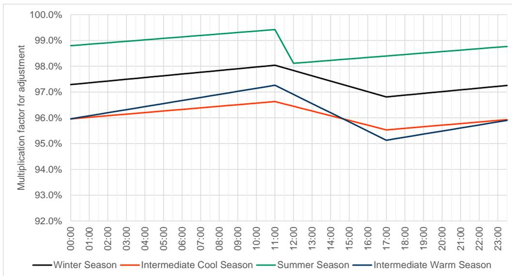
Figure 13 Primary substation 2050 demand half-hourly adjustment factors (example for Bodmin primary)
