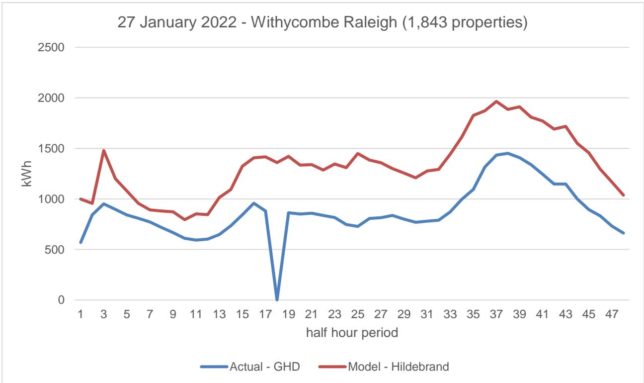
Figure 49 Comparison of model to actual electricity demand in kilowatts for all of Withycombe Raleigh
