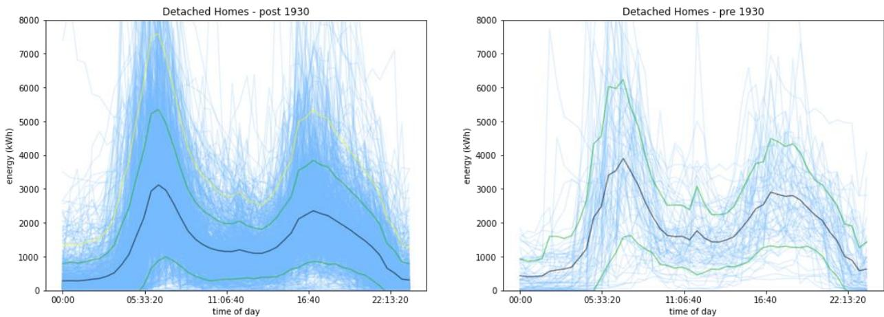
**Figure 15 Gas usage for Detached Homes, pre and post 1930 construction by half hour for all days of the heating season. The black line is the mean with green one standard deviation above/below, yellow line is 2 standard deviations.**
