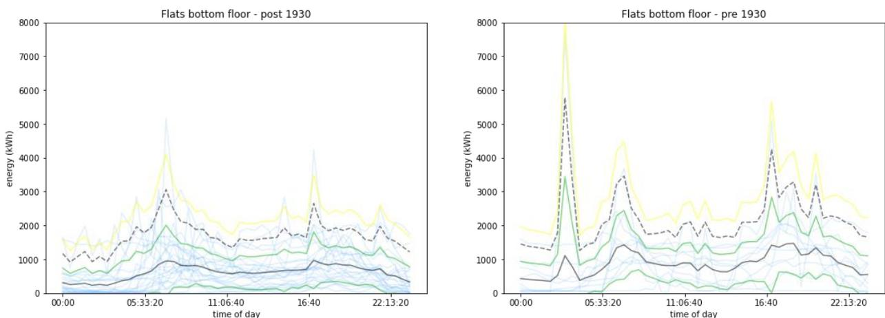
**Figure 19 Gas usage for Bottom floor flats, pre and post 1930 construction by half hour for all days of the heating season. The black line is the mean with green one standard deviation above/below, yellow line is 2 standard deviations.**
