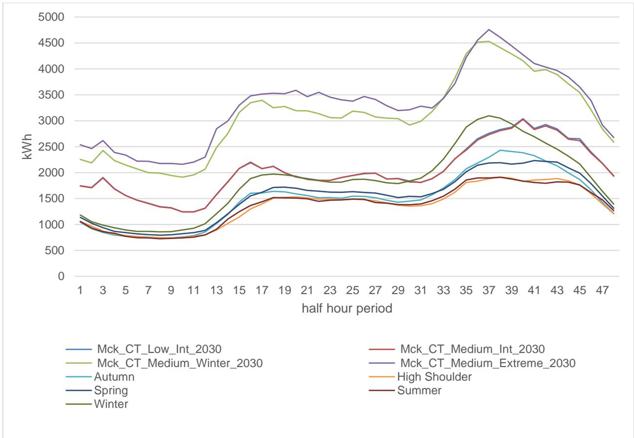
**Figure 34 Energy profiles comparing Elexon Profile Class 1 half hour by season for the whole of Mackworth (approximately 3,363 homes). Scenario labels are the same as above, reduced number to be able to fit on to graph.**
