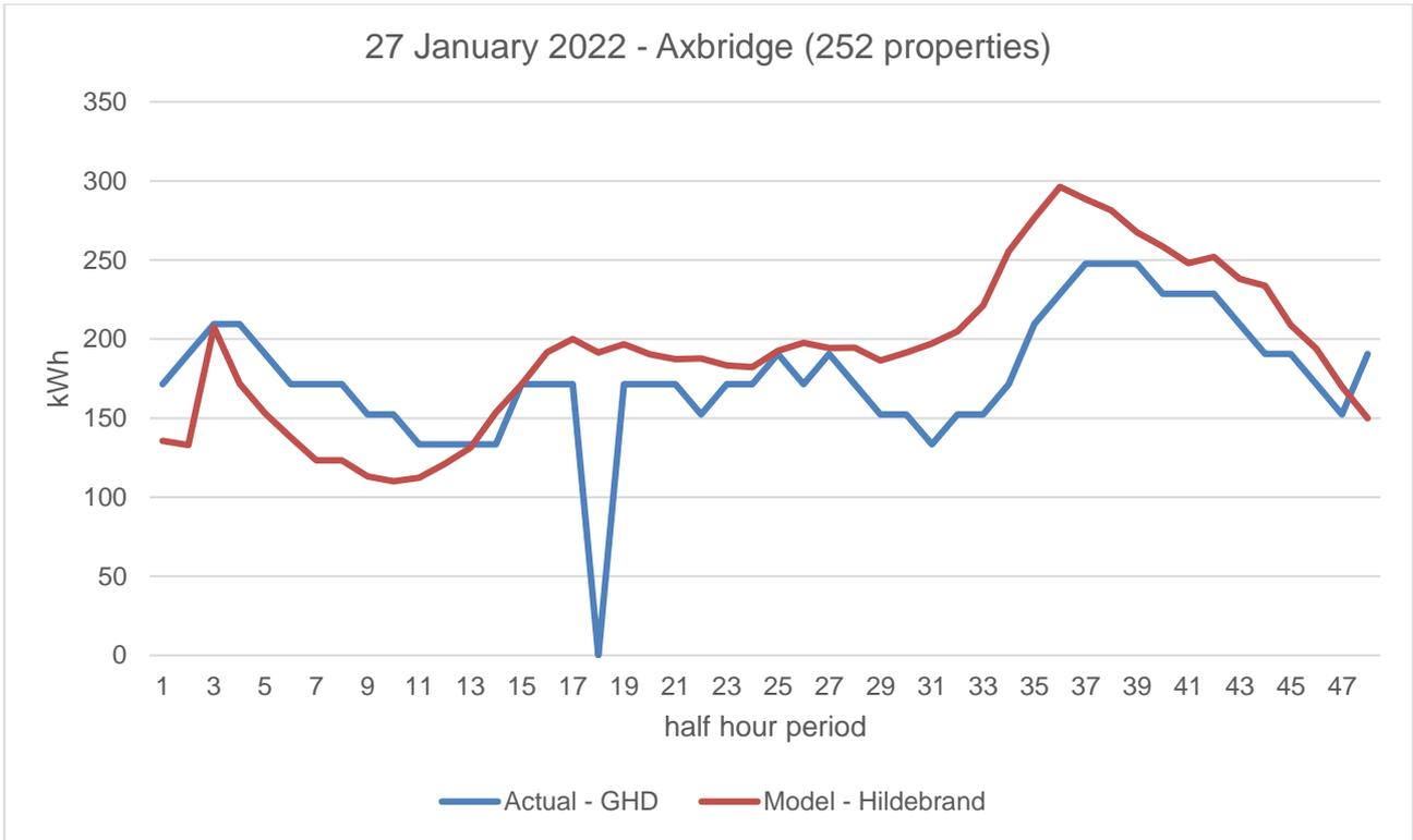
Figure 48 Comparison of model to actual electricity demand in kilowatts for all of Axbridge
