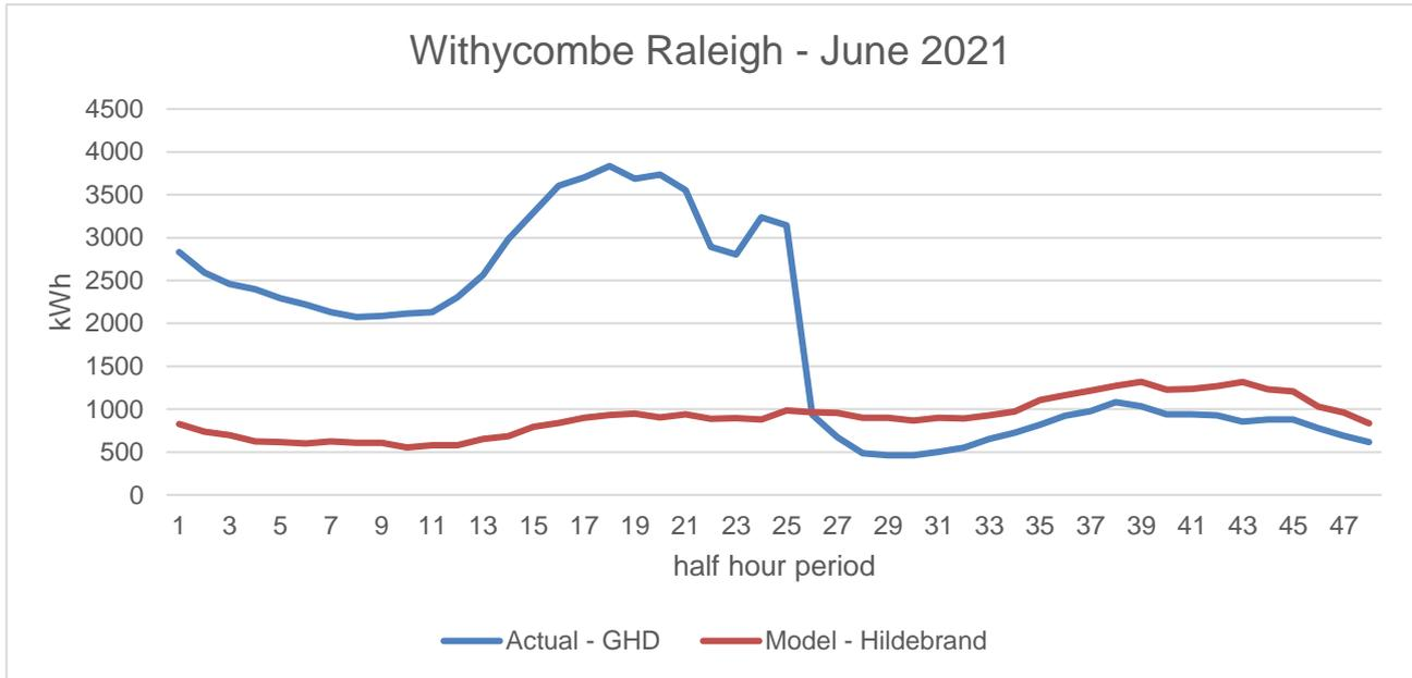
Figure 52 Large overnight load in June 2021 for Withycombe Raleigh which is an anomaly
