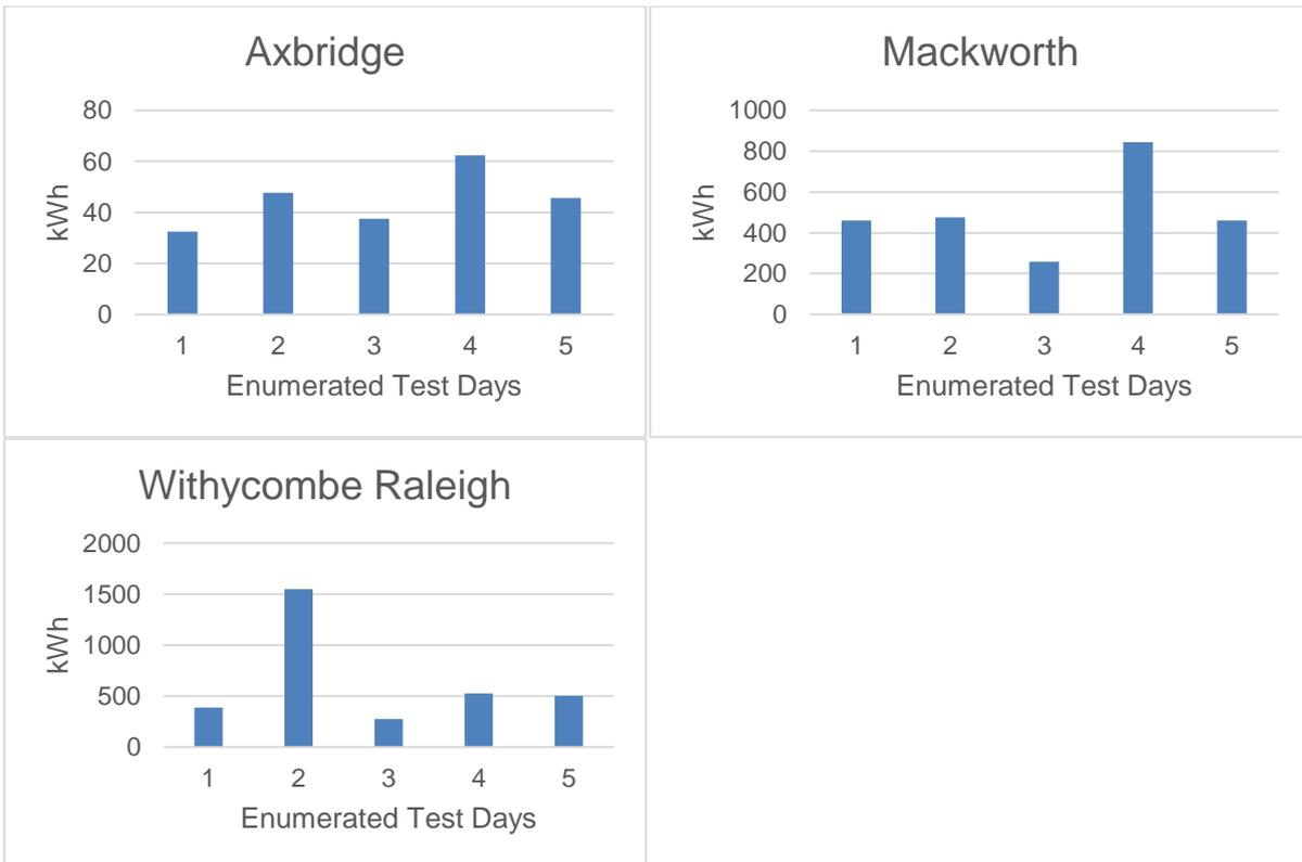
Figure 51 Root mean squared error over the five different test days, error is in kWh for the entire day. Days 1 (March) and 5 (January) are representative of heating days.
