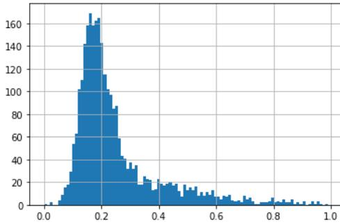
**Figure 8 Histogram of ratio night to total electricity consumption; at approximately 30% there is a new cluster of properties**
