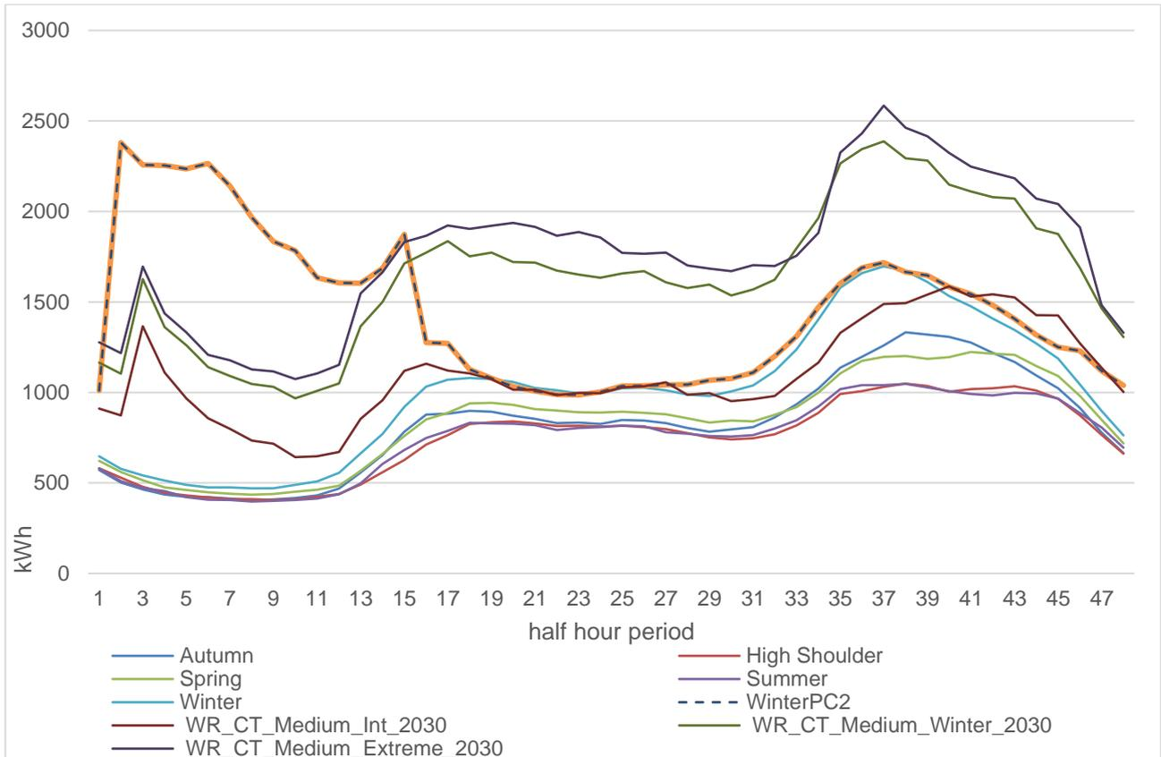
**Figure 33 Energy profiles comparing Elexon Profile Class 1 half hour for the whole of WithycombeRaleigh (approximately 1,843 homes). Winter PC2 applies a Elexon Profile Class 2 (night storage heater) to all of the homes. Scenario labels are the same as above, reduced number to be able to fit on to graph.**
