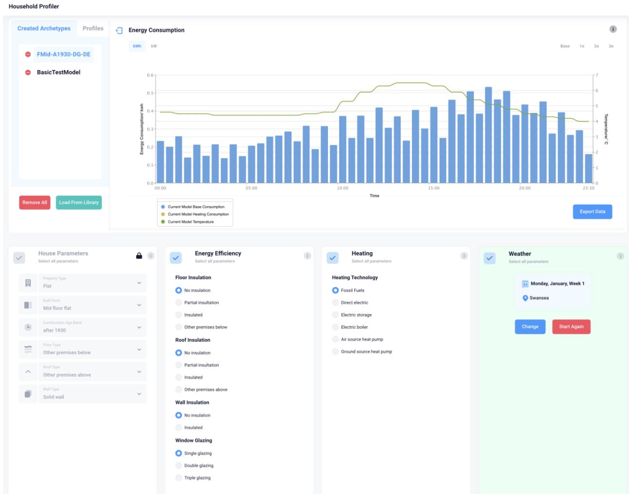
**Figure 12 Example parameters selected to generate half hourly electricity profiles. The Property Type, Built Form and date parameters drive the generation of the profile.**
