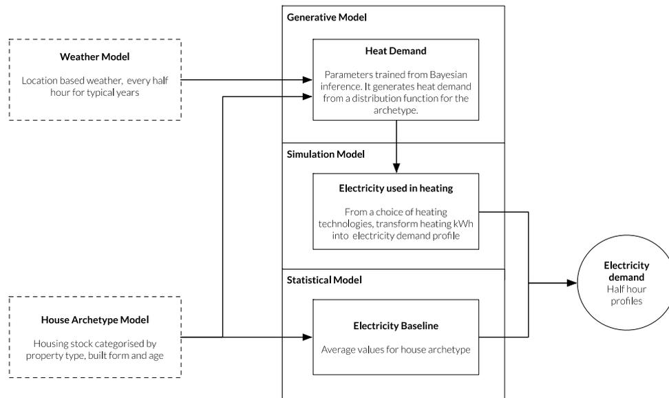
**Figure 2 Details of the model elements as they are used to generate data; the data sources and model parameters are in the code running on an end user's browser**
