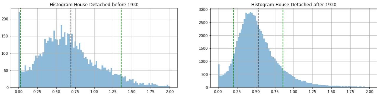
**Figure 20 Detached houses before 1930 have a higher spread of values and overall worse energy efficiency**
