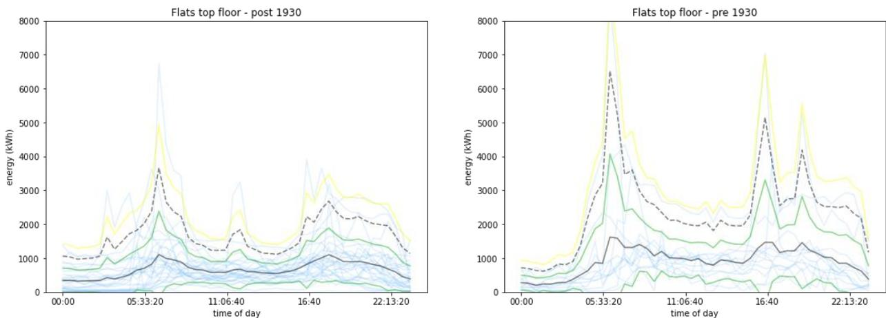
**Figure 18 Gas usage for Top floor flats, pre and post 1930 construction by half hour for all days of the heating season. The black line is the mean with green one standard deviation above/below, yellow line is 2 standard deviations.**
