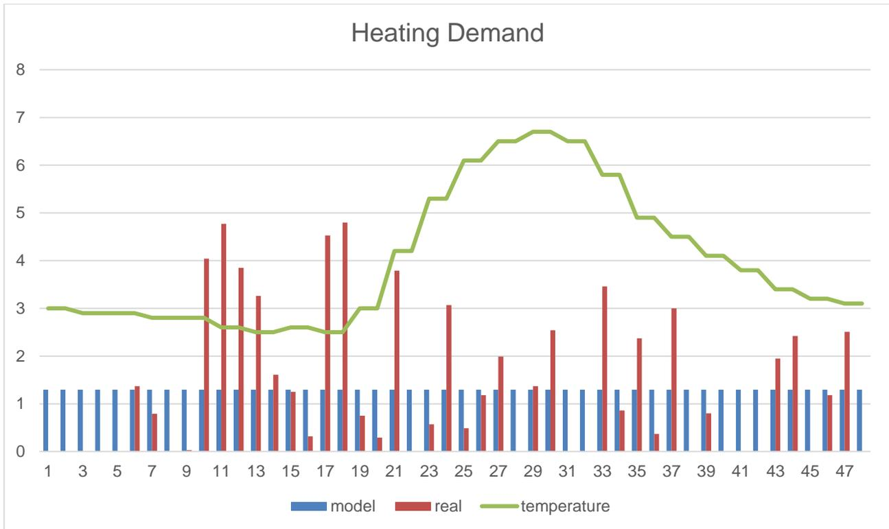
Figure 47 Model (blue) energy for heat and real gas usage (red) for a Thursday 27 January 2022, both in kWh units. Temperature is overlaid in green. A heat pump model is used for the simulated data.
