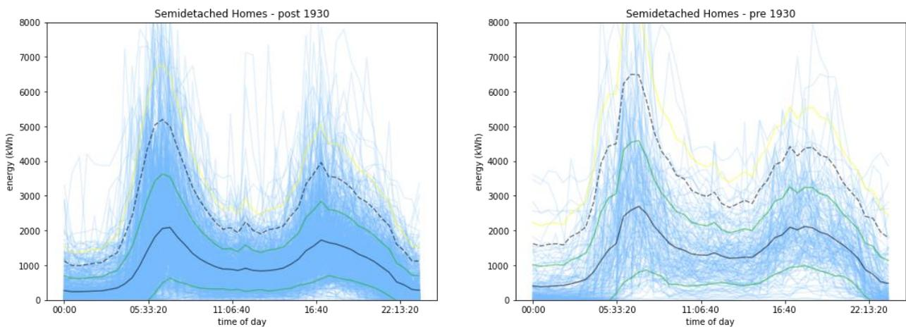
**Figure 16 Gas usage for Semi-detached Homes, pre and post 1930 construction by half hour for all days of the heating season. The black line is the mean with green one standard deviation above/below, yellow line is 2 standard deviations.**
