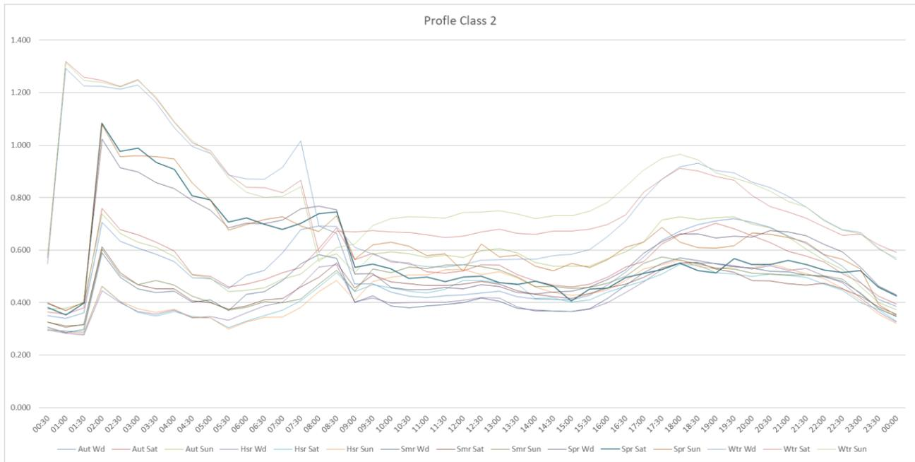
**Figure 41 Average half hourly power consumption of Profile Class 2 meters, collected over a 10 year period by Elexon**
