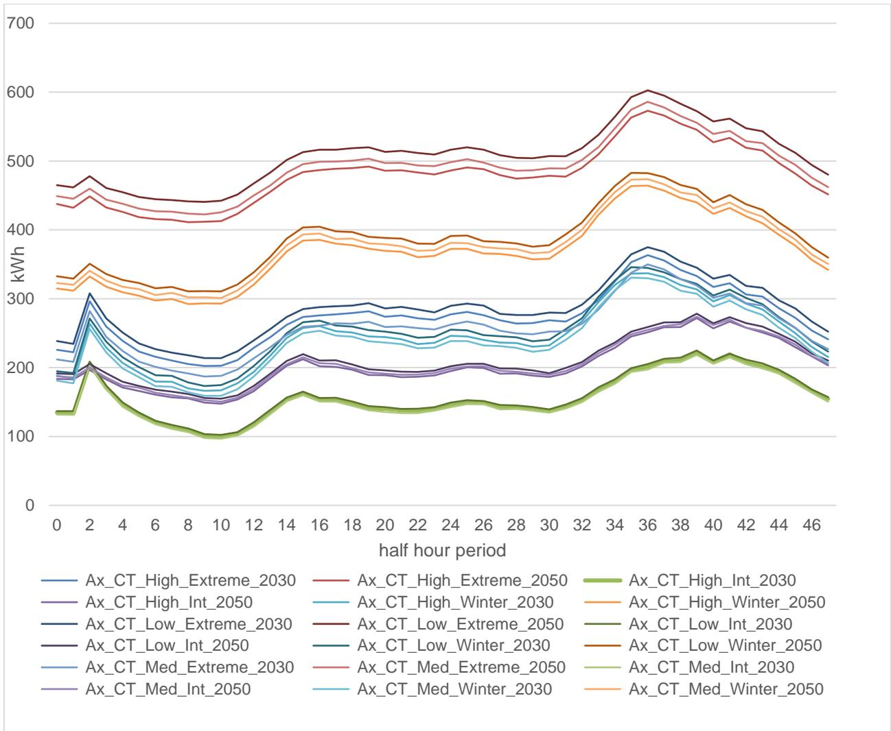
**Figure 32 Energy profiles for heating simulated for the whole of Axbridge (approximately 252 homes) and takeup of heat pumps using percentage offsets to the HTC random variable, results are in the expected order**
