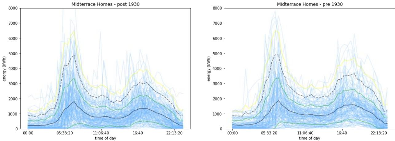
**Figure 17 Gas usage for Midderrace Homes, pre and post 1930 construction by half hour for all days of the heating season. The black line is the mean with green one standard deviation above/below, yellow line is 2 standard deviations.**
