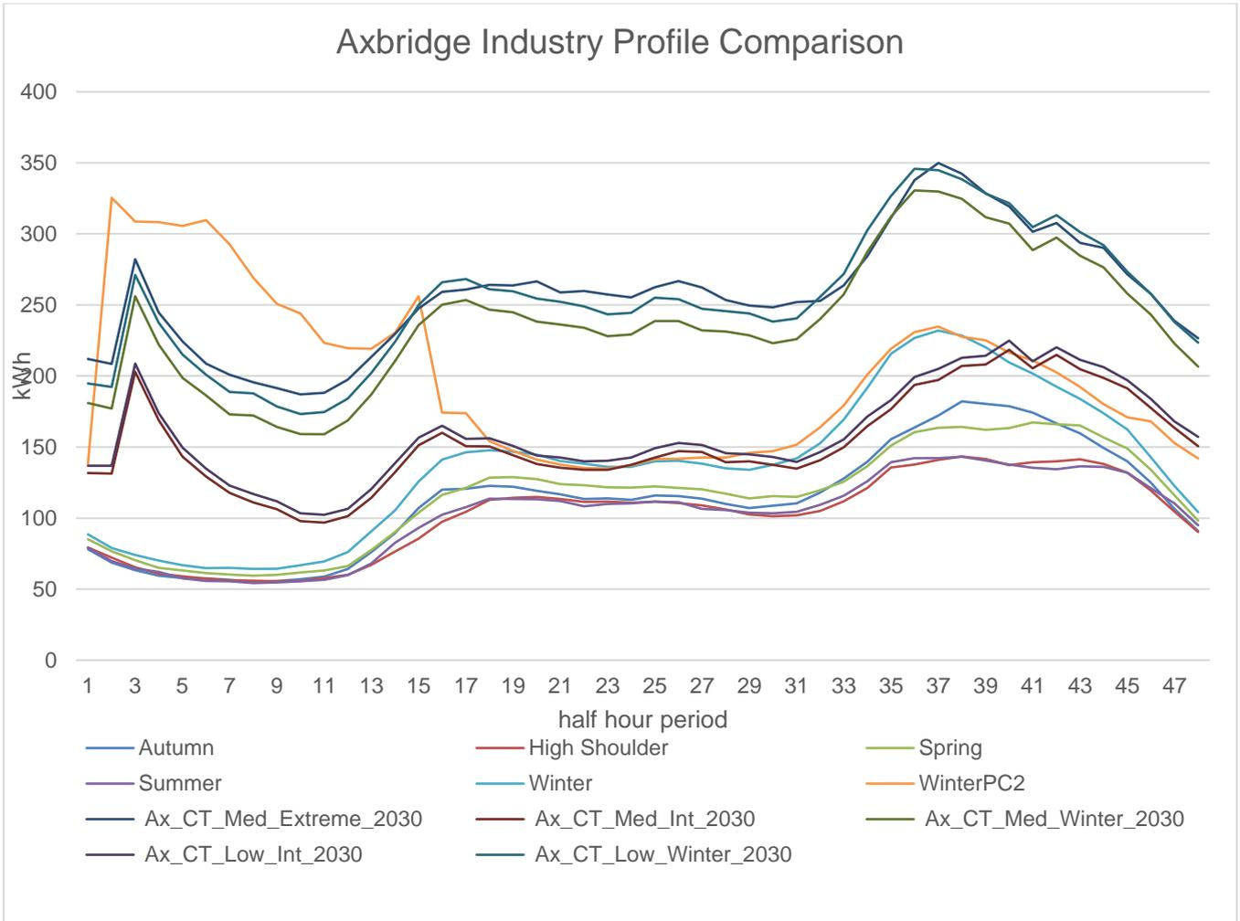
**Figure 35 Energy profiles comparing Elexon Profile Class 1 half hour by season for the whole of Axbridge (approximately 252 homes). Winter PC2 applies a Elexon Profile Class 2 (night storage heater) to all of the homes. Scenario labels are the same as above, reduced number to be able to fit on to graph.**
