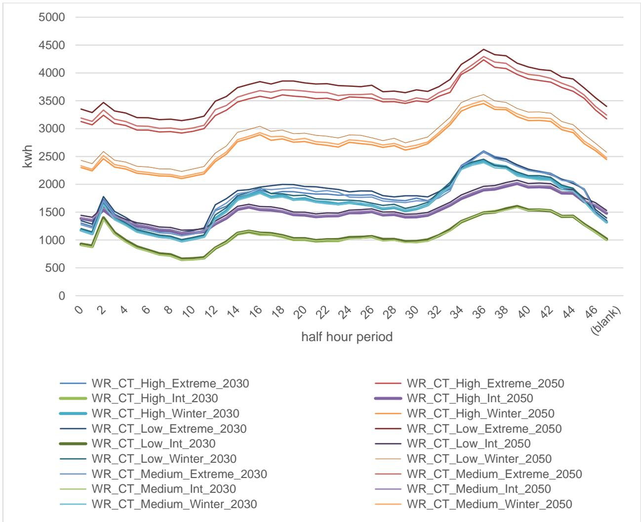
Figure 30 Energy profiles for heating simulated for the whole of WithycombeRaleigh (approximately 1,843 homes) and takeup of heat pumps using percentage offsets to the HTC random variable, results are in the expected order
