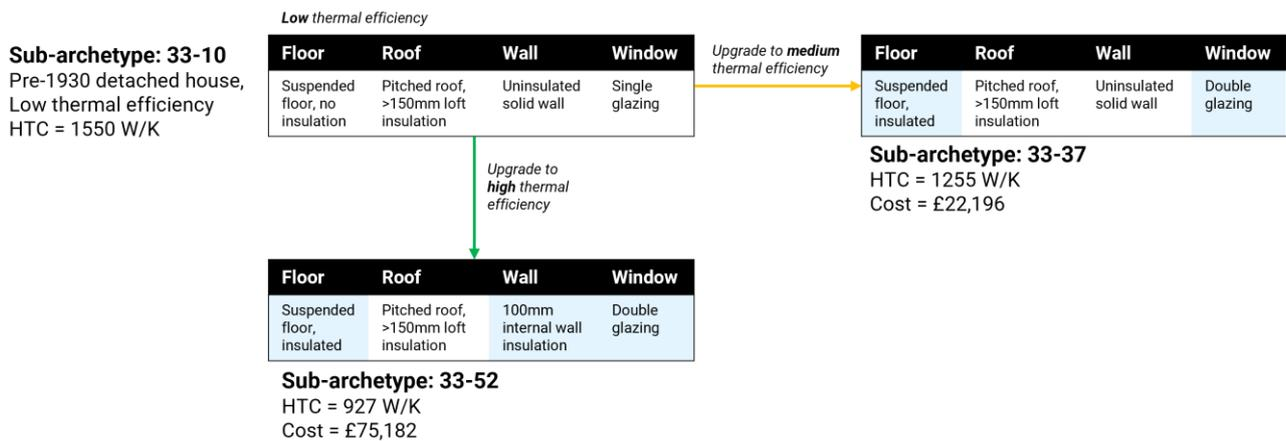
Figure 3. Diagram showing the cost optimal interventions required to move sub-archetype 33-10 (low thermal efficiency) to medium and high thermal efficiency
