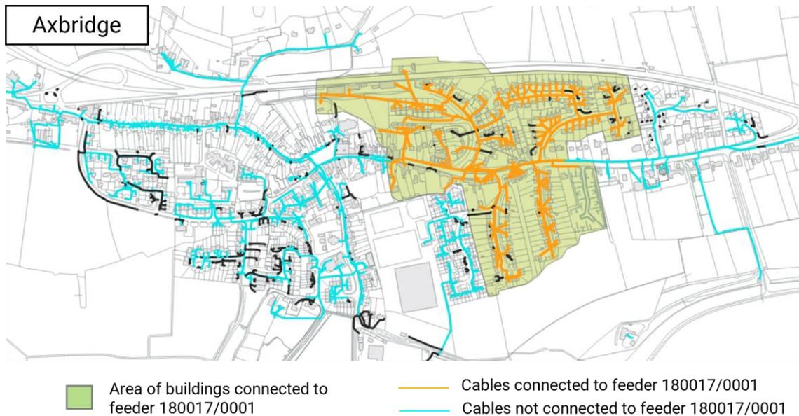
Figure 1. Image of GIS proximity analysis showing how network cable files were used to draw polygons (shown in green) to map buildings connected to feeder 180017/0001
