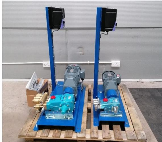
**Figure 5 Liquid carbon dioxide pumps**
