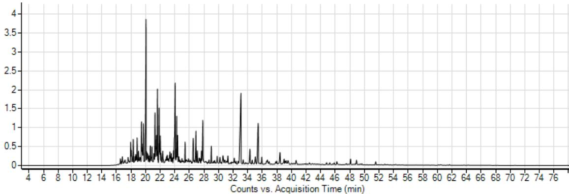
**Fig.6. Gas chromatogram of Creosote, each peak represents an individual component**
