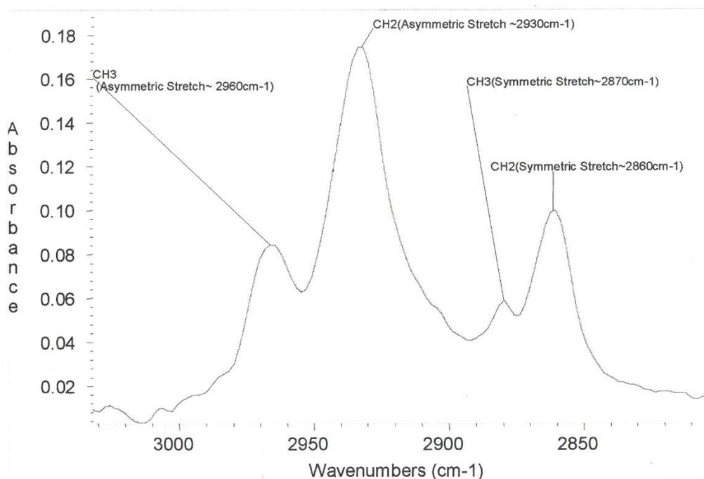
**Fig.4. Individual peaks and their associated stretching configurations**
