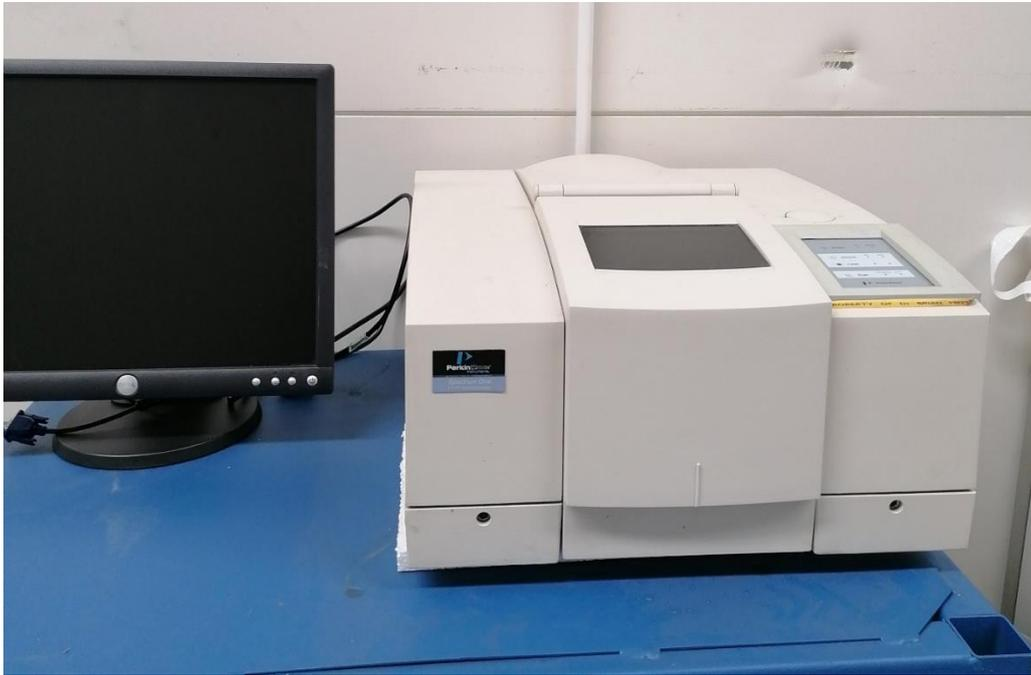
**Fig. 10 Infrared spectrometer**
