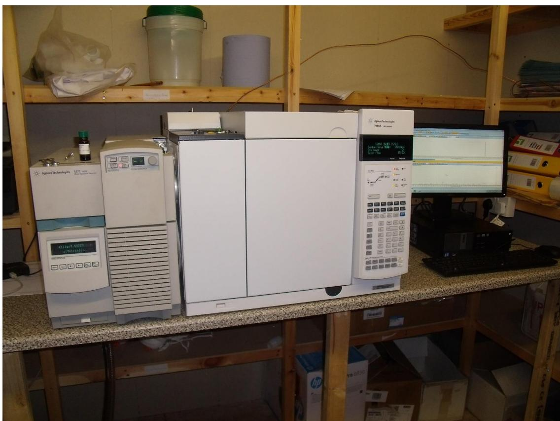
Fig.7 GC/MS system (MS on left, GC on right)
