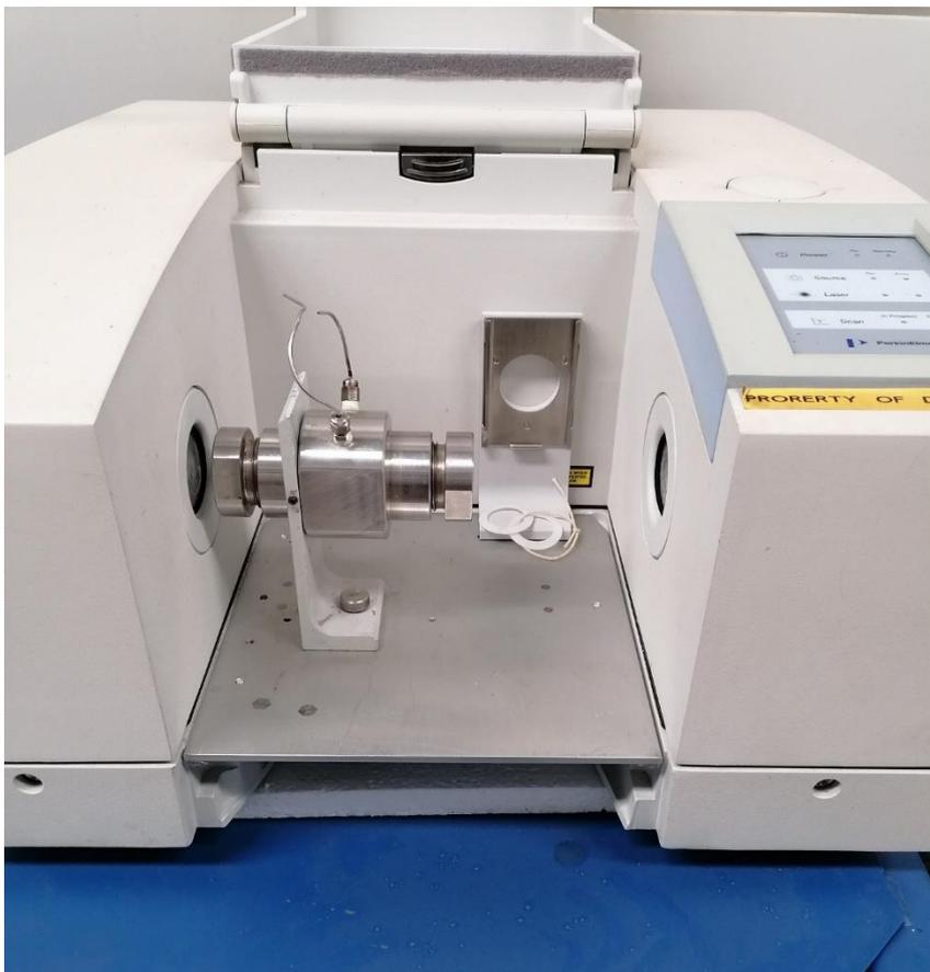
**Fig. 11 High pressure cell situated in infrared spectrometer**
