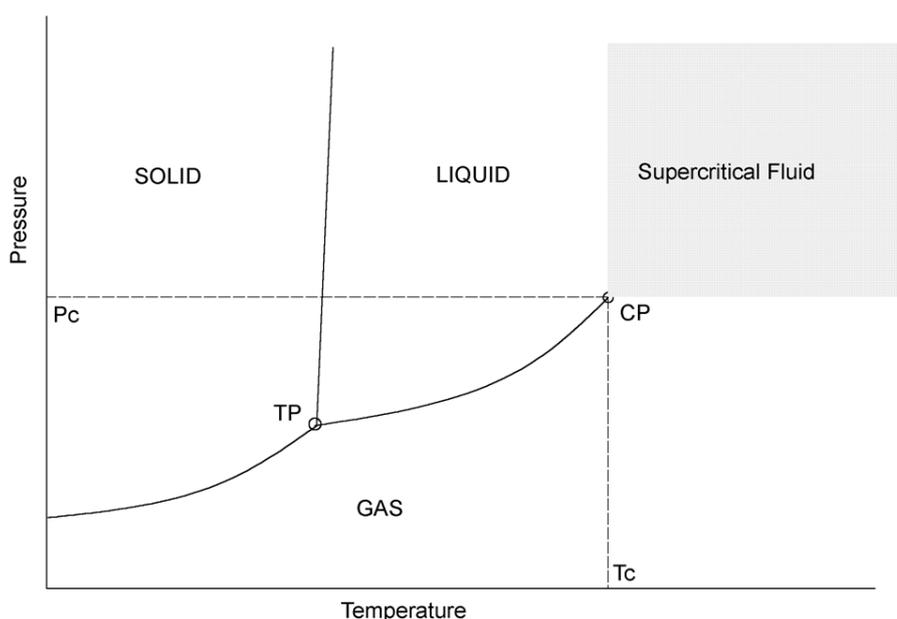
**Fig. 1. Phase diagram showing Supercritical Fluid region**
