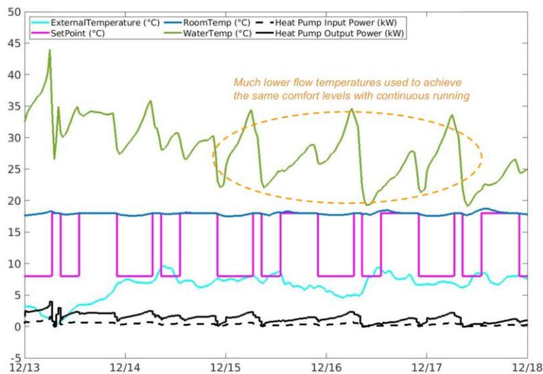
**Figure 47** shows an example simulation output for theoretically optimised controls. The flow temperature is dynamically chosen to achieve the same comfort levels at lowest running cost.
