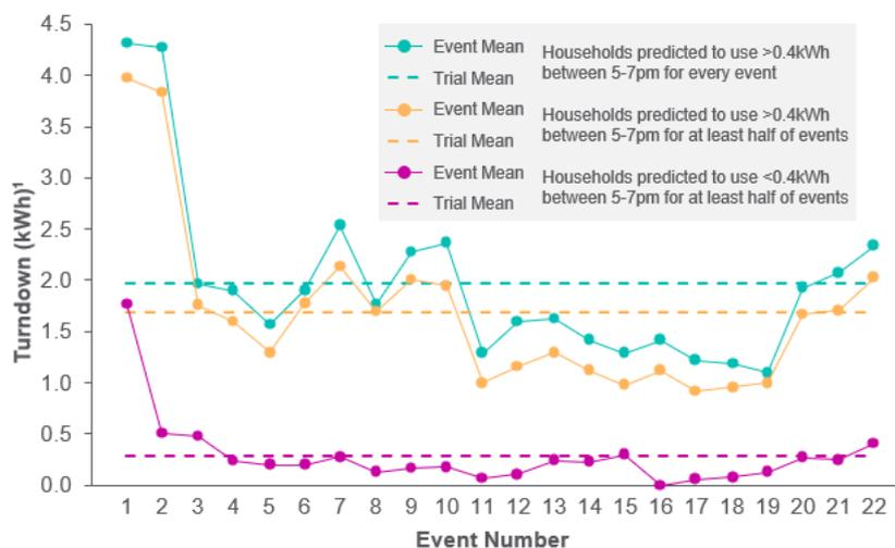
Figure 31 shows that the turndown impact of these households was measurably lower than for those who were baselined to be using grid electricity for at least half of events (0.29 kWh per household per event vs 1.68 kWh). Those baselined to use more than 0.4 kWh for all events provided an average per event turndown of 1.97 kWh.
