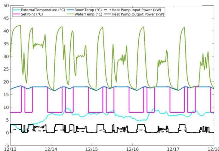
**Figure 45** shows an example simulation output for standard manufacturer controls without weather compensation. This is assumed to be an “optimum start” thermostat that pre-warms the house at maximum flow temperature.
