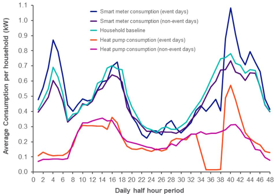
**Figure 22** shows the average per event heat pump kWh turndown. The average across the trial was 0.61 kWh per household per event.
