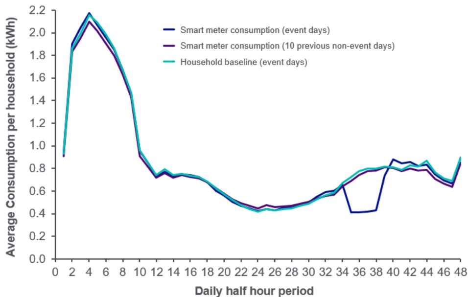
As **Figure 16** above illustrates, gradually increasing consumption between 5-7pm on non-event days was replaced with a sharp drop at 5pm and flatlining consumption to 7pm. The figure also shows that the baseline for the event days closely followed the average household consumption on recent prior non-event days, providing confidence in the turndown calculations.
