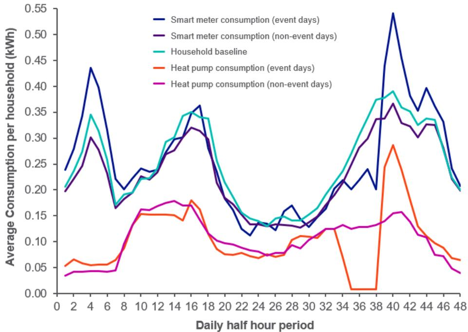
Even more stark, however, is the spike, or *snapback*, which occurs at 7pm when all households' heat pumps were automatically turned back on. Heat pump consumption in the 7-8pm window was almost double that on non-event days.
