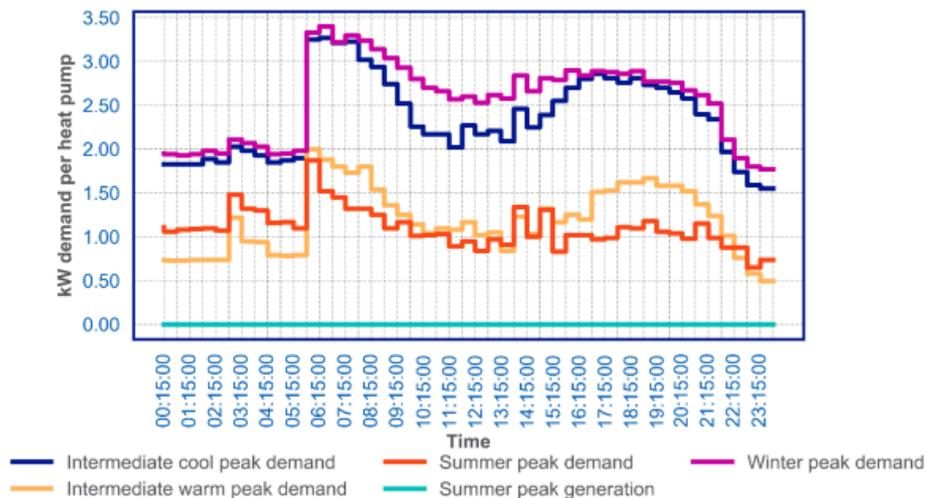
**Figure 50 – Non-hybrid heat pump profiles with thermal storage**
