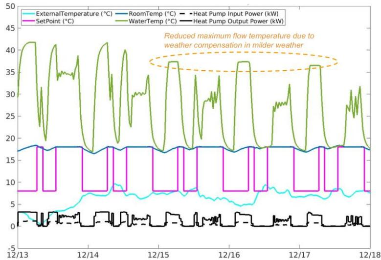
**Figure 46** shows an example simulation output for standard manufacturer controls with weather compensation. Heat pump maximum flow temperatures are limited in milder weather to improve the coefficient of performance (CoP).
