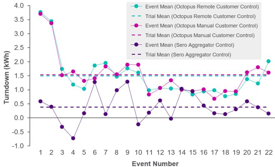
**Figure 29** also shows that there is no meaningful difference in the average household turndown provided between the remote customer control and manual customer control participants, 1.50 kWh and 1.54 kWh per participating household per event, respectively. This similarity in turndown amount can be attributed to the fact that both control types were evenly spread across the two payment types.
