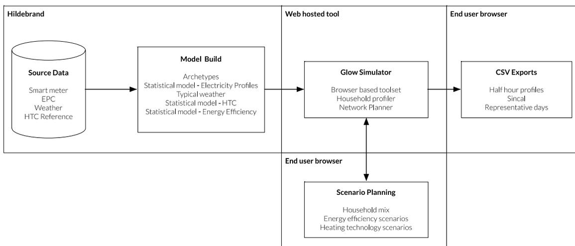
Figure 5-1. Overall system components
