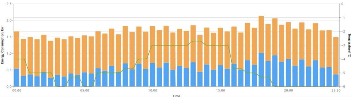
**Figure 5-6. Post-1930 mid-terrace house with flat roof and solid floor, electrical baseload plus ground source heat pump with “high” insulation**
