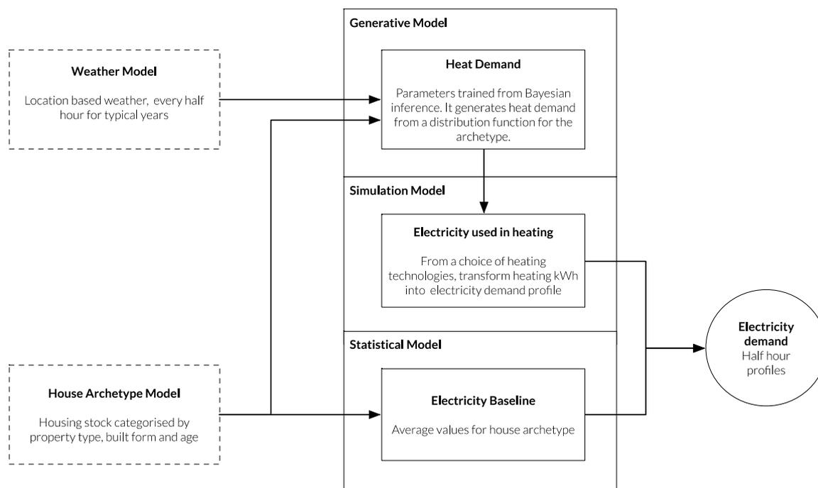
**Figure 5-2. Model elements used to generate data**
