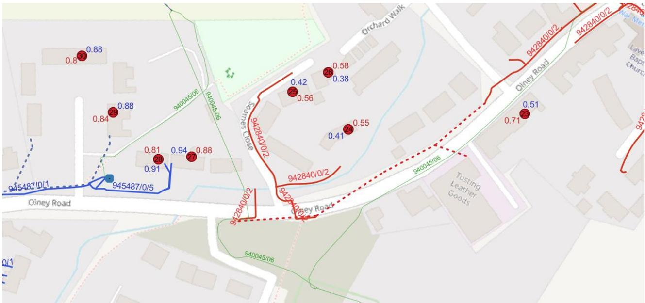
**Figure 9: Wrong MPAN assignments between two SS which are fed from the same primary feeder**
