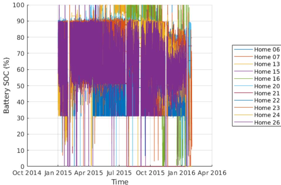
Figure 2.13 - Battery SOC across the SoLa Bristol data set for all eleven homes
