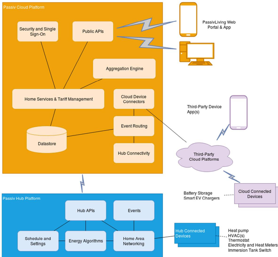
Figure 2-7: MADE system architecture
