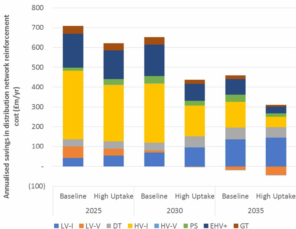
Figure 2-5 Breakdown of annualised savings in network reinforcement cost driven by MADE concept across voltage levels and asset types
