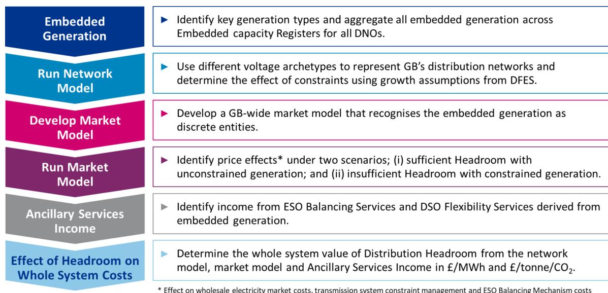
**Figure 1: High Level Process to Determine Whole System Value of Distribution Headroom**
