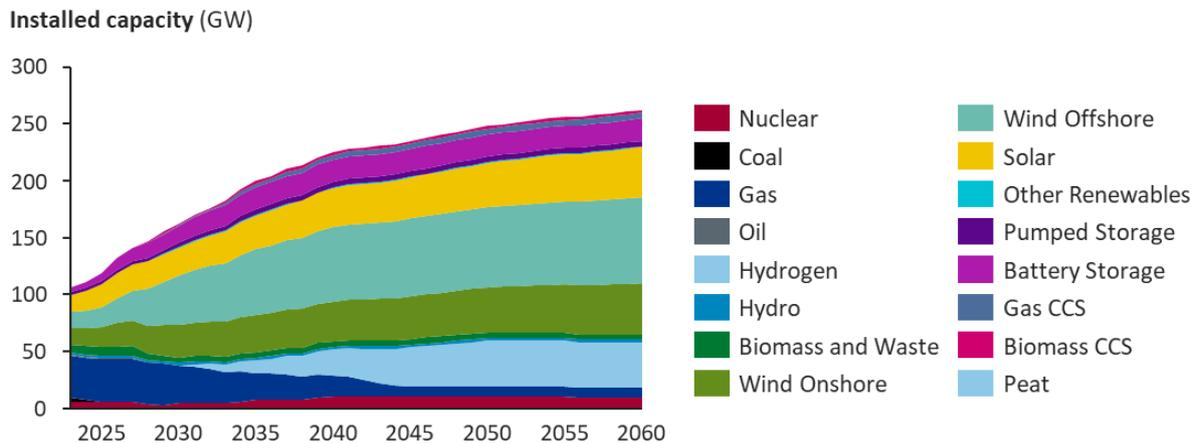
**Figure 5: Capacity assumptions, Baringa Net Zero High**
