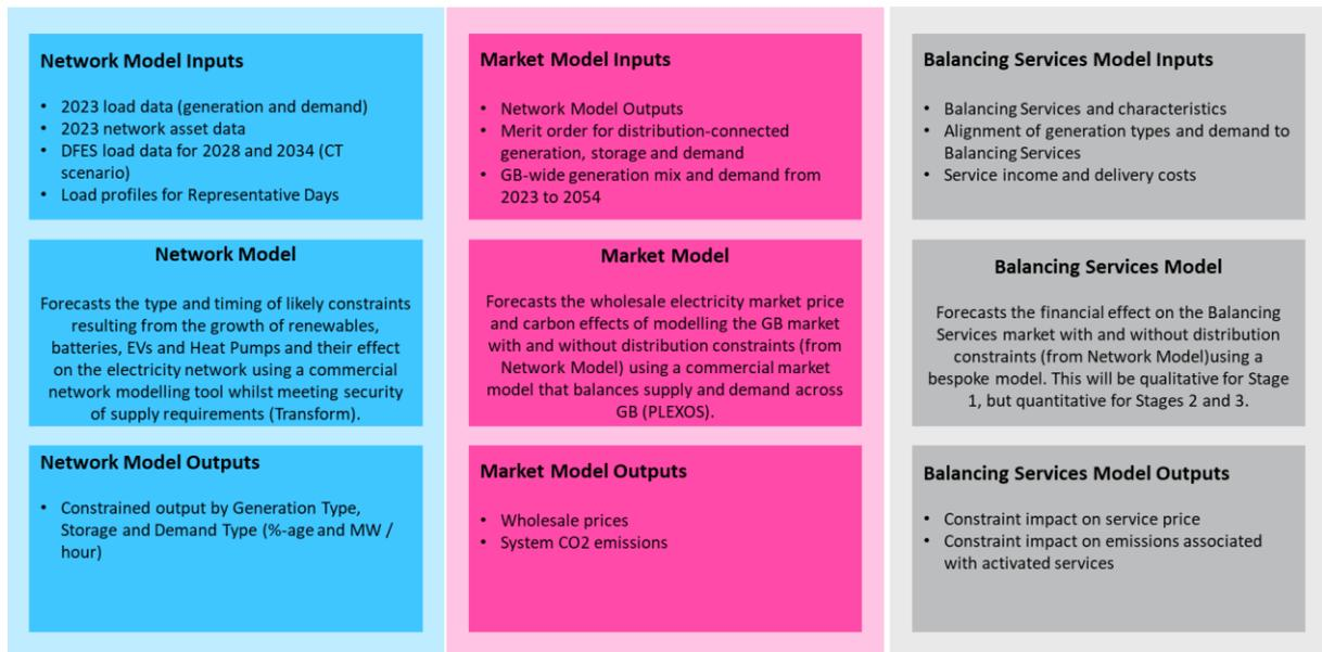
**Figure 2: Process for Determining the Whole System Value of Distribution Headroom**
