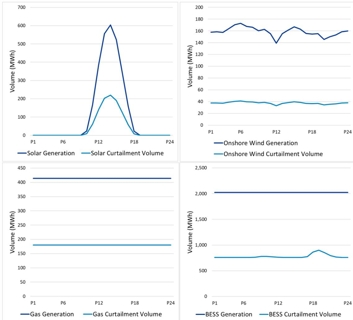
**Figure 17: January 2034 mean day, SCT aggregated curtailment and generation volume dataset**
