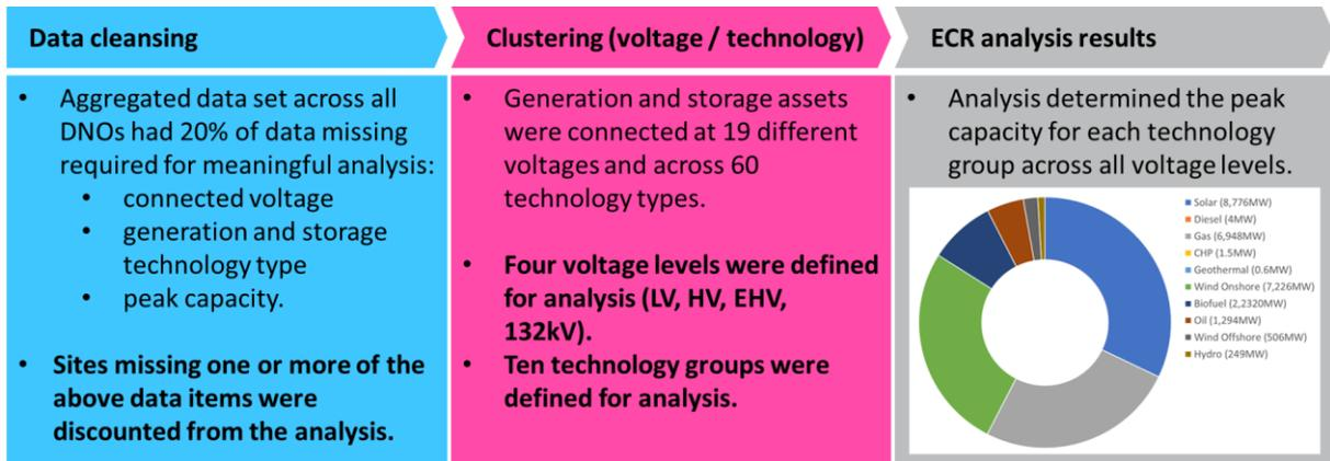
Figure 10: Process for analysis of ECRs
