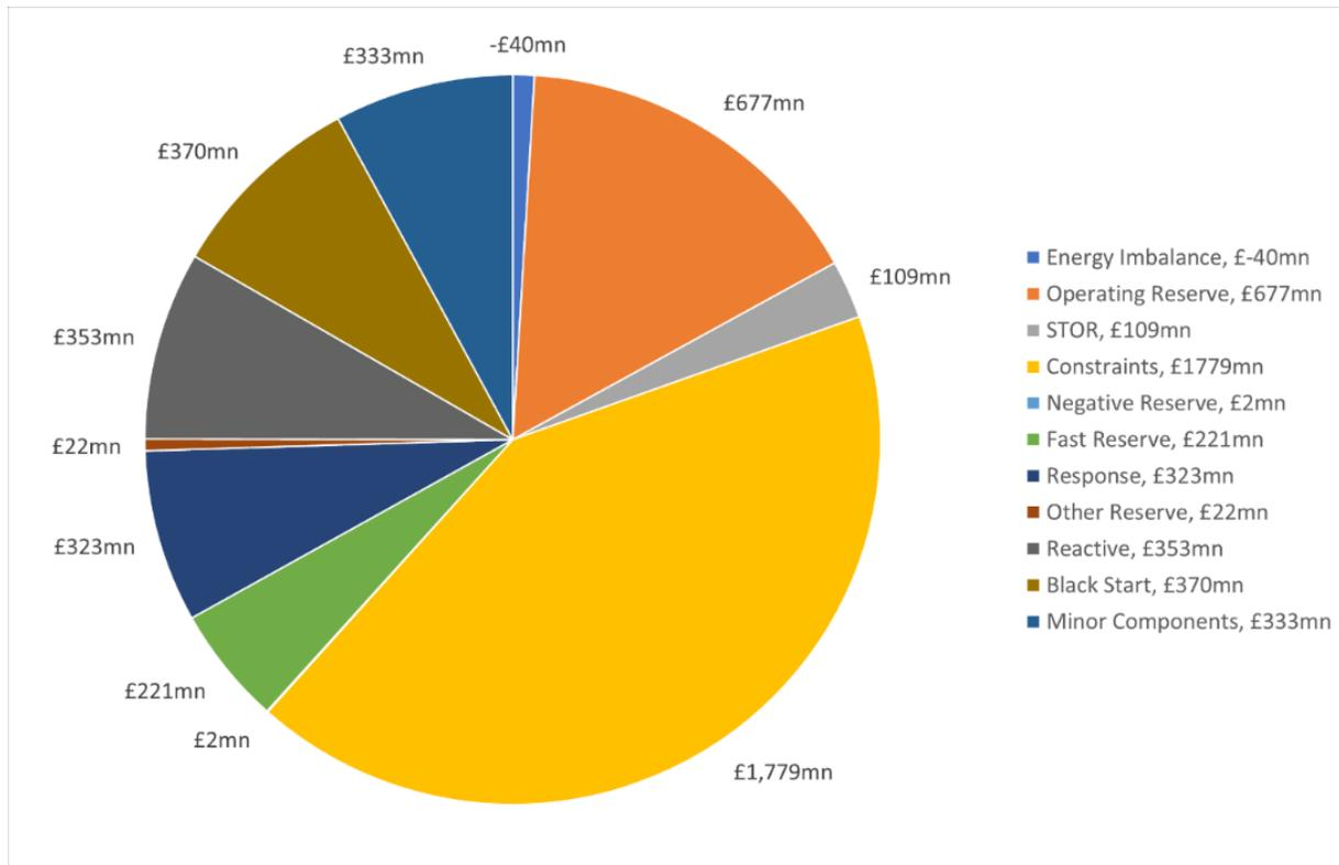
**Figure 33 NGESO Balancing Services breakdown 2022/23<sup>22</sup>**
