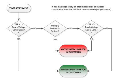
The safety limit for touch voltages shall be determined in accordance with Standard Technique TP21AA and the 'design' HV or EHV fault clearance time.
