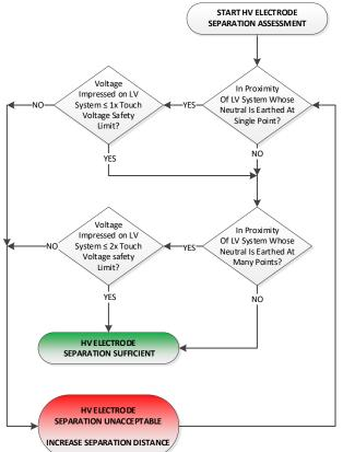
The HV electrode shall be separated from NGED, IDNO or Customer LV systems<sup>22</sup> by sufficient distance such that the voltage impressed on the LV system in the event of either a HV or source substation fault is not greater than:
