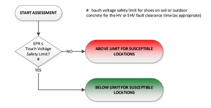
The safety limit for touch voltages shall be determined in accordance with Standard Technique TP21AA and the 'design' HV or EHV fault clearance time for shoes on soil or outdoor concrete (or other surface as appropriate).
