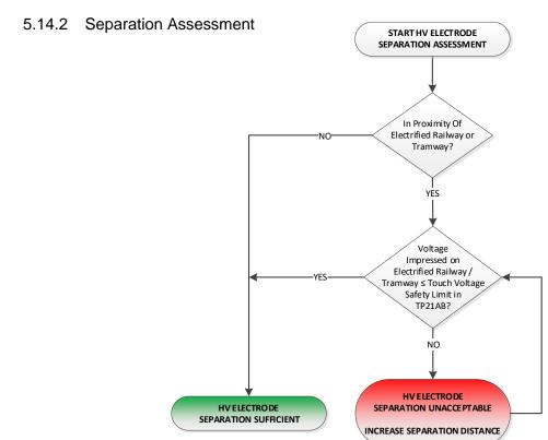
The HV electrode shall be separated from electrified railways & tramways by sufficient distance such that the voltage impressed on those installations in the event of either a HV or source substation fault is not greater than the touch voltage limit specified in TP21AB for the fault clearance time of the distribution substation or source substation (as appropriate).
