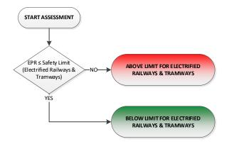
The safety limit for touch voltages shall be determined in accordance with Standard Technique TP21AB and the 'design' HV or EHV fault clearance time.
