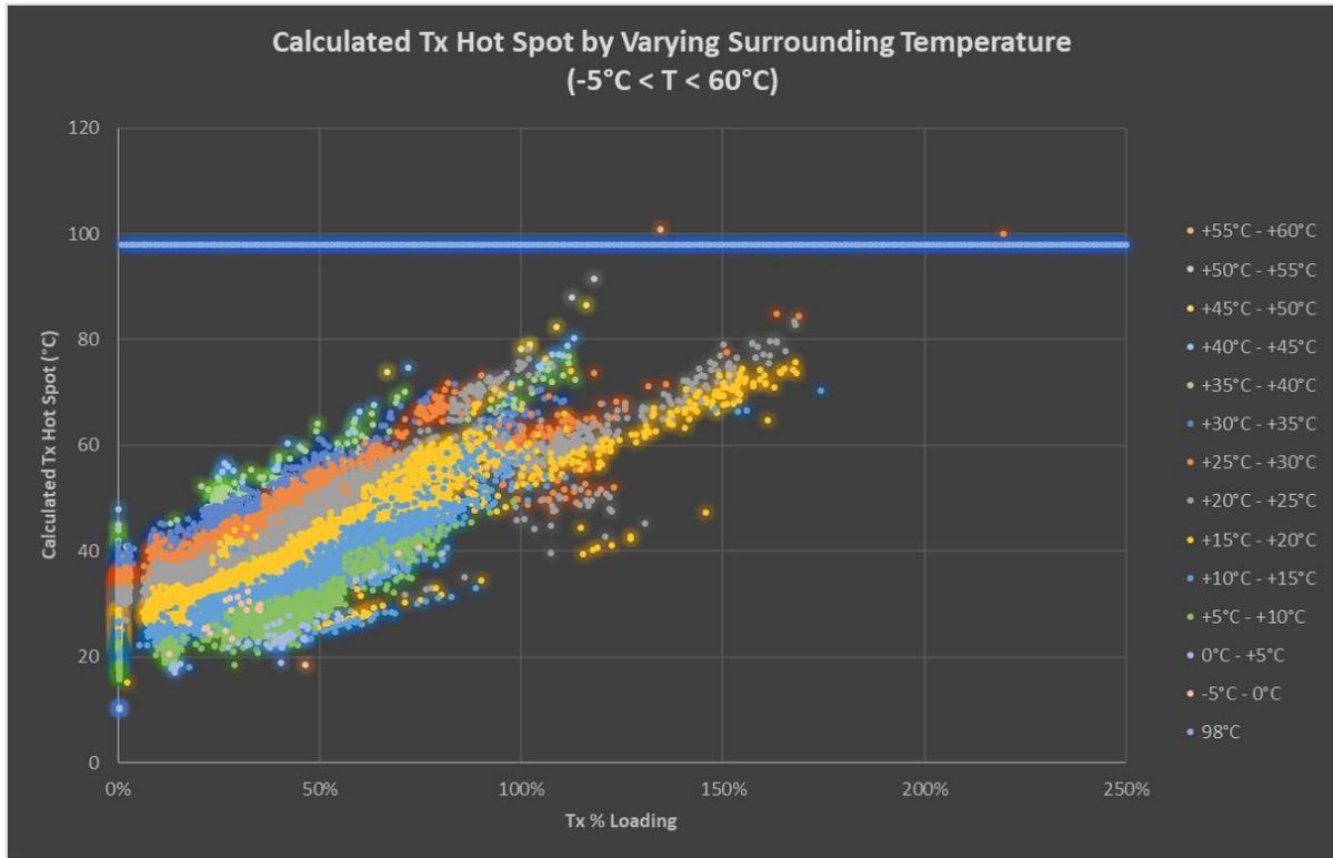
Figure 29: Calculated Tx Hot Spot by Surrounding Temperature (-5°C < T < 60°C)
