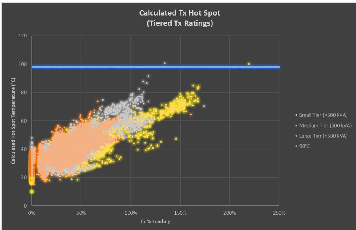
**Figure 22: Calculated Tx Hot Spots by % Loading**
