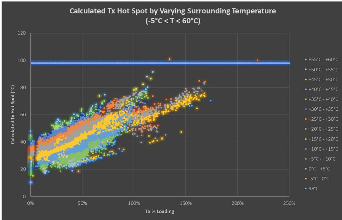
**Figure 18: Calculated Tx Hot Spot in relation to surrounding temperature**
