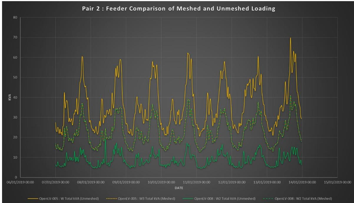
**Figure 20: Pair 2 – Feeder Comparison – Meshed & Unmeshed Loading**
