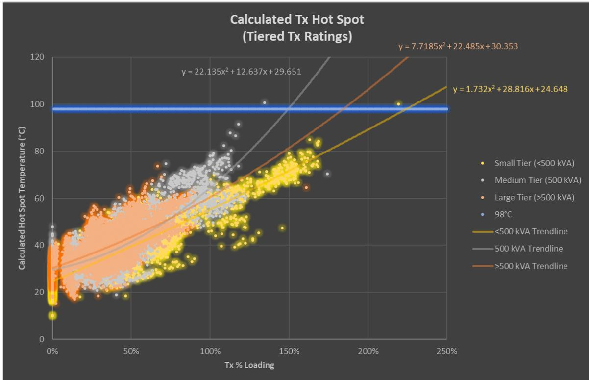
**Figure 17: Forecasting Tx Hot Spot Temperatures**
