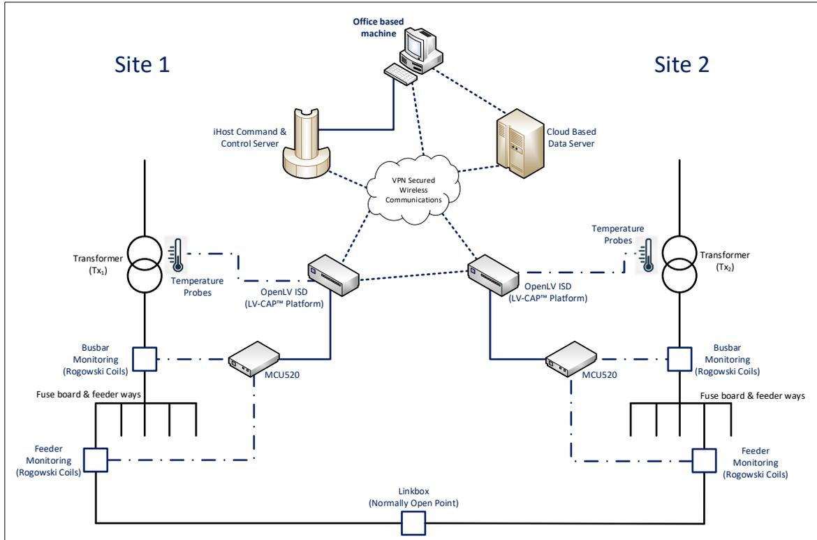
**Figure 4: LV network arrangement and LV-CAP deployment**
