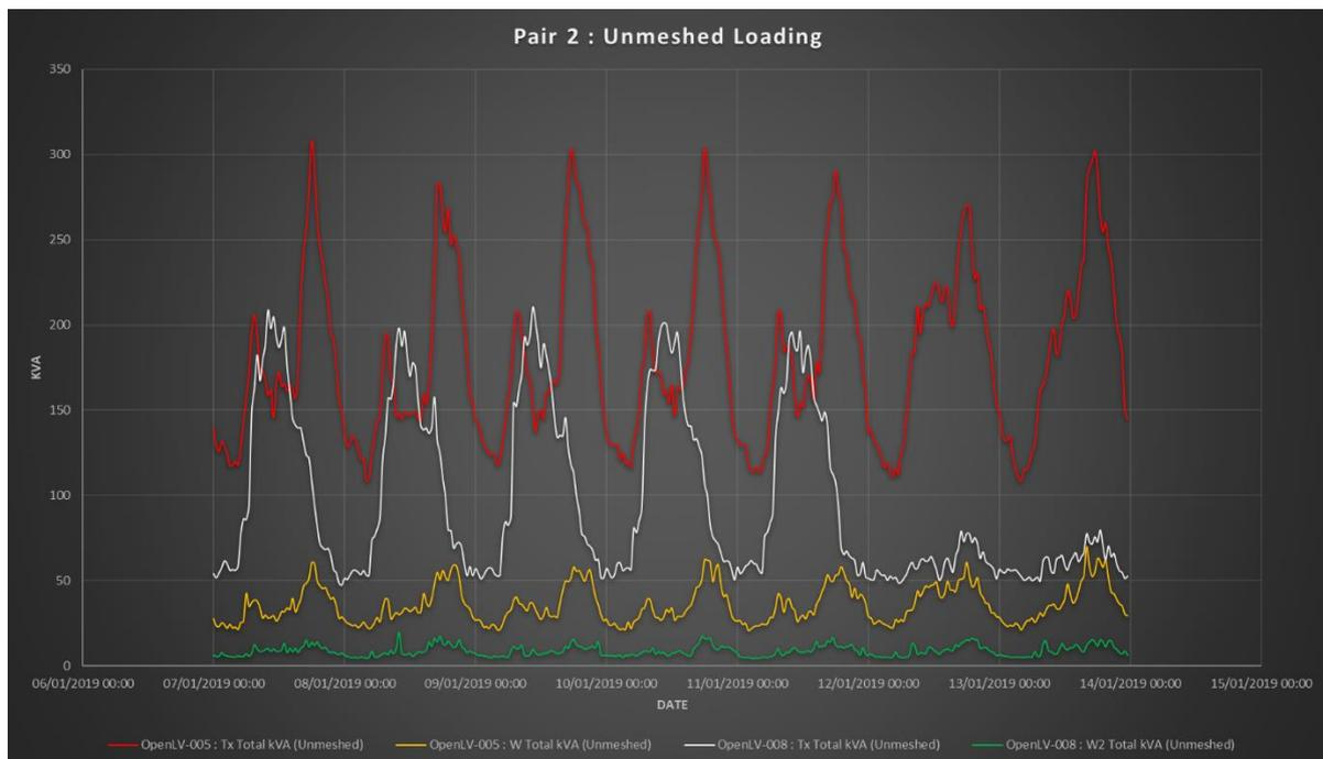
**Figure 19: Pair 2 - Unmeshed Loading**
