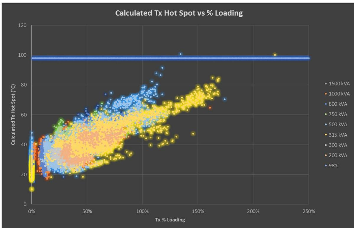
**Figure 26: Calculated Hot Spot vs % Loading**
