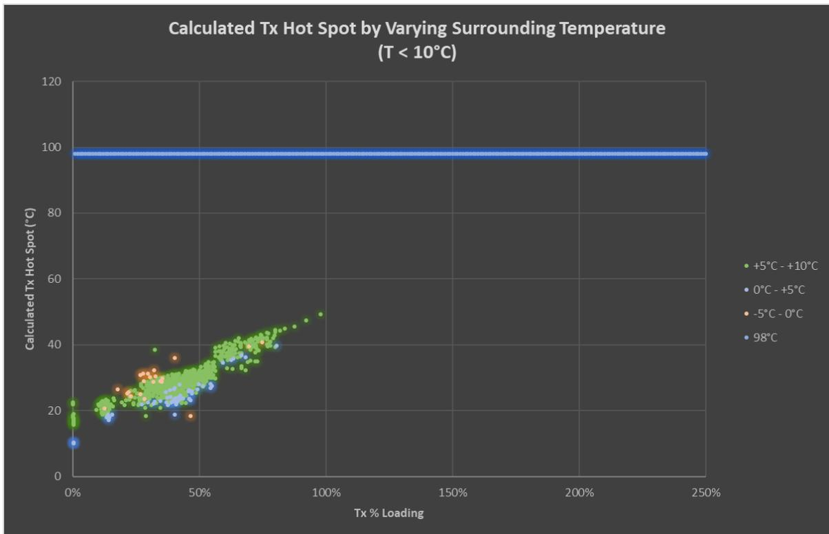
**Figure 35: Calculated Tx Hot Spot by Surrounding Temperature (T < 10°C)**
