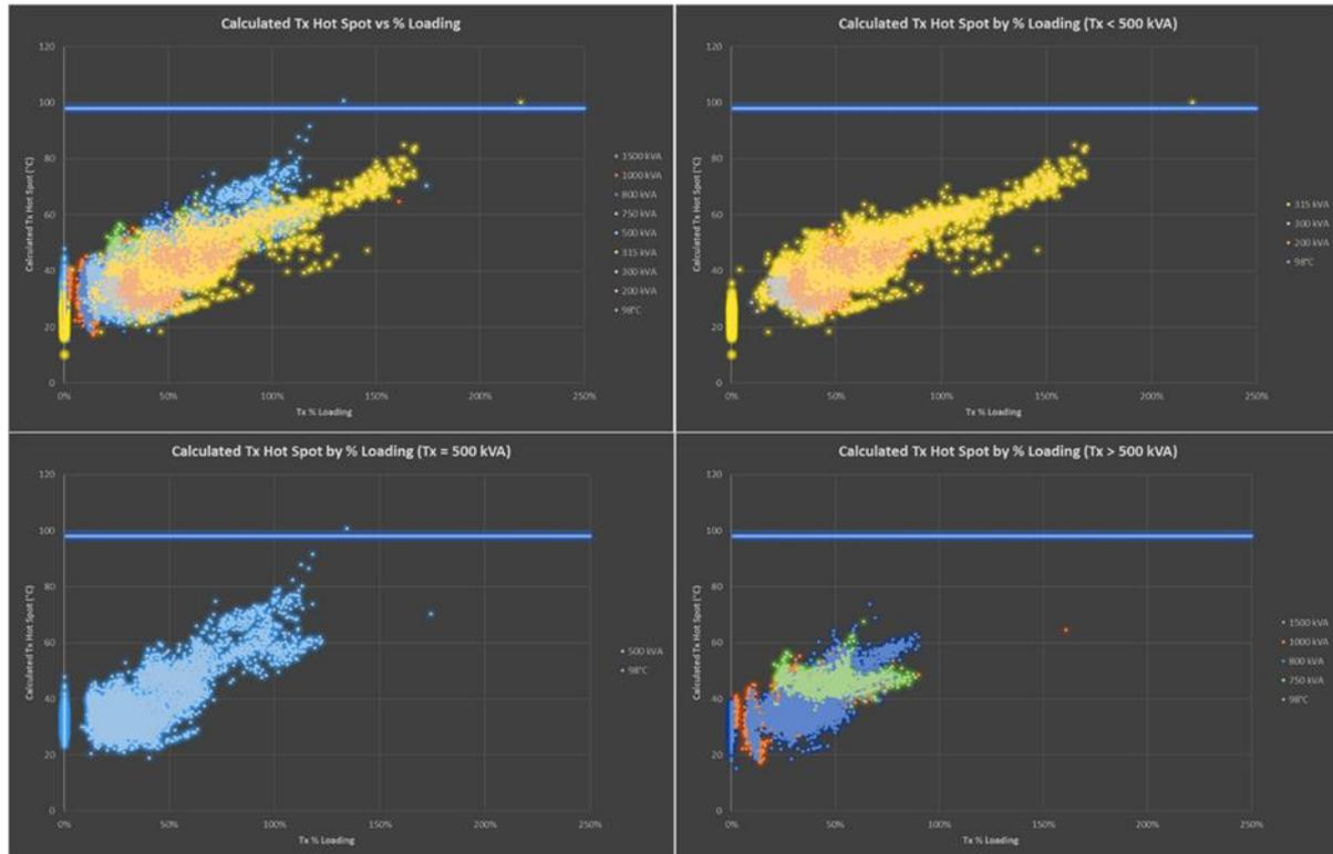
**Figure 16: Calculated Hot Spot vs % Loading (Tx Groupings)**
