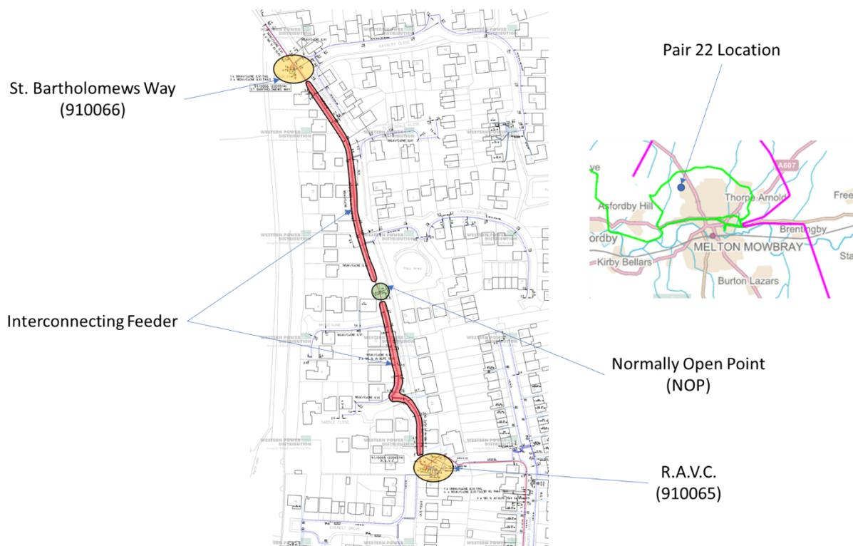
**Figure 6: Pair 22 - Location and Network Layout Details**
