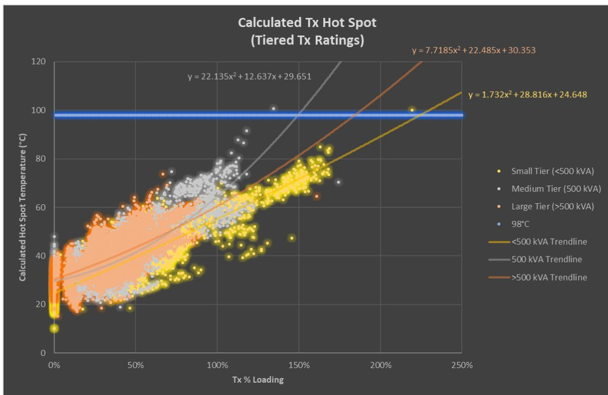
**Figure 28: Forecasting Tx Hot Spot Temperatures**
