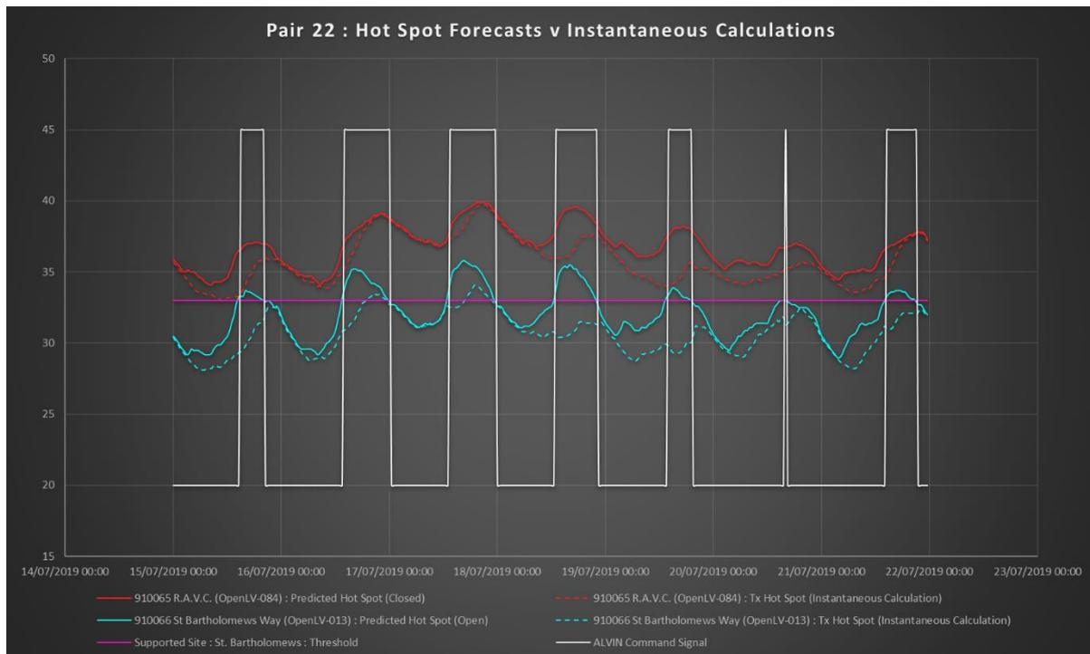
**Figure 12: Pair 22 - Effect of Switching on Tx Temperatures**
