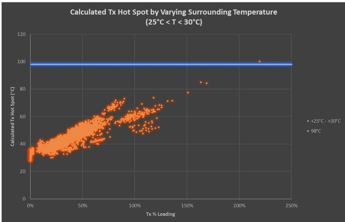
**Figure 31: Calculated Tx Hot Spot by Surrounding Temperature (25°C < T < 30°C)**
