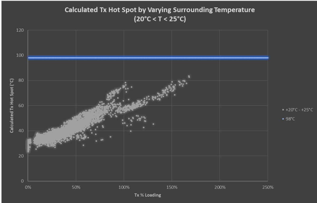
**Figure 32: Calculated Tx Hot Spot by Surrounding Temperature (20°C < T < 25°C)**
