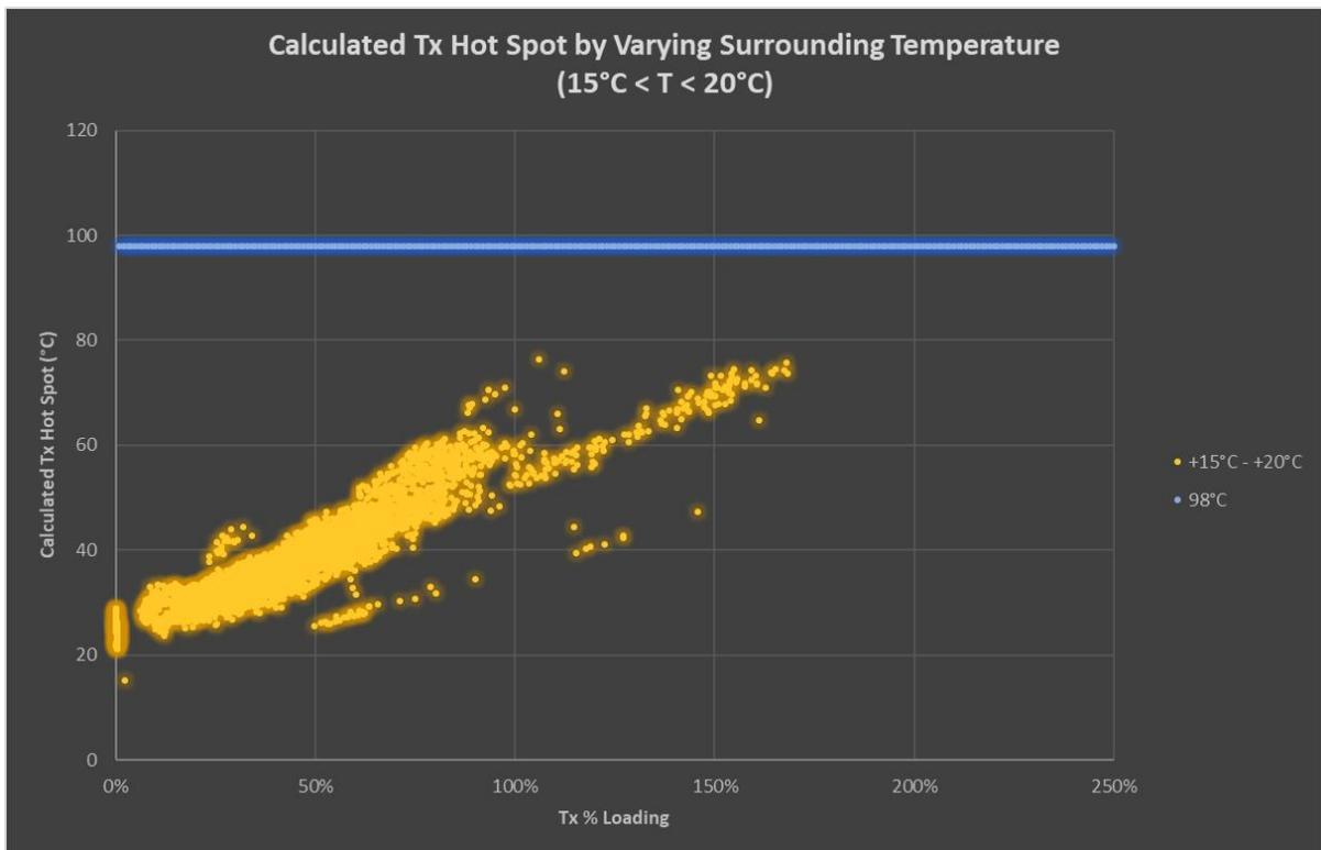
**Figure 33: Calculated Tx Hot Spot by Surrounding Temperature (15°C < T < 20°C)**
