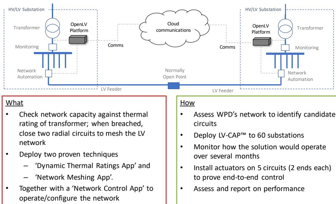
**Figure 1: Method 1 – Network Capacity Uplift**
