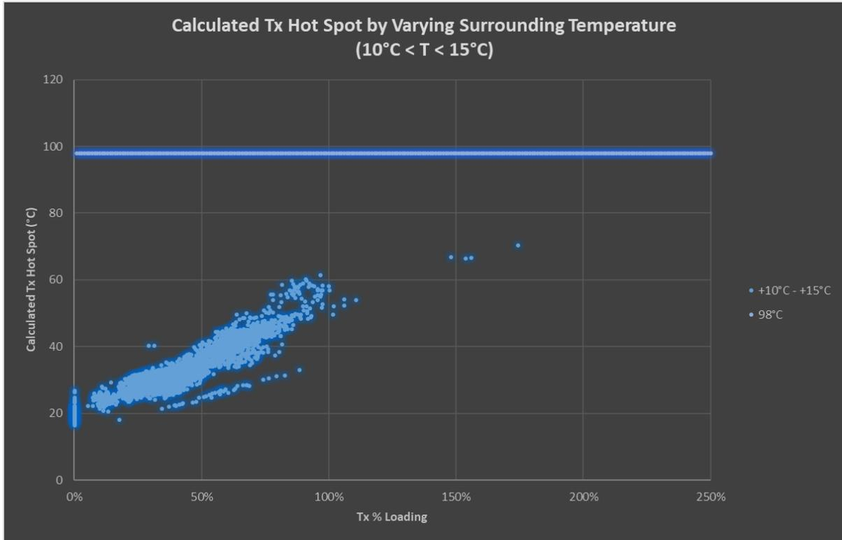
**Figure 34: Calculated Tx Hot Spot by Surrounding Temperature (10°C < T < 15°C)**
