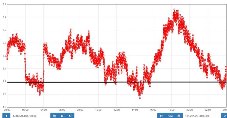
Fig 2. Plot showing subsea cable loading over an average day (red) and where a +2.2MW limit would have triggered system operation.
