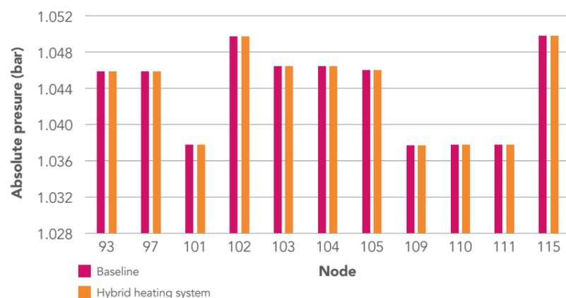
Figure 42: Pressure profile for LP#2 at 07:00 (peak) for different scenarios
