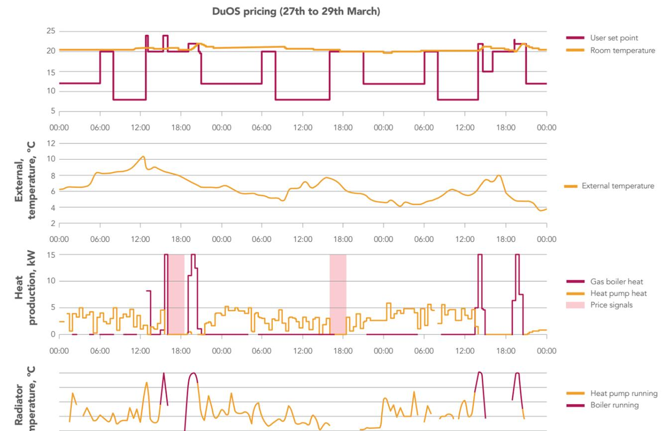
Figure 17: Case study showing time-series of a hybrid heating system, optimised for LPG (GCR=0.49), but with two periods of DuOS pricing applied
