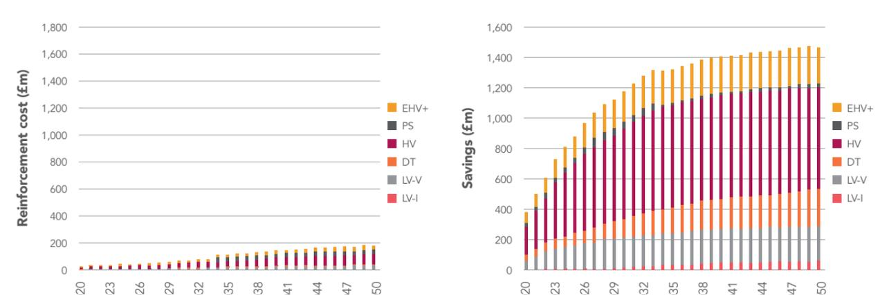
Figure 32: Development of South Wales' electricity distribution network upgrade cost for PassivSystems smart control of hybrids scenario
