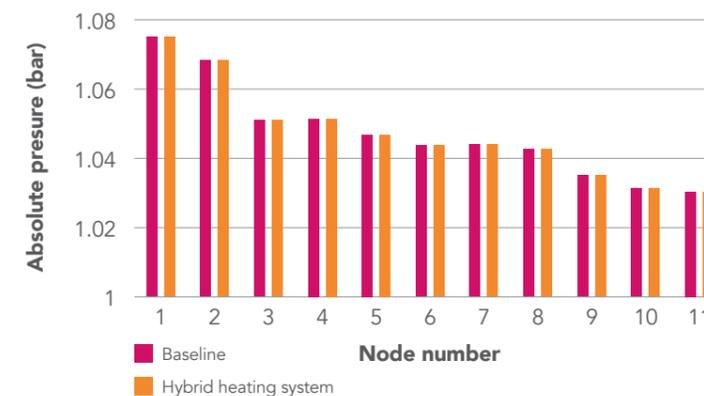
Figure 40: Pressure profile for LP#1 at 08:00 (peak) for different scenarios
