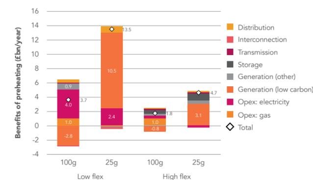
Figure 52: The benefits of high preheating in a low flexible and high flexible system
