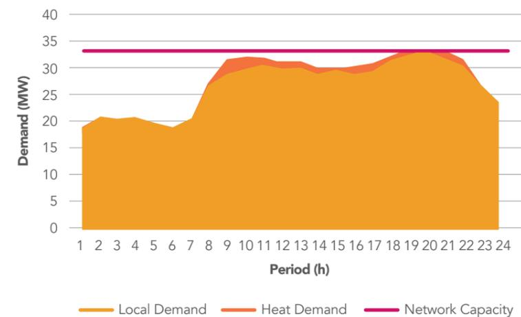
Figure 67: Local and electrified heat demand at the distribution network (a) without and (b) with network support service
