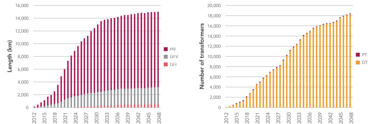
Figure 24: Development of South Wales's electricity distribution network upgrade (left) network length and (right) number of transformers for ASHP scenario; LV – low voltage network, DT – distribution transformer, HV – high voltage network, PT – primary transformer, I – thermal driven reinforcement, V – voltage driven reinforcement
