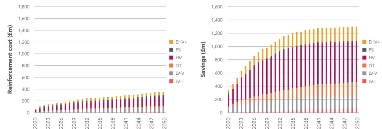
Figure 28: Development of South Wales's electricity distribution network upgrade cost for hybrid heating-only scenario
