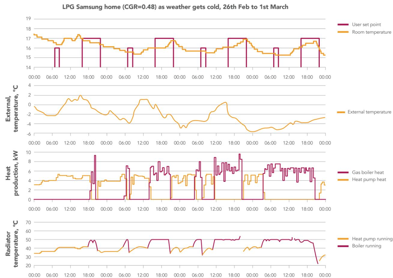
Figure 16: Case study showing time-series of a hybrid heating system with LPG, configured with a very high gas cost ratio matching real pricing in cold weather
