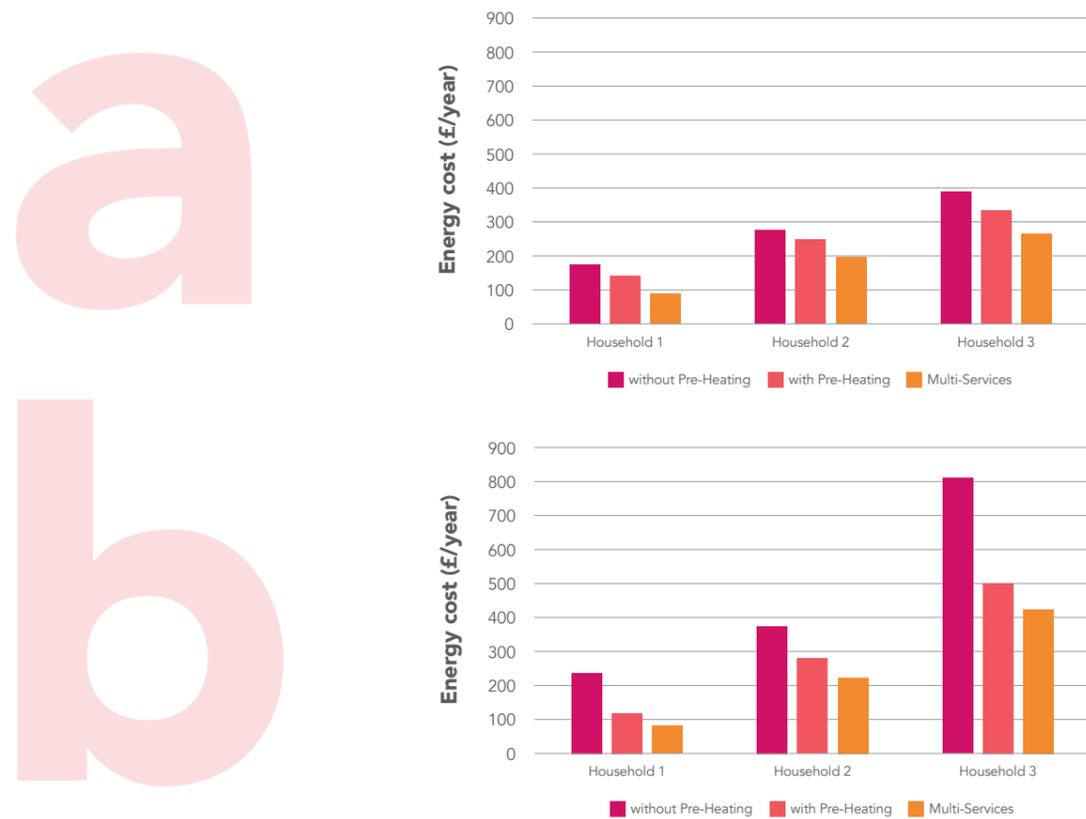
Figure 56: Energy costs when considering the provision of Multi-services (i.e. Pre-heating + Capacity + Balancing), considering different carbon targets for the energy sector (a) 100g CO<sub>2</sub>/kWh, and (b) 25g CO<sub>2</sub>/kWh. Households 1-3 increase from low to high heat demand
