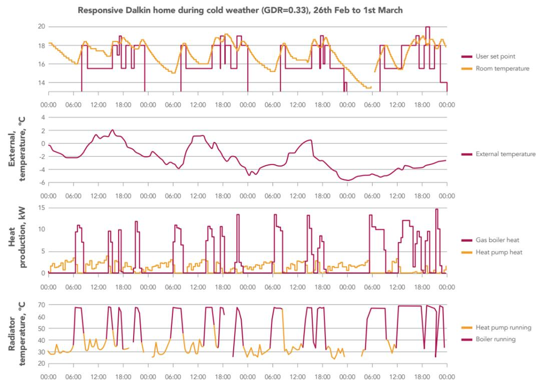
Figure 12: Case study showing time-series of a hybrid heating system during cold weather, on a high gas cost ratio
