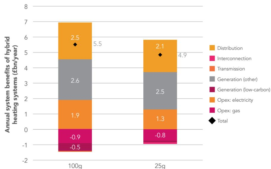
Figure 47: System-level benefits of responsive hybrid heating systems in a system with demand flexibility and storage
