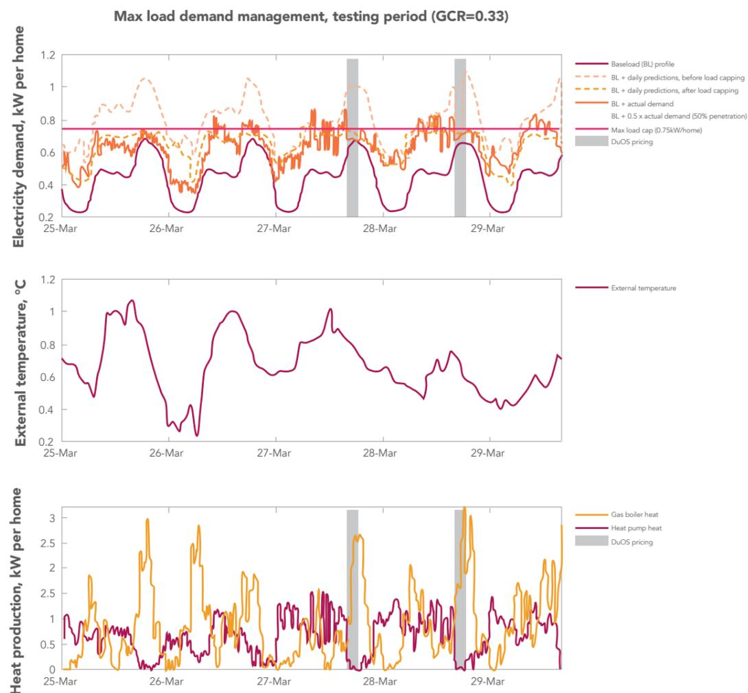
Figure 8: Aggregate electricity and heat demand over time during max load demand management operation, in a high gas price (GCR=0.33) scenario, involving 54 homes on average
