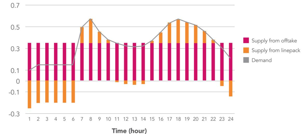
Figure 36: Gas supply and demand for the hybrid heating systems case
