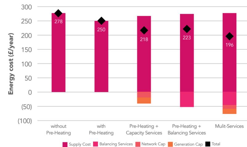
Figure 57: Energy costs when considering: Pre-heating strategies, Pre-heating + Capacity services, Pre-heating + Balancing services and Pre-heating + Capacity + Balancing services (i.e. Multi-service provision)
