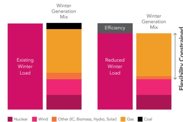
Figure 63: Illustration of generation sources responding to reduced demand from efficiency measures
