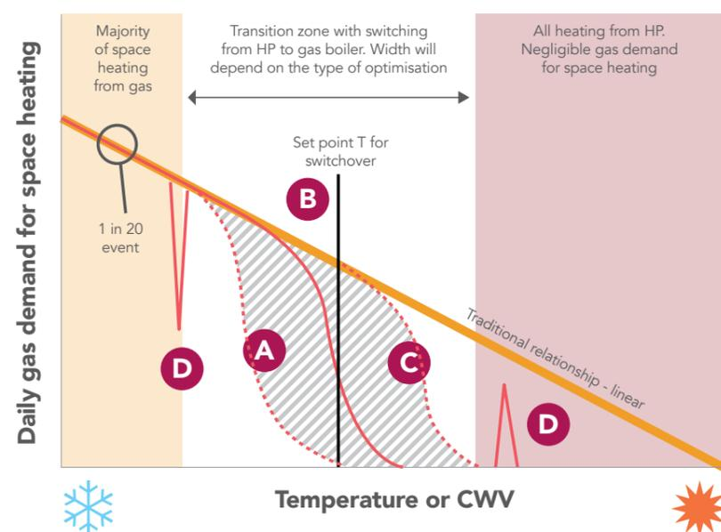
Figure 77: Hybrid heating system impact on gas demand
