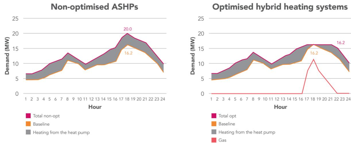
Figure 22: Non-optimised vs. PassivSystems' optimised hybrid heating system profiles
