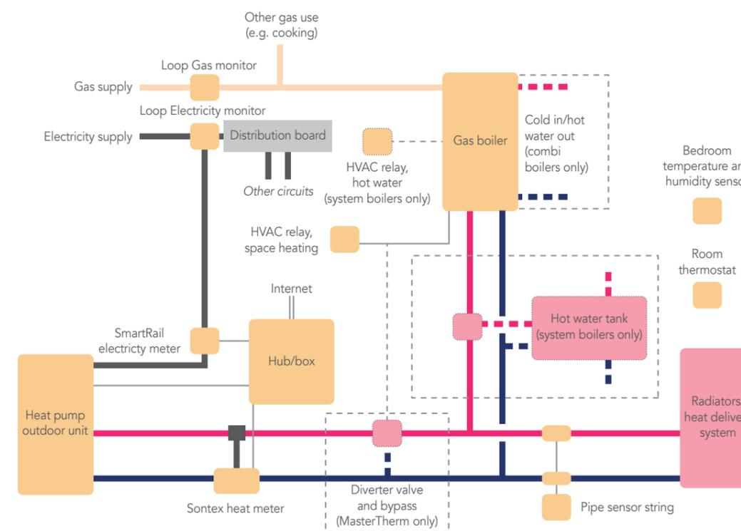
Figure 6: Schematic diagram of physical equipment deployed in a Freedom installation. Note that the Daikin configuration is different as the boiler and heat pump have a 'series' plumbing arrangement within the integrated unit
