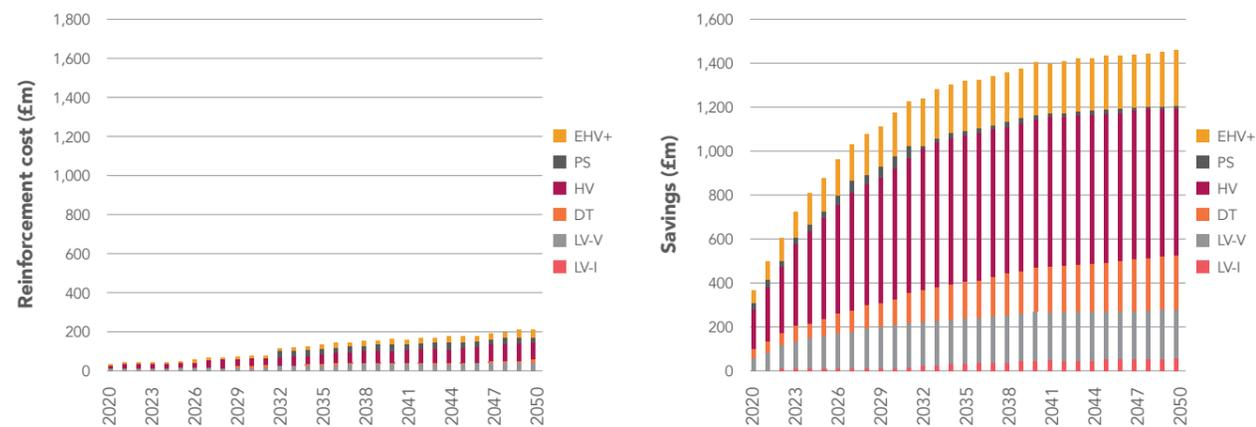
Figure 30: Development of South Wales' electricity distribution network upgrade cost for hybrid heating DUoS Tariff scenario
