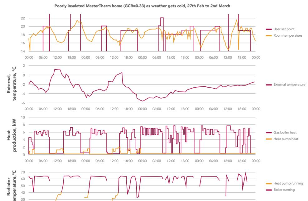
Figure 13: Case study showing time-series of a hybrid heating system during cold weather, on a high gas cost ratio, in a home that struggles to heat, presumably due to poor insulation or similar
