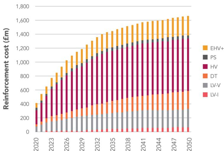
Figure 26: Development of South Wales' electricity distribution network upgrade cost for ASHP scenario; LV – low voltage network, DT – distribution transformer, HV – high voltage network, PS – primary substation, EHV+ - Extra high voltage network, bulk transformers and 132 kV network, I – thermal driven reinforcement, V – voltage driven reinforcement
