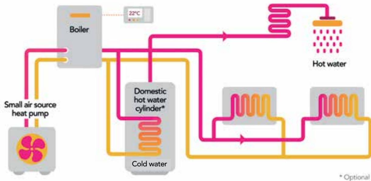
Figure 1: The hybrid heating system
