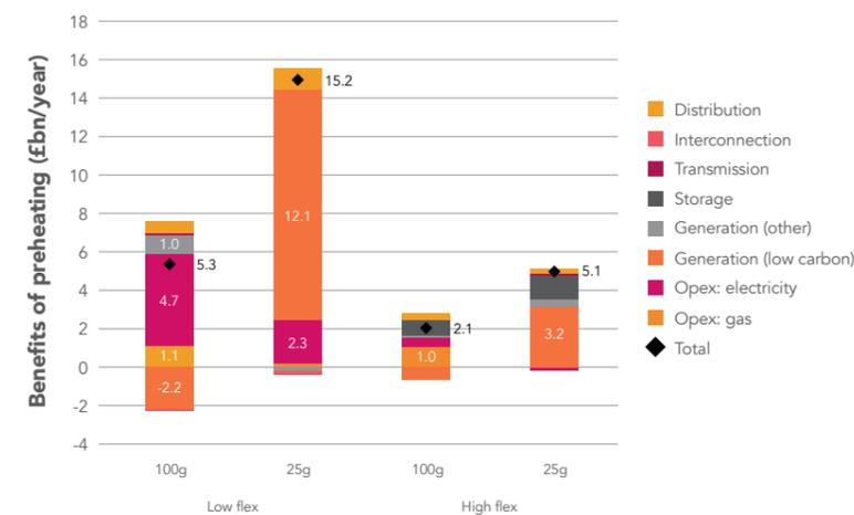
Figure 54: Benefits of PassivSystems' smart hybrid heating system control
