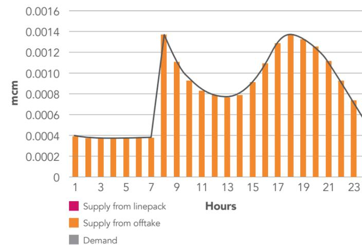
Figure 39: Gas supply and demand in the presence of hybrid heating systems
