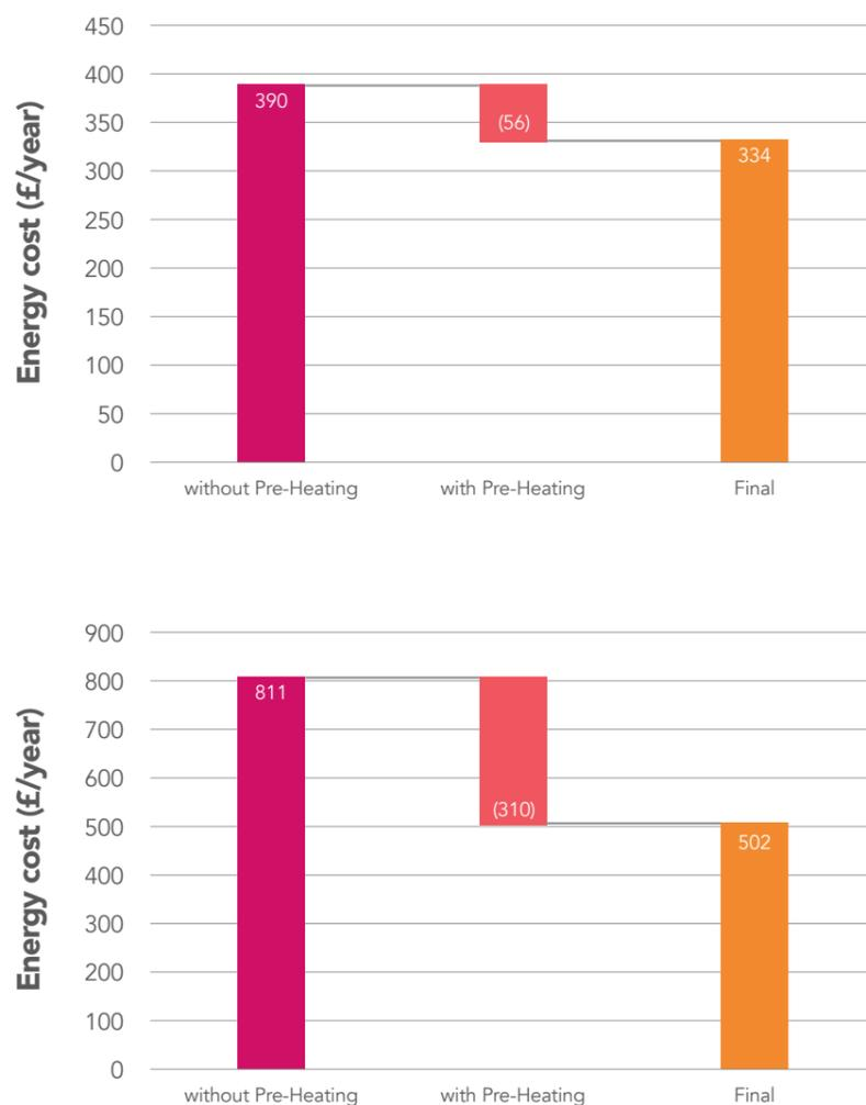
Figure 55: Energy costs for a single household with and without pre-heating strategies, and considering the carbon targets of (a) 100g CO<sub>2</sub>/kWh, and (b) 25g CO<sub>2</sub>/kWh, for the electricity sector.
