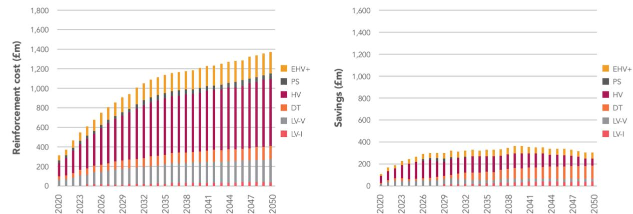
Figure 27: Development of South Wales's electricity distribution network upgrade cost for ASHP and hybrid heating scenario.
