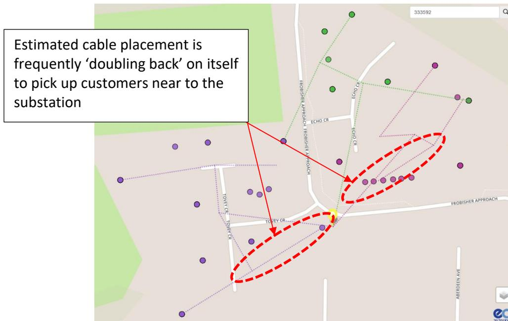
Figure 18: Line and load estimation based on absent network data illustrating the original issue
