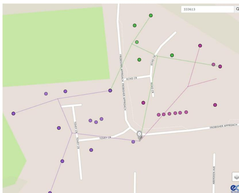
Figure 19: Line and load estimation with the corrected implementation and no 'doubling back' effect
