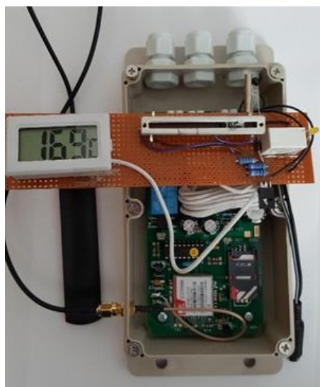
Figure 105: temperature alarm with GSM text message warnings. The LCD display is a self-contained unit used for testing.
