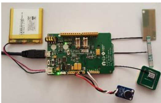
Figure 149: LinkitOne PCB front side with Battery, Wi-Fi, GPRS, GSM antennae and microphone.
