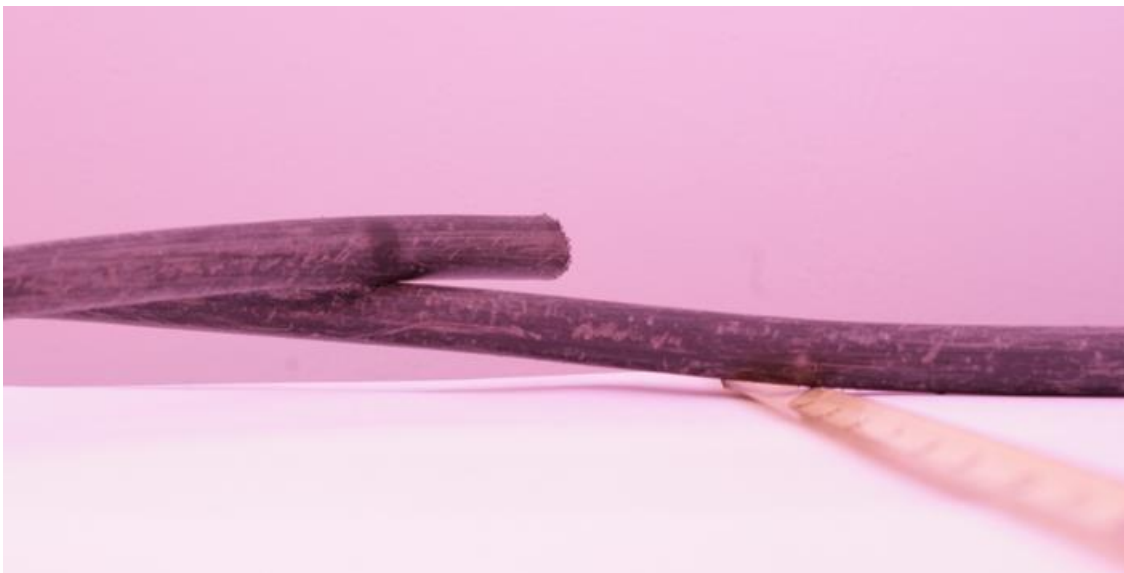
Figure 110: Infra-red image of Steel wire armoured cables (SWA) at 60°C (top) and 20°C (bottom).
