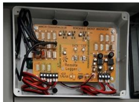
Figure 150: Remote Logger by www.re-innovation.co.uk based around LinkitOne PCB modified for use on this project (the LinkitOne PCB is fitted to the rear of the Remote Logger PCB).
