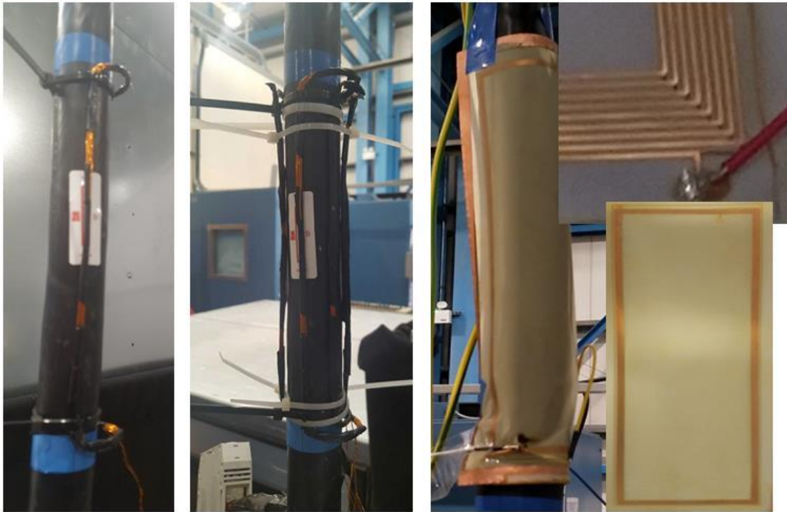
Figure 44: Photograph of one of the coils, a set of 3 coils and the PCB based coil
