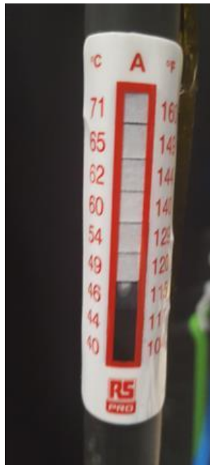
Figure 103: Thermal sticker change after hairdryer
