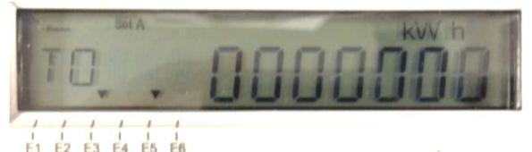
EW    Export register is stored on Set B registers. They can be obtained by holding down the SELECT button for 3 seconds this switches the meter between Set A registers and Set B registers.
