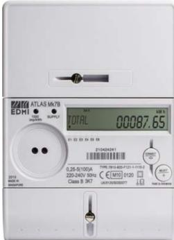
The EDM1 MK7B has built-in GSM communications which allows the register reads and half hourly consumption data to be remotely retrieved daily.
