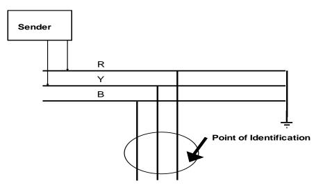
**Test 1** - With **Earths** removed from the leg to be identified ensure no signal is detected. Do not spike until the second test has been completed.
