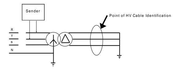
If it is not possible to make direct connection to the cable a signal may be injected through a distribution transformer.
