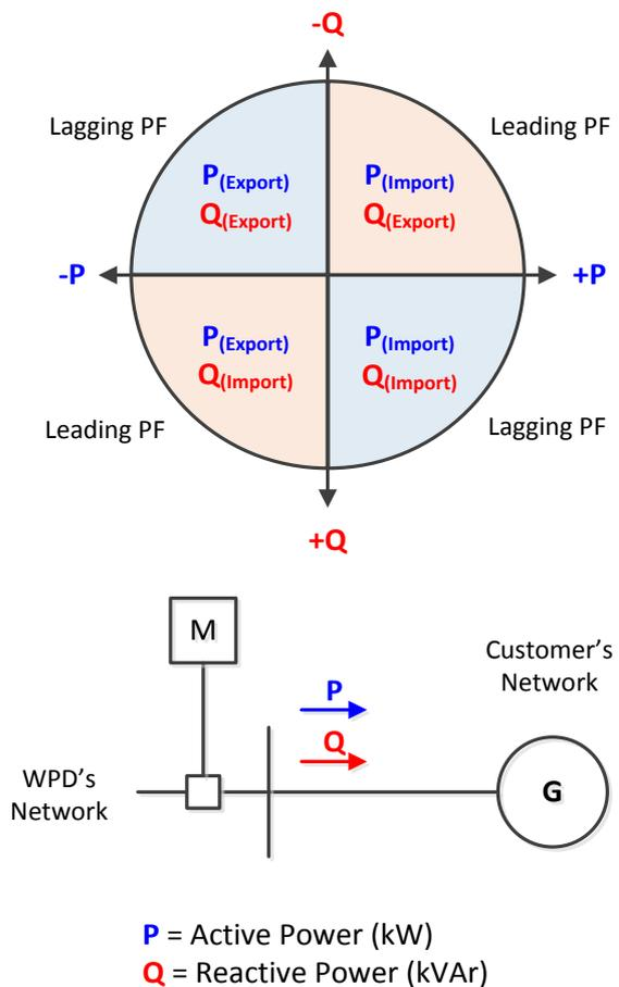
**Active Power (P)** is deemed to be positive (+ve) when it flows into the customer's installation from the distribution system.
