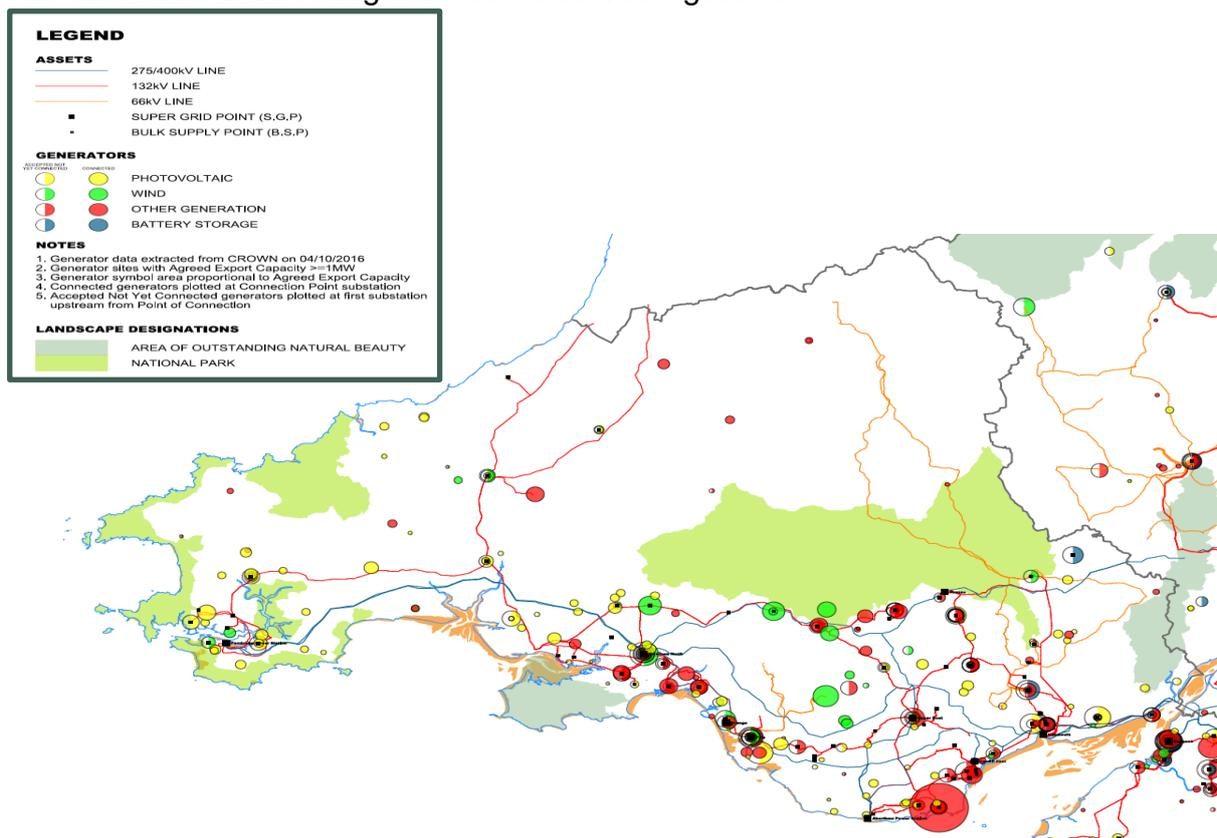
Figure 1: Network in South Wales showing 400kV, 132kV and 66kV networks together with generation in excess of 1MW capacity connected to the distribution network
