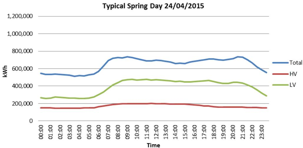
Figure 5: Typical Spring day energy usage profile
