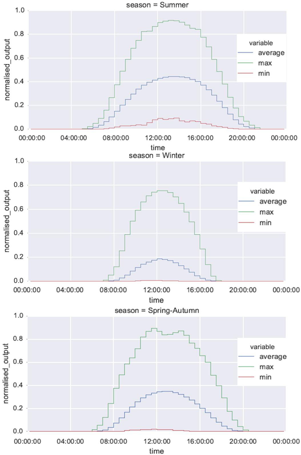
Figure 14: Normalised PV Profiles based on season
