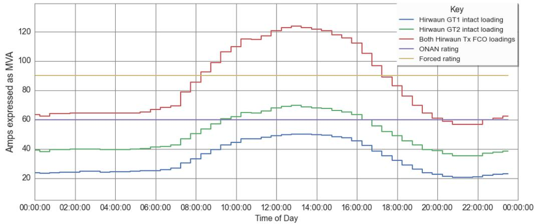
Figure 19: Hirwaun BSP GT1 and GT2 peak summer intact and FCO loadings under Gone Green 2025
