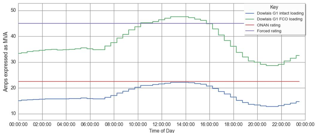
Figure 20: Dowlais Intact and FCO loading under Summer Consumer Power 2025
