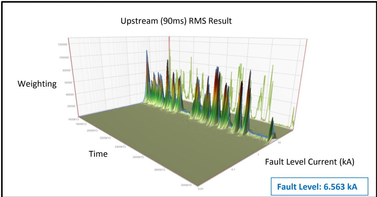
**Figure 2-4 - Prospective Break fault level results for Chester Street Primary substation**
