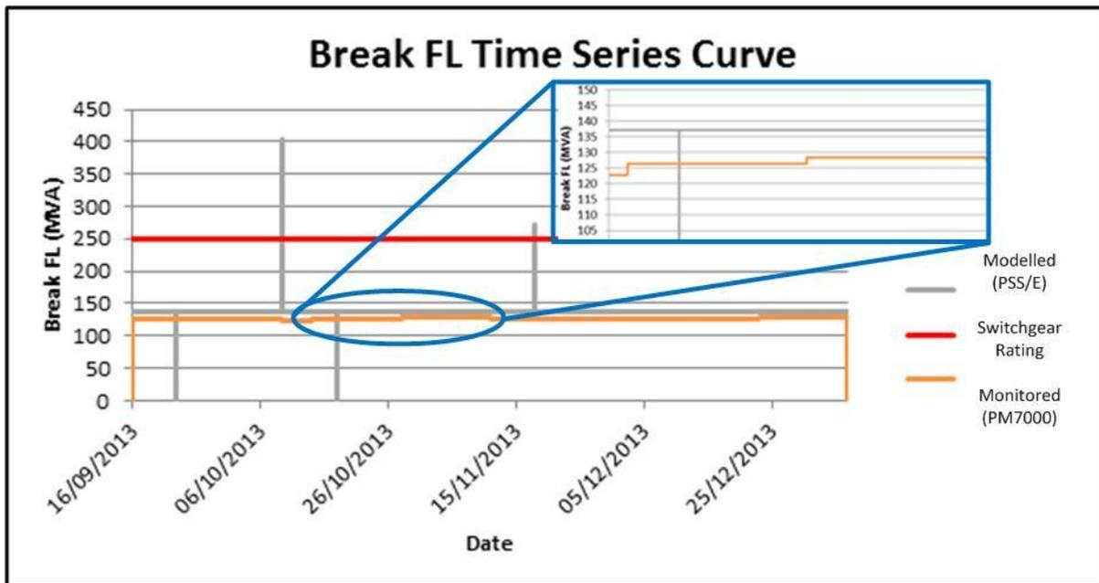
Figure 2-5 - Comparison of modelled and monitored fault level at GT2 in Chester Street Primary substation
