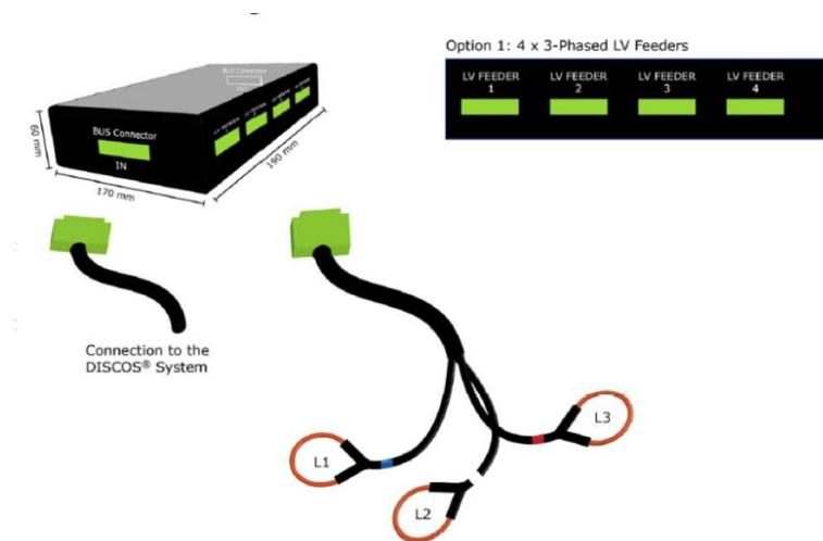
Figure 16: PowerSense LV satellite box and Rogowski coils
