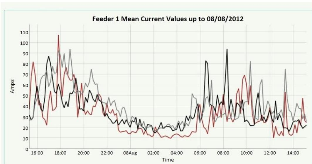
**Fig 12 – Typical Load Profile – Ritchie Gdns (WPD) -Gridkey**
