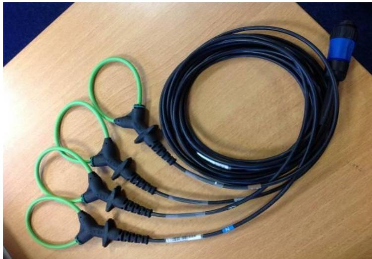
**Figure 1:** Rogowski coils with single screw on connector from GMC i-Prosyst.
