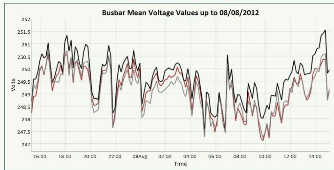
**Fig 13** – Typical voltage profile – Ritchie Gdns (WPD) –Gridkey
