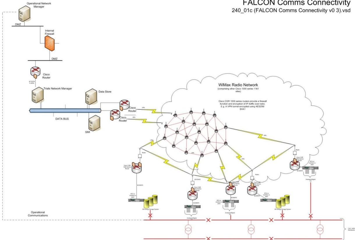
A pair of Cisco CGR1000 will be used to interface the network data to the Data Bus. This bus will connect the following:
