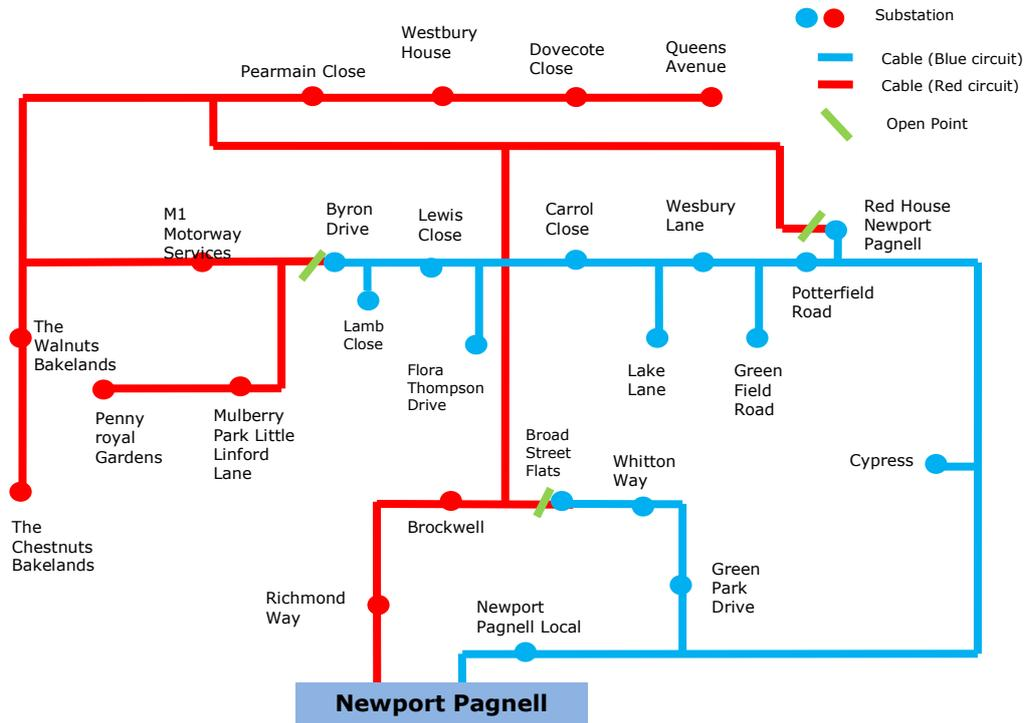
An example of how Automated Load Transfer can be configured on these feeders the following actions can be taken:
