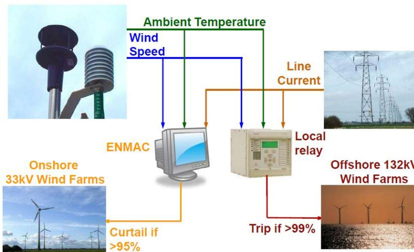
Dynamic Assets have previously being trialled and implemented on higher voltage circuits (33kV / 132kV) overhead line circuits to increase the output allowed from Wind Farms without having to replace or reinforce the connected circuits. Similar benefits could be obtained by expanding this technique to encompass points on the network where dynamic circuit ratings may be able to achieve extra utilisation within allowable rating.
