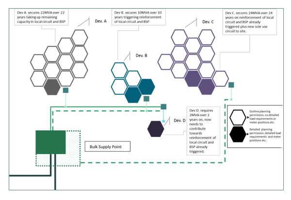
Dev. A is a multiphase development with a capacity requirement of 22MVA and an expected buildout timescale of 22 years for the 11 phases. This development utilises the available network capacity on the local circuit and the bulk supply point (BSP) and their accepted connection offer secures this capacity for the length of the entire development's construction.
