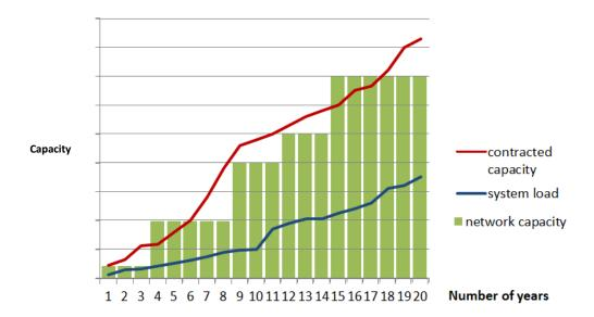
**Example scenario 1:** multiple large multi-phase developments securing large demand capacities over long timescales and triggering reinforcement
