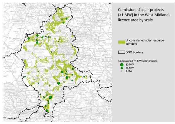
The occurrence of existing ground-mounted PV farms, shown as green circles, indicates a very strong correlation between the location of PV farms and the developable resource areas when a 2.5 km from 33 kV network proximity criteria is included.
